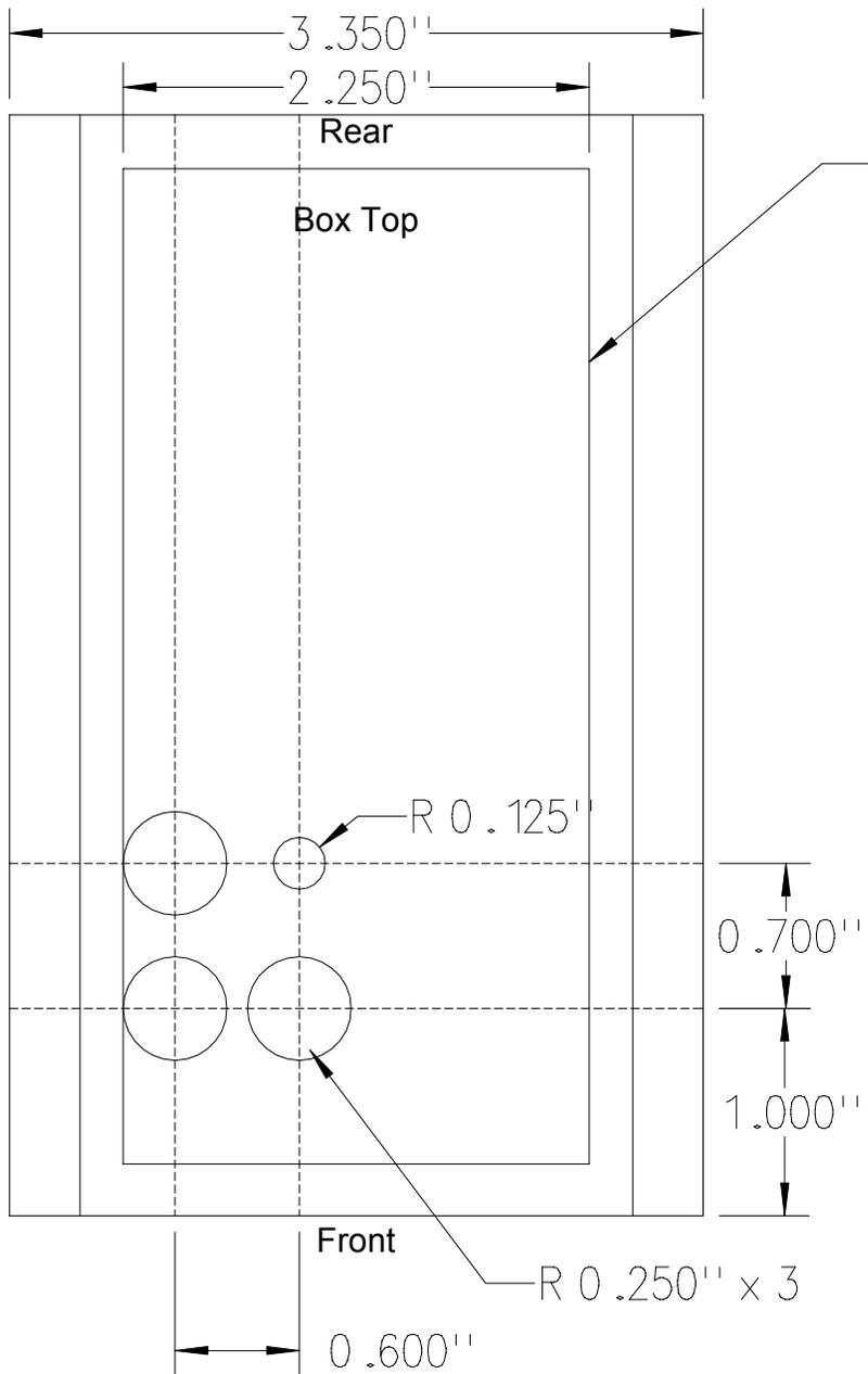
Cut out this section to locate holes on the enclosure.
