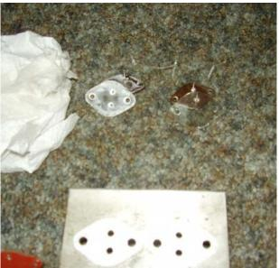
Once disassembled, it is time for some cleaning. When clean, the mica insulators will usually be clear (if you don't have the tinted version and aren't using thermal pads instead).
