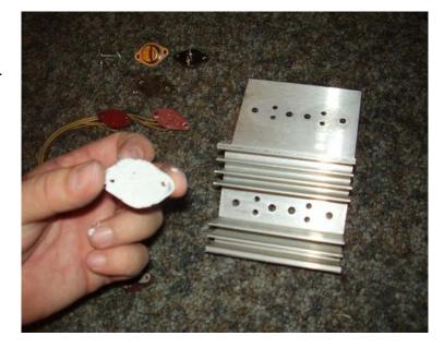
Also make note that the holes for the terminals on the transistors are off-center as are the holes in the insulators. They only go in one way. You CAN put them in backwards but it takes some effort as the sockets are pinned to fit the heat sink only one way as well and the terminal holes will not line up easily.
