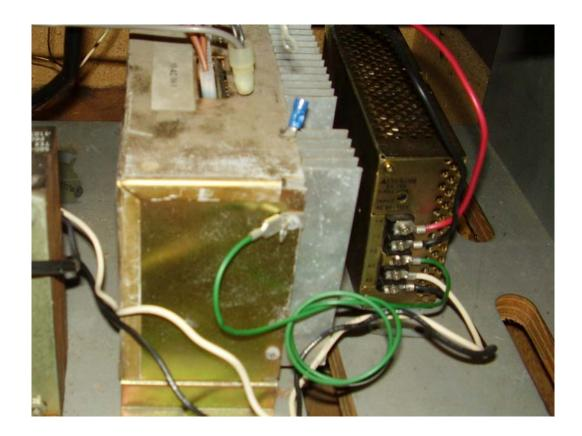
There was a nice tab already installed on the case of the linear power supply. My switcher is pictured on the right. The black and white wires are my AC supply that I piggybacked onto the transformer earlier. The green is a ground. The red and black wires will be going to my adaptor.
