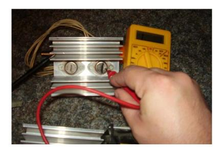
And I am seeing no continuity on my transistors. This means my mica insulators are doing their jobs and most likely none of the transistors are in backwards. Now it is time to put this back together.
