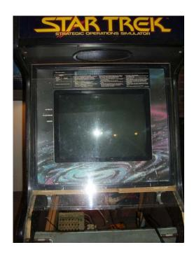
Now remove the black Plastic Bezel by simply sliding it out. It is a snug fit but should not be anchored by anything. Once removed, you will be greeted by the monitor mounting bolts.
