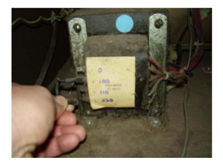
Plug the game back in (leaving the monitor power unplugged as well as the power supply) and measure the voltage again. This should put you right back in the ballpark of what voltage your monitor was designed to use (45VAC).
