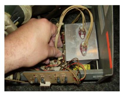
The harnesses are keyed and only go on the connector one way. It does not matter which harness goes on which paddle board\* or header. Do not abuse the paddle boards at this point as they are not mounted solidly.
