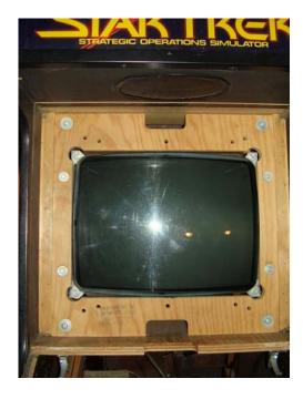
The power wire has clips that need to be squeezed together. The input wires on the upper right are just a slip fit usually but that header can be tight. Once the wires are disconnected, grab the hand holds in the plywood mount and slide the monitor out the front of your cabinet.
