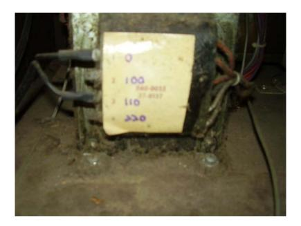
Just wiggle and pull on the connector at tap 1 and move it to tap 2. Then do the same with the connector on tap 3 and move it to tap 4.
