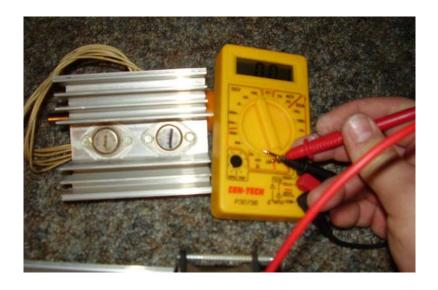
Now that I know my meter is working, I just need to verify the transistors are not shorted to the heat sinks.
