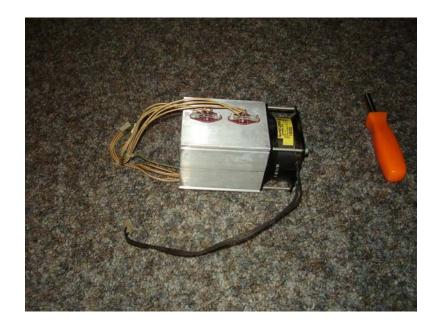
I have put it back together after wiping up the excess heat sink compound that I slopped around as it will attract dust. I have also made sure to orient the harnesses in the most advantageous positions for reassembly.
