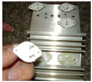
Put the transistor in place and slip on the socket from the back. On this particular monitor\*, all the transistors (2n6529) are identical and interchangeable.
