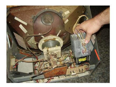
There is a small "stop" punched into the monitor frame that helps you align the unit. It is almost dead center in the picture below.
