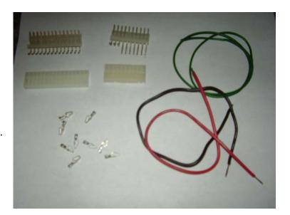
I simply use pliers to straighten out the first 7 pins of the angled header. This gives me some nice long connectors to work with.
