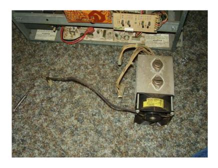
Now pull the fan by removing the four end screws.
