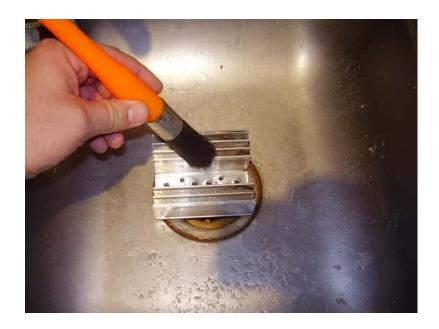
Once it is all clean we are ready to reassemble. Inspect the sockets for loose wires and the transistors legs for corrosion. Anything that will prevent a clean, tight, connection will cause problems down the road to include periodic screen collapse.
