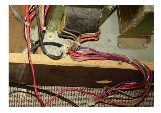
Per the schematics, the monitor is designed to take 45 VAC input from the two red wires with the black wire being a ground (common). Set your meter to measure AC Voltage. Put the black lead on the black wire and the red lead on the red wire. Make sure that you do not have your leads on a conductive surface (i.e. metal, water, etc.). Now power on the game and observe the voltage.
