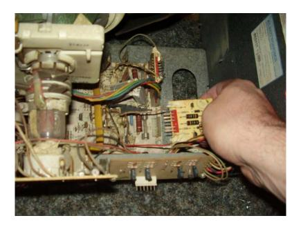
If you are having collapse problems on your monitor, you may have cracks in the solder on the header pins on the paddle board (in the picture above they are red). Another possibility is that you may have bad solder joints on the paddle board header pins, located on the main board.
