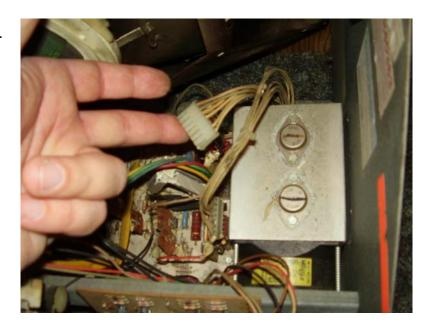
In order to pull these two harnesses, it may be necessary to hold down the paddle boards\* or they will come loose. Not a big deal if that happens but it should be noted that even though the paddle boards remove easily from their headers on the main board, they have jumpers that are soldered in and cannot be removed completely...
