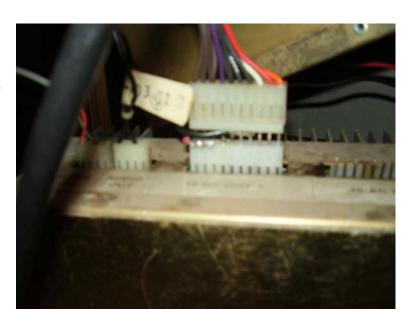
Make sure that everything is as it should be (no shorted wires, everything secure), double check my connections, and power it up! You should immediately measure and adjust (if necessary) the +5 at this point. The load of the game board will need to be compensated for.
