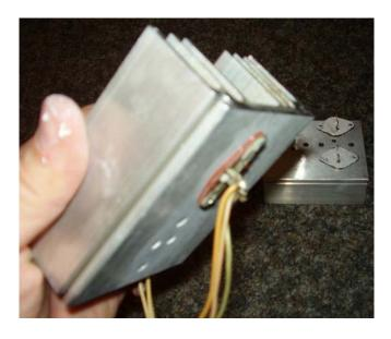
If your socket is sitting **FLAT** against the heat sink then you have things lined up right. Just screw the transistor down. Don't apply too much force.
