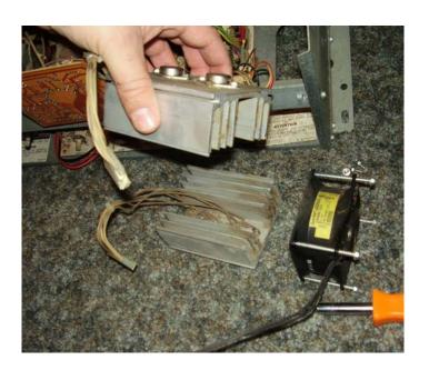
Remove the transistors\* by removing the two screws holding each one in and pulling firmly on the transistor body.
