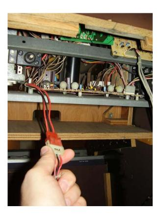
...and the AC input connector from the power supply.
