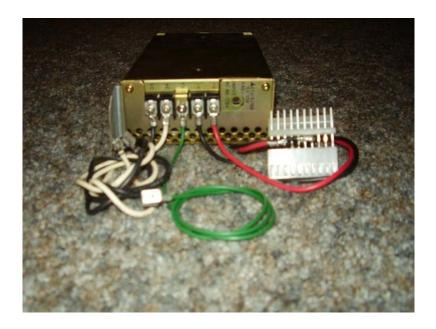
On my Star Trek, the three pins on the left were the +5. Notice those pins do not go all the way through to the bottom connector. The next pin was the -5 voltage so I skipped it. The next three pins are my grounds. I stripped about half an inch of each of my DC supply wires and soldered my +5 (red wire) across the isolated +5 pins and my ground (black wire) across the common ground pins. I was very careful to ensure the -5 pin did not get shorted to either my ground or +5 line when soldering.
