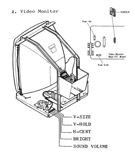
Do not touch the inside of the video monitor in which many parts are supplied with high tension.
