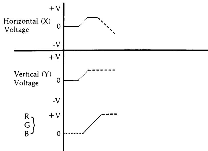
In our example, we made a very short line, considering we could have drawn one clear across the screen. In order to draw longer lines, in any direction, we simply increase the positive or negative voltage on the inputs. Remember - the higher the voltage, the more the deflection, the longer the line.
