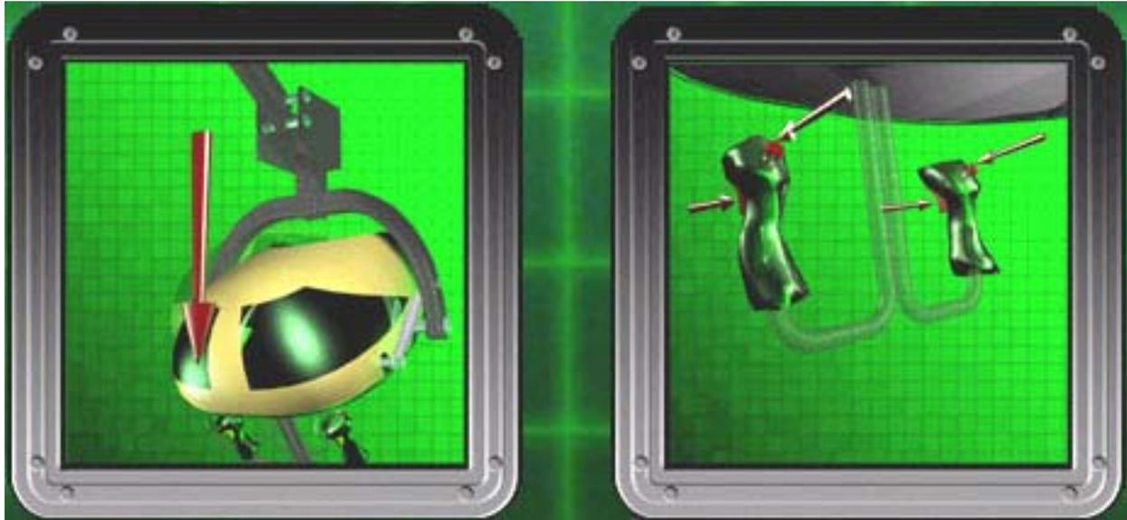
The Player Control Test will validate that the controls are setup correctly and working on the cabinet. When you press a button a red arrow will appear on the test screen when it is operating correctly as shown in the picture above. When you move the Headset in any direction a red arrow will appear in the direction that the Headset is moving when it is operating correctly. When you are finished testing the player controls press the Operator Button to exit back to the main operators menu.
