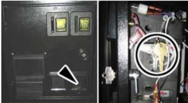
Remove the back door from the cabinet and inspect the computer system. Verify that all cables and major assemblies are securely connected to the computer and mounted to the side of the cabinet.
