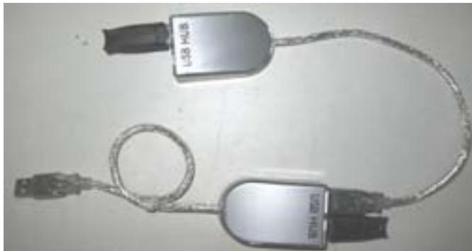
In the event that 2 USB HUB's are needed to create enough USB ports for all the game dongles you can daisy chain the USB HUBs together as shown above. Do not plug the USB cable coming from the HAPP GCI Controller card in the USB HUB's as this will cause the card to not work.
