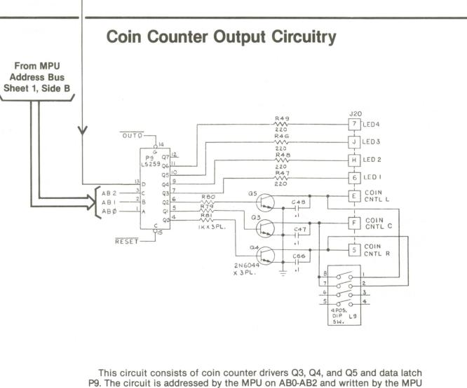
This circuit consists of coin counter drivers Q3, Q4, and Q5 and data latch P9. The circuit is addressed by the MPU on AB0-AB2 and written by the MPU on data line DB7. When the input to a driver is clocked high, its collector goes low grounding the return of the coin counter in the coin door.
