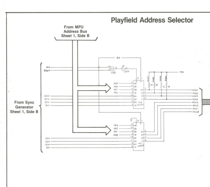
The Playfield Address Selector controls the access to the playfield memory. It allows either the game MPU or the sync generator to scan the playfield memory. The Playfield Address Selector consists of multiplexers M3, and M5 and gates J6 and N9.
