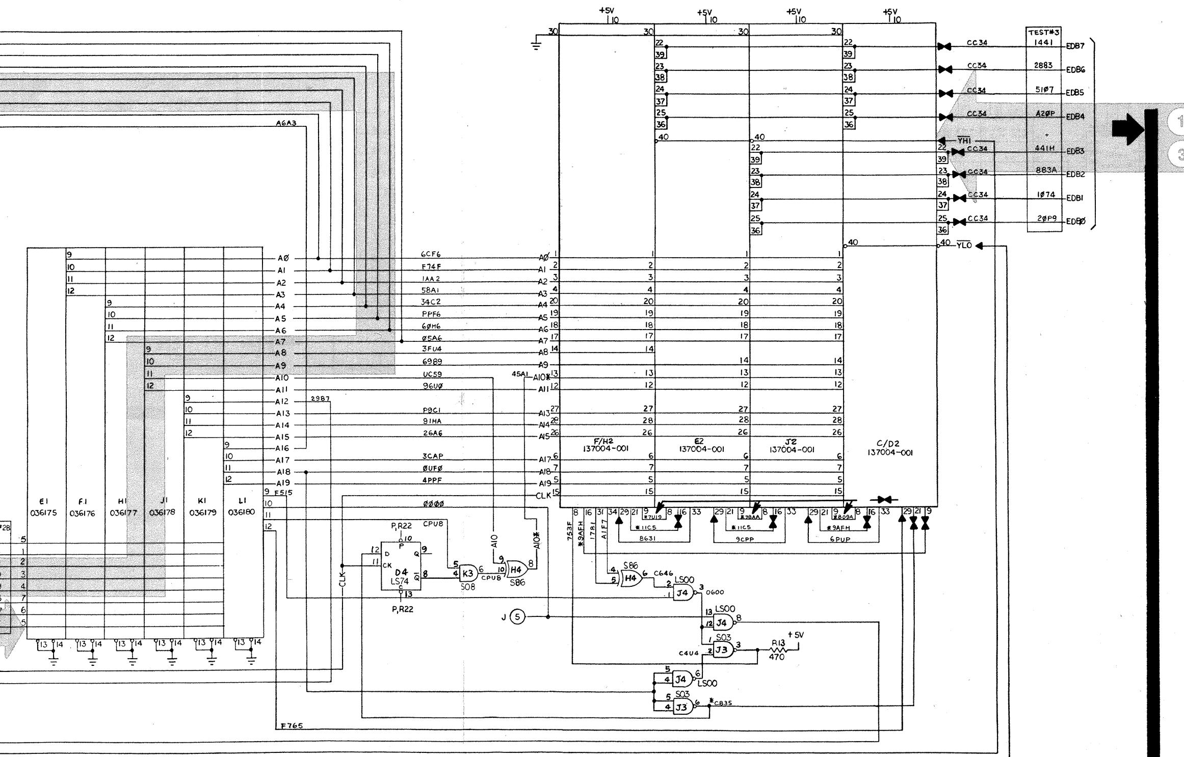
\* All signatures with an asterisk are taken with a 1K ohm pull-up resistor attached between the signature analyzer data probe and +5 VDC.
