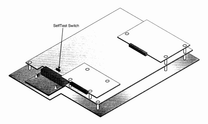
Figure 2-1 Location of Self-Test Switch
