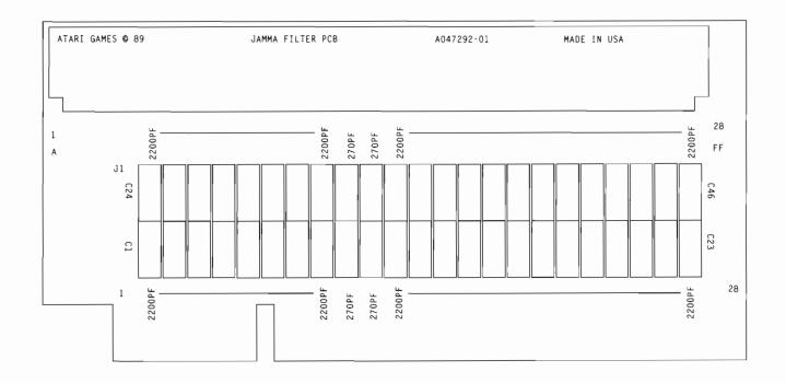
Figure 4-5 JAMMA Filter PCB Assembly
