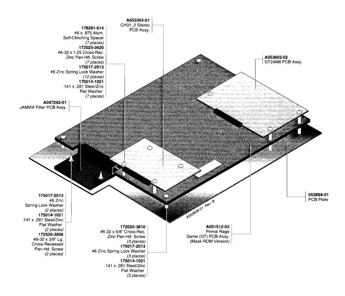
Figure 4-2 Board Stack Assembly
