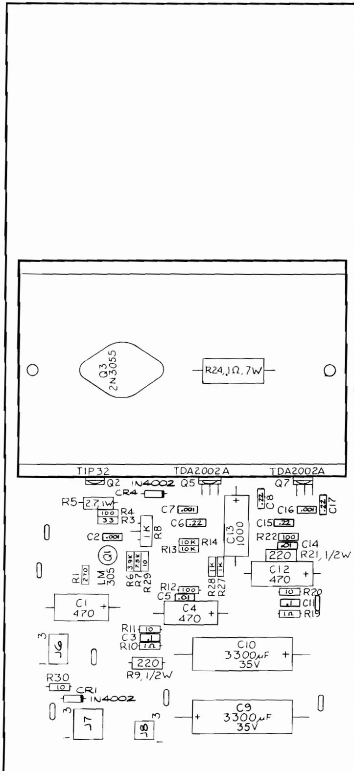
Figure 3-18 Regulator/Audio II PCB Assembly
