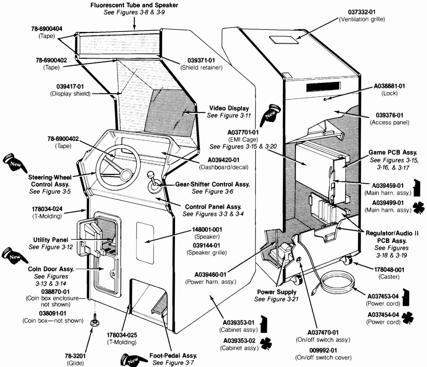
**Figure 3-1 Cabinet-Mounted Assemblies**
