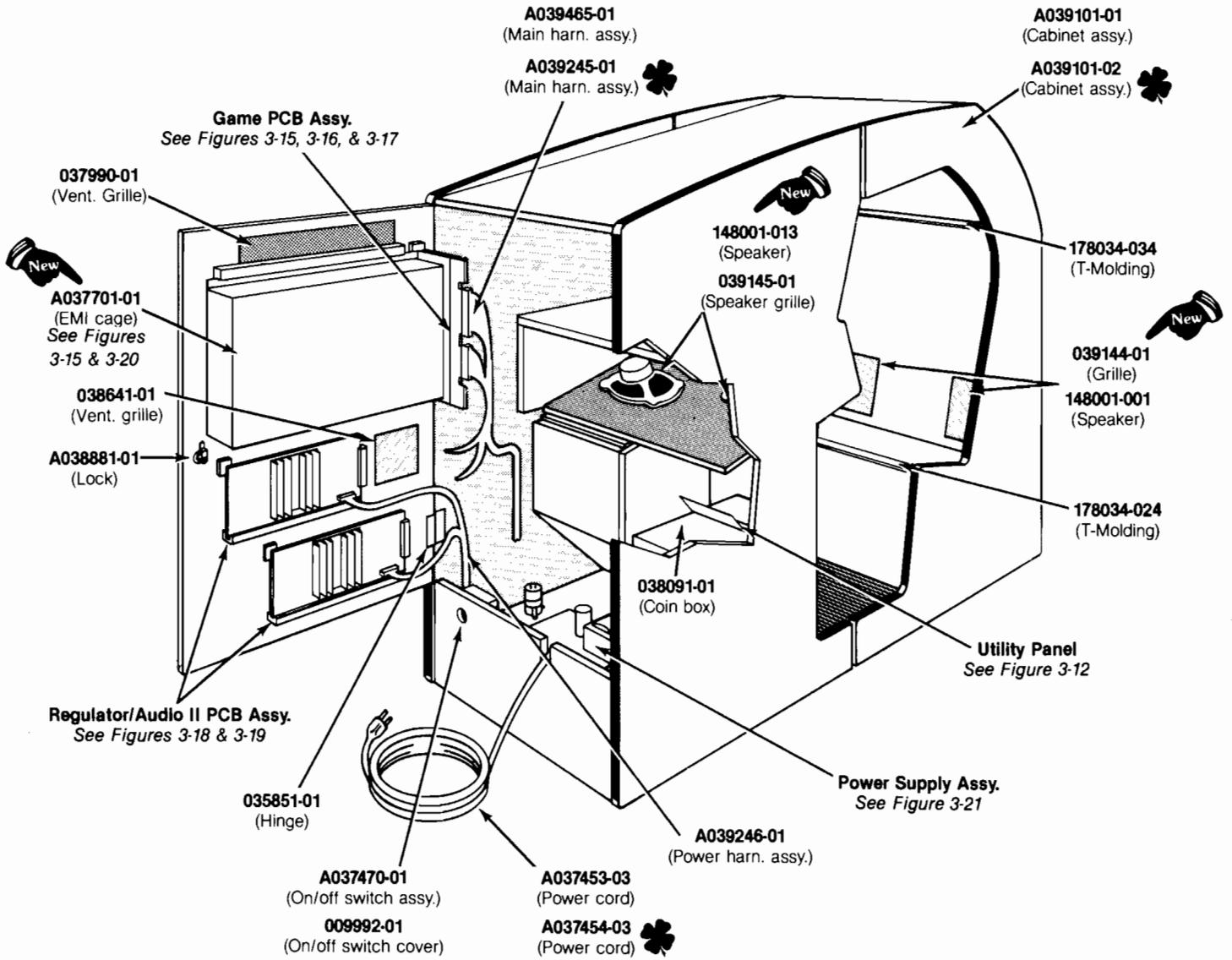
**Figure 3-2 Cabinet-Mounted Assemblies**
