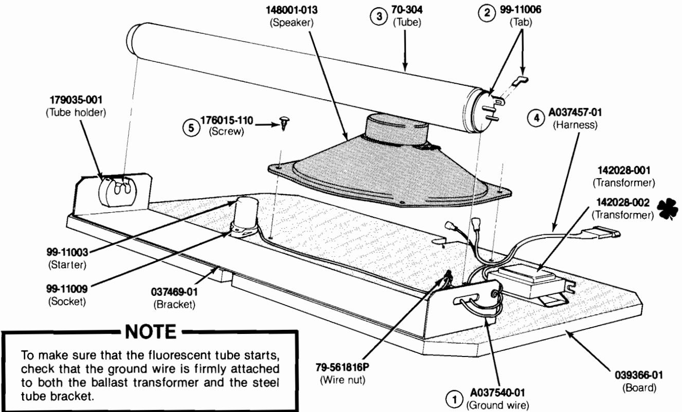
**Figure 3-9 Fluorescent Tube and Speaker Board Assembly**
