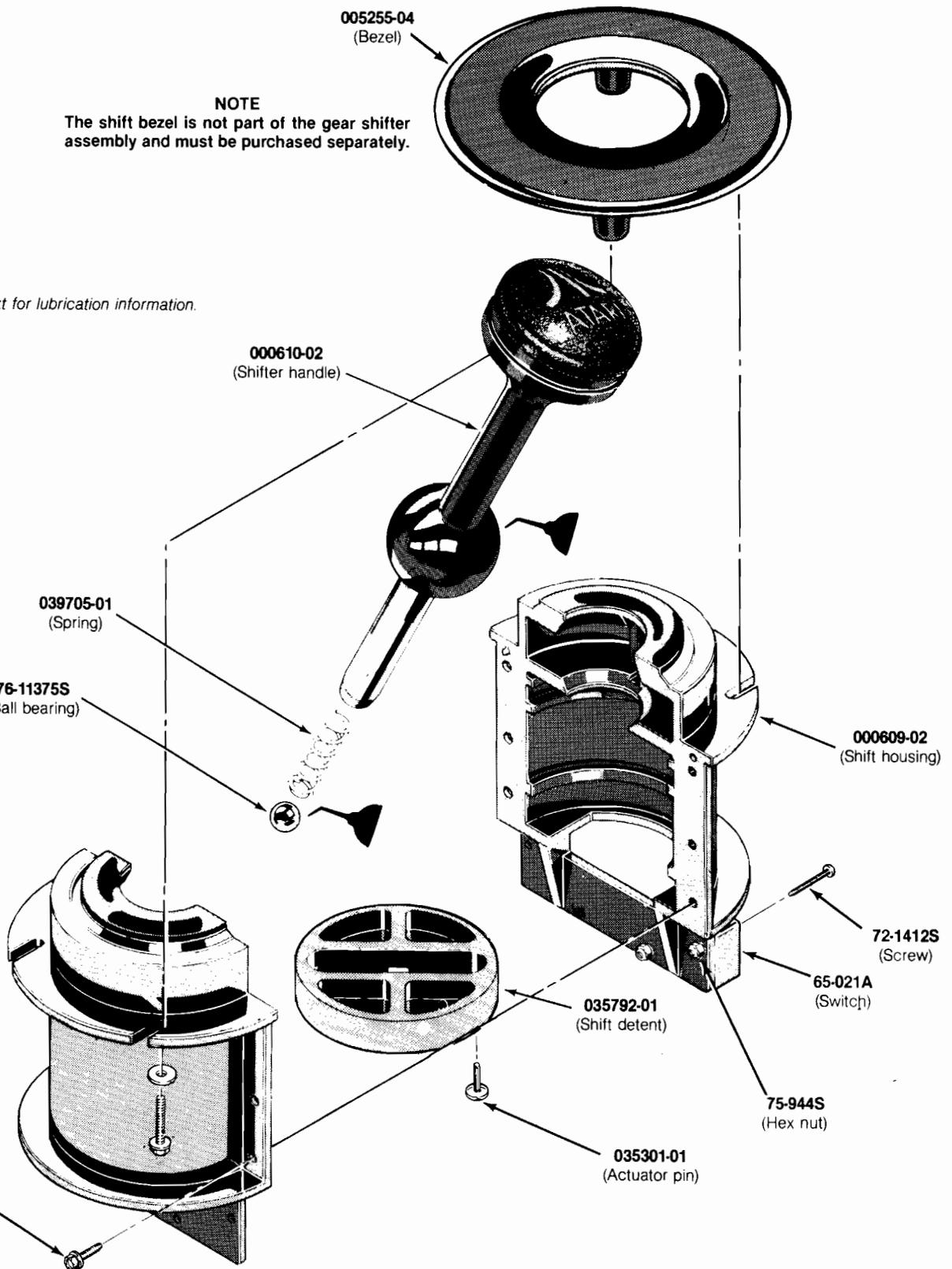
**Figure 3-6 Gear-Shifter Control Assembly
