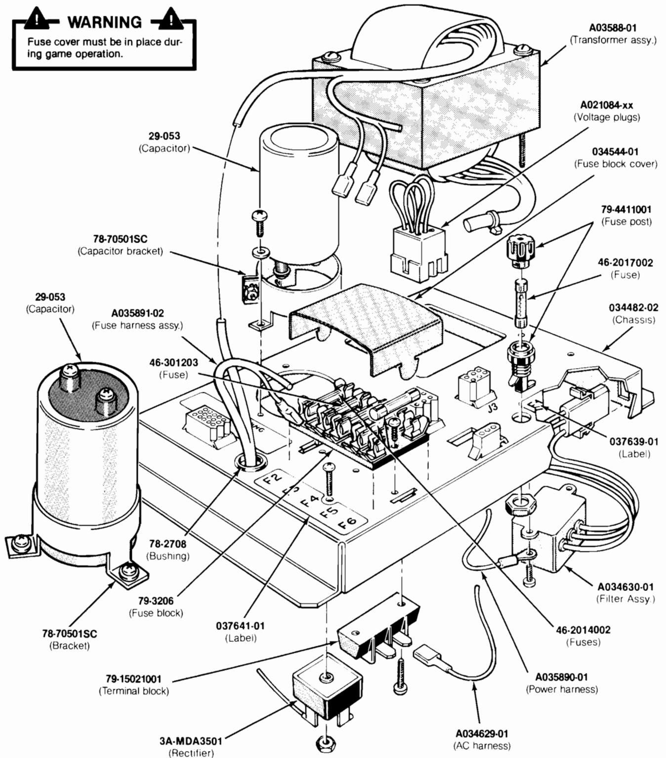
**Figure 3-21 Power Supply Assembly
