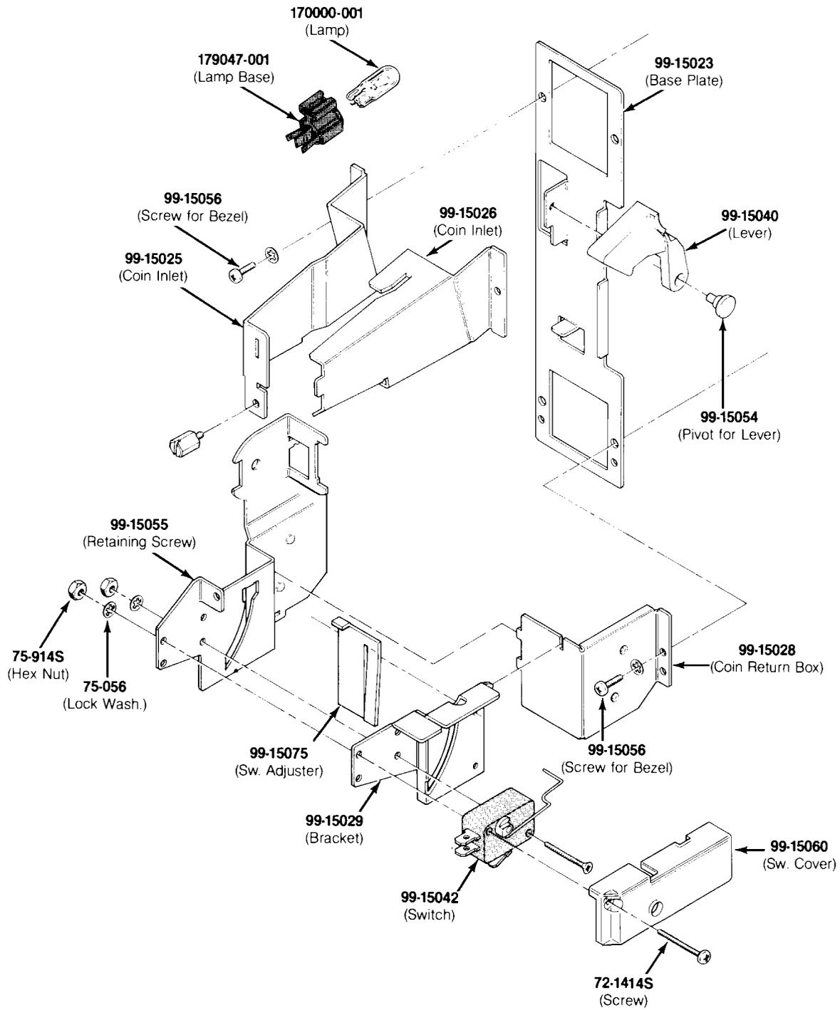
**Figure 3-13 Vertically Mounted Coin Door
