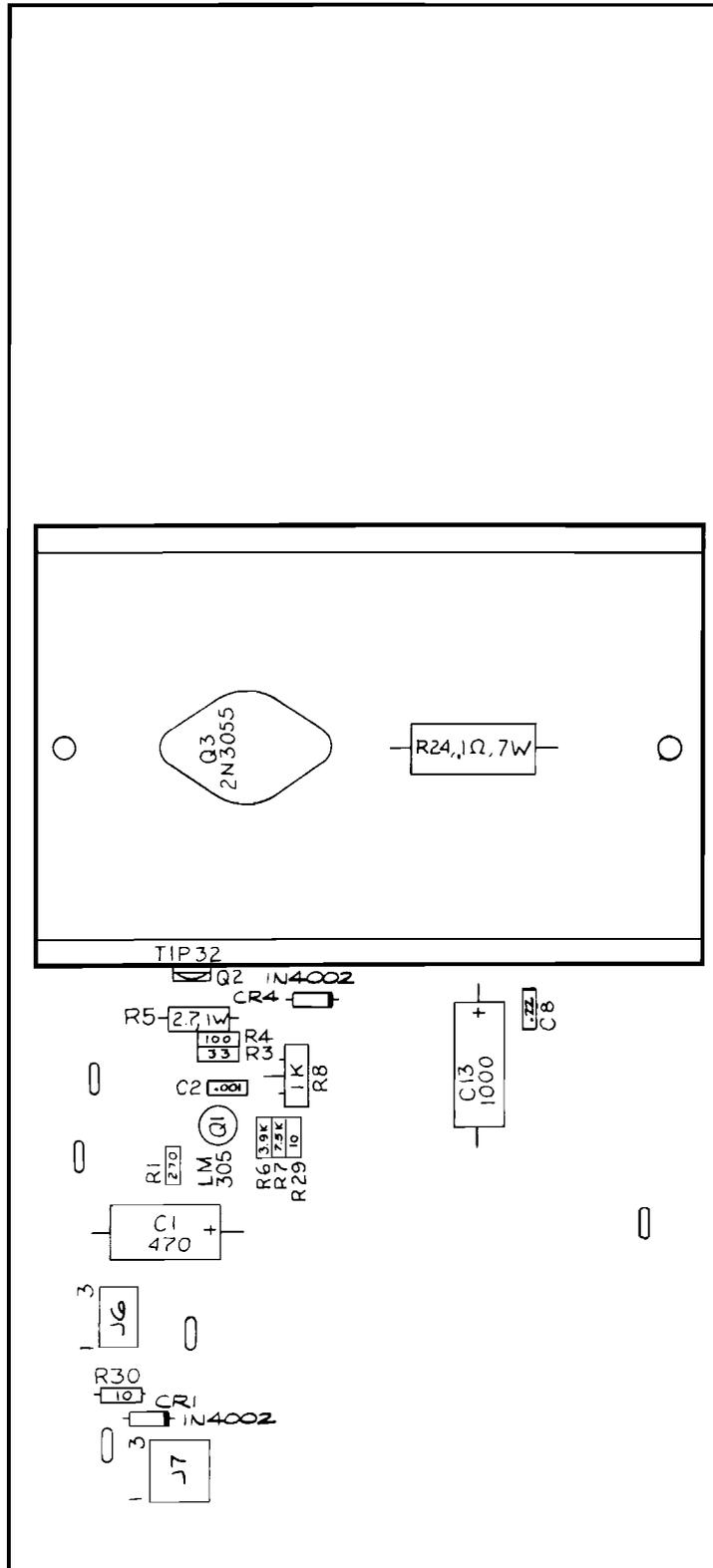
**Figure 3-19 Regulator/Audio II PCB Assembly**
