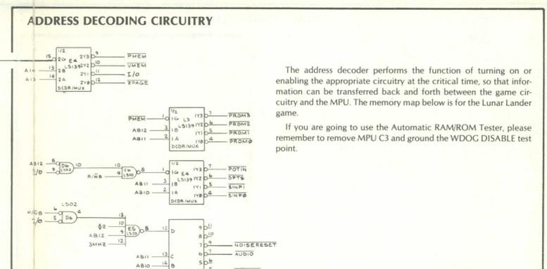
The address decoder performs the function of turning on or enabling the appropriate circuitry at the critical time, so that information can be transferred back and forth between the game circuitry and the MPU. The memory map below is for the Lunar Lander game.
