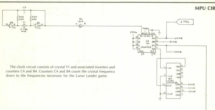
The clock circuit consists of crystal Y1 and associated inverters and counters C4 and B4. Counters C4 and B4 count the crystal frequency down to the frequencies necessary for the Lunar Lander game.
