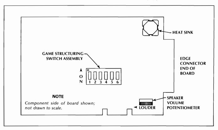
Figure 4-1 Approxiate Locations of Game Structuring Switches and Speaker Volume Adjustment
