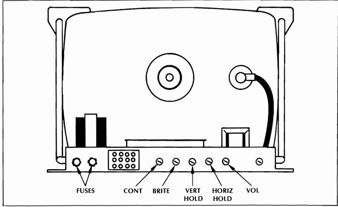
Figure 5-1 Location of Adjustments on TV Chassis
