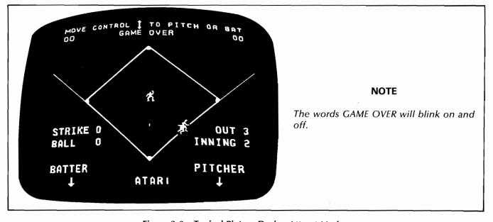
Figure 3-3 Typical Picture During Attract Mode
