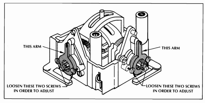
Figure 5-4 Detail View of Joystick Assembly
