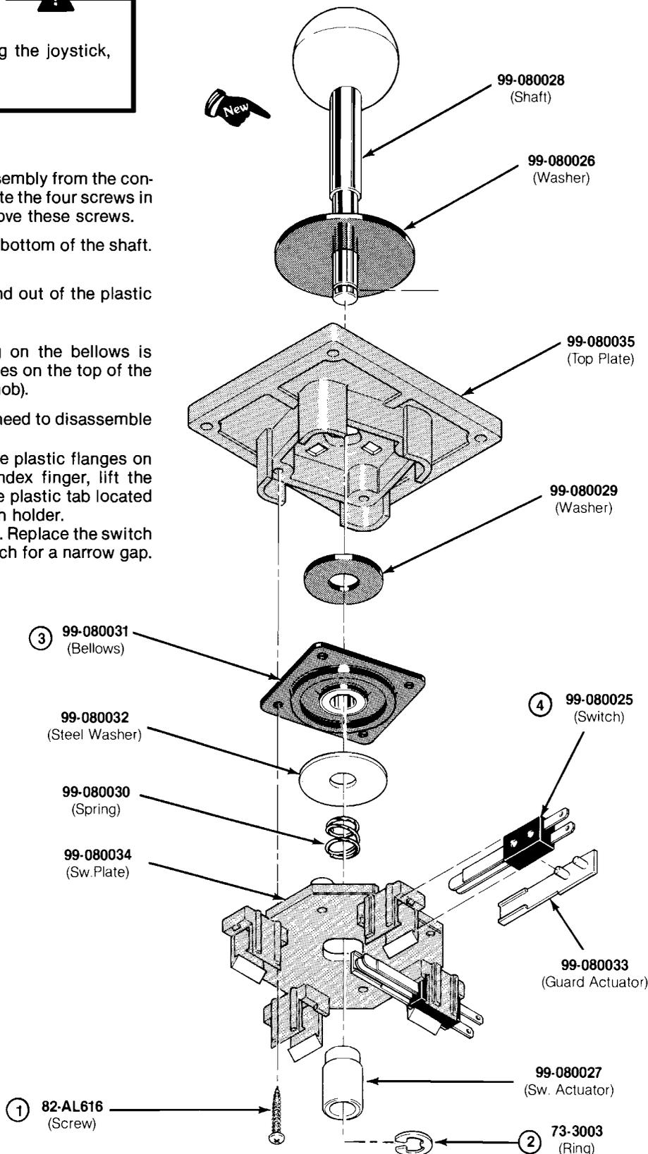
**Figure 3-4 Joystick Assembly**
