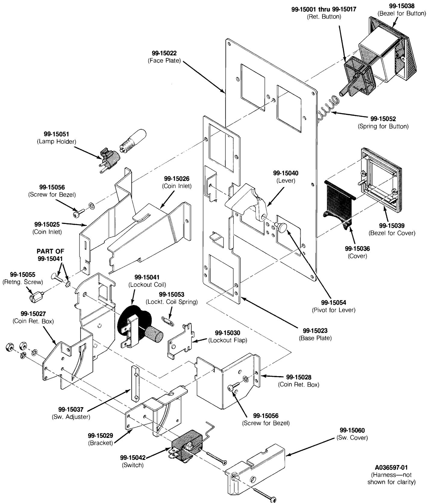
**Figure 3-8 Double Coin Acceptor/Mount Assembly
