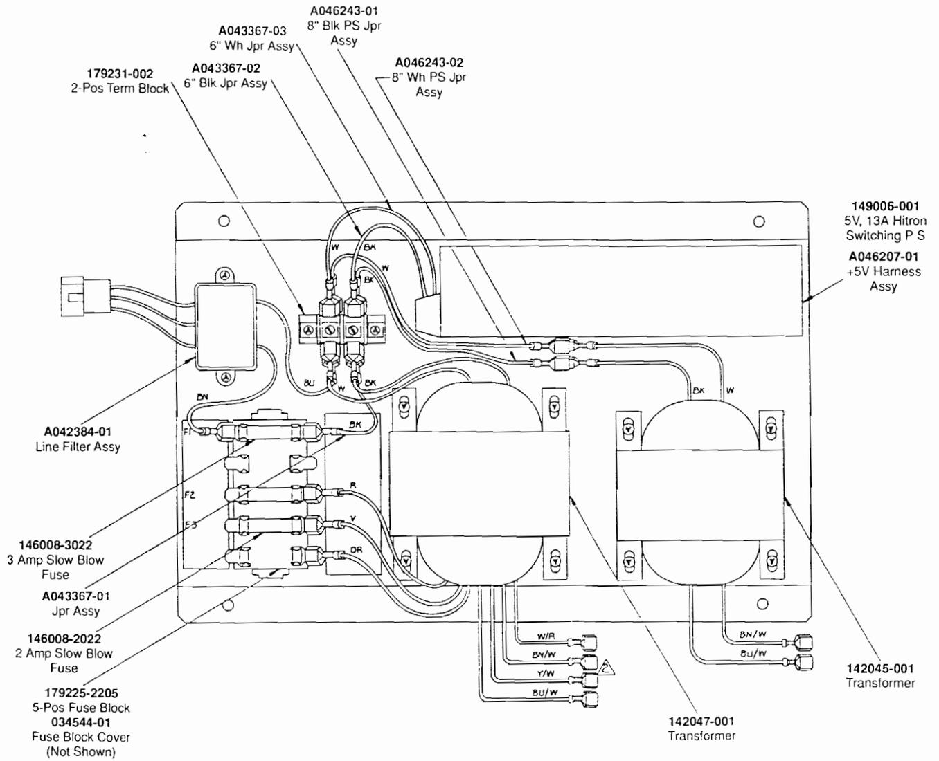
**Figure 4-4 Power Supply Assembly
