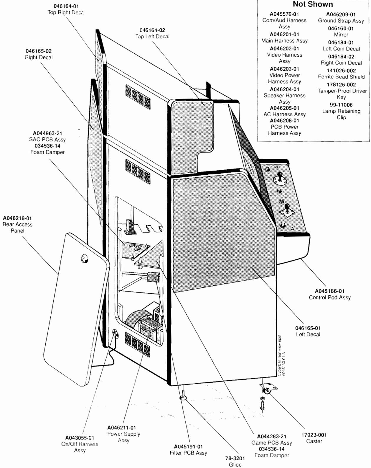
**Figure 4-1 Cabinet-Mounted Assemblies, Rear View
