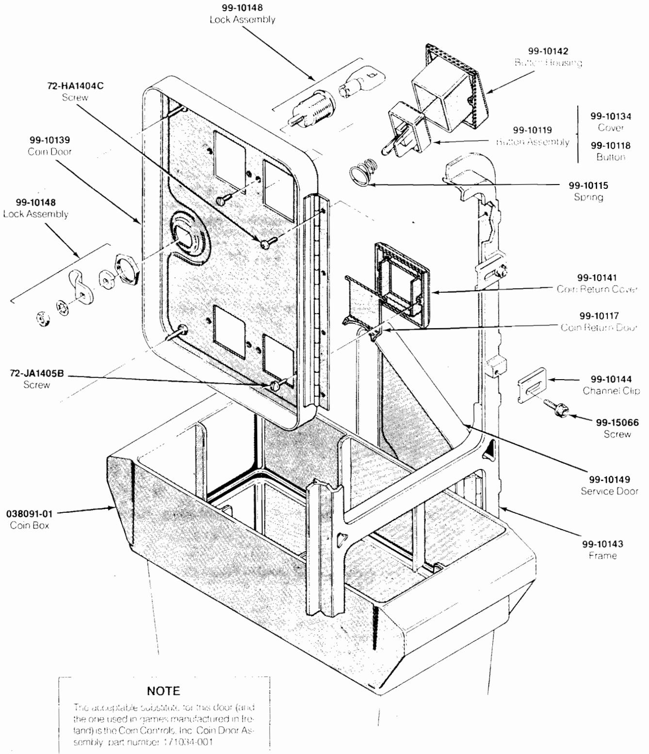
Figure 4-5 Coin Acceptors, Inc. Coin Door Assembly, Continued
