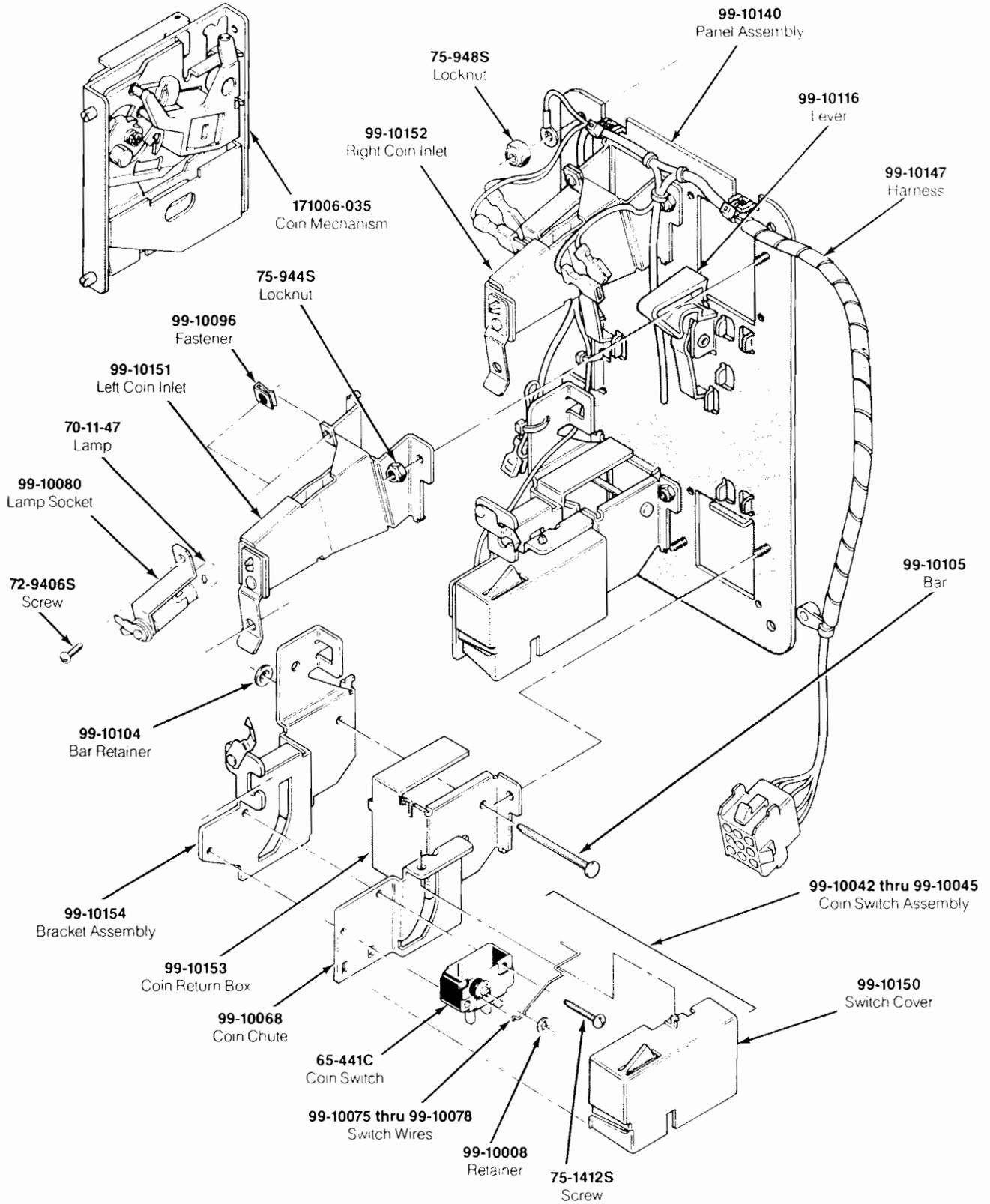
**Figure 4-5 Coin Acceptors, Inc. Coin Door Assembly
