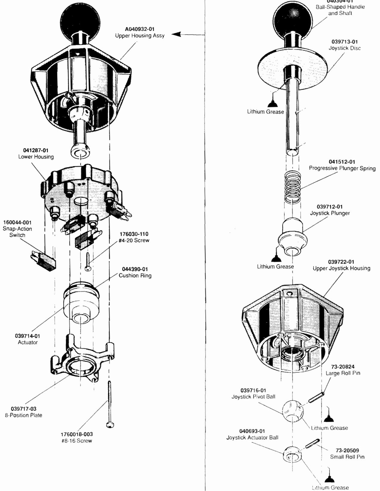
**Figure 4-3 Joystick Assembly**
