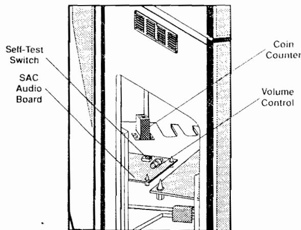
**Figure 1-1 Control and Switch Locations**
