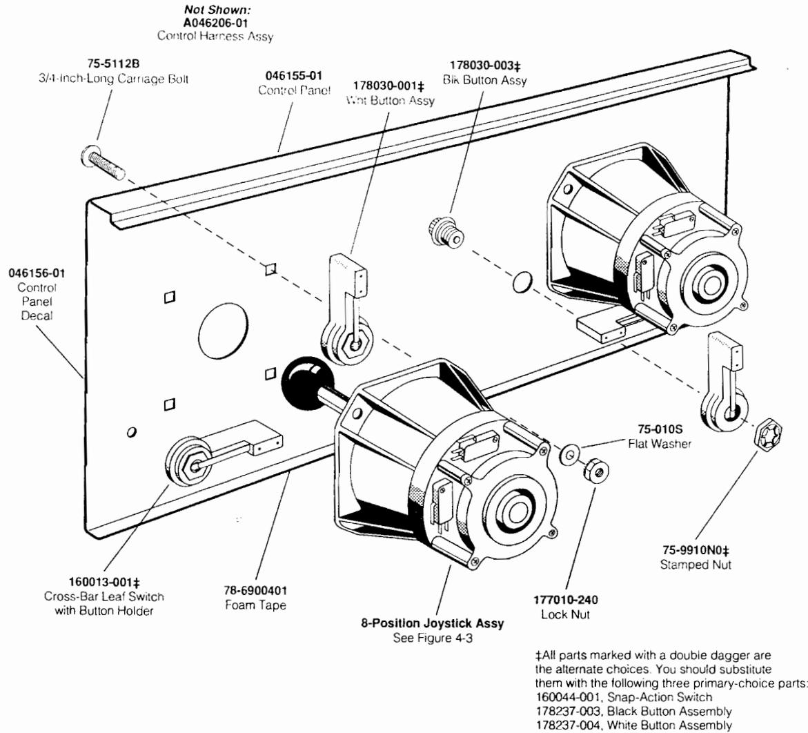
**Figure 4-2 Control Panel Assembly
