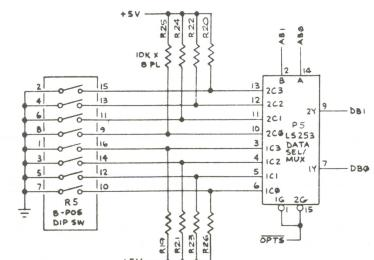
The game option switches are read by the MPU when OPTS (option switch enable) is low. Switch toggles to be read are selected by AB0 and AB1 from the MPU. Switch toggles 1, 3, 5 and 7 are read on data line DB0 and toggles 2, 4, 6 and 8 are read on DB1. Toggle inputs are "on" when pulled to ground.
