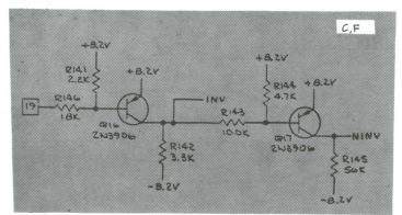
The video inverter circuitry is only used in a cocktail game. In an upright game, pin 19 is unconnected and therefore floats. When pin 19 floats, transistor Q16 is turned off and transistor Q17 is turned on. Therefore, INV is -8.2 VDC and NONINV is about +8.2 VDC. The result is a non-inverted X-axis and Y-axis output.
