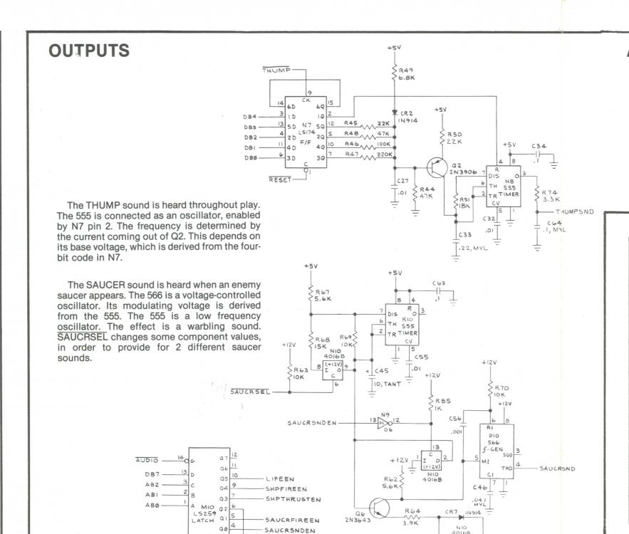
M10 latches control signals to enable different sounds.
