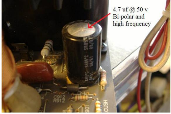
Capacitors C412, C817, C818, and C908 can only be accessed for replacement by temporarily removing the Resolution Selector Board.
