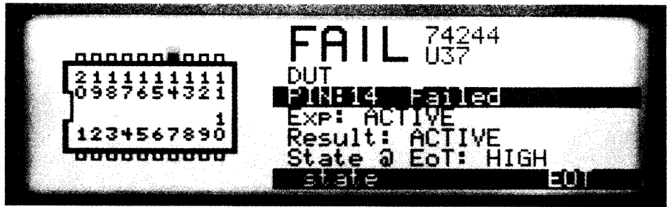
Upon detection of a mismatch between the outputs of the Reference Device and the corresponding output pins of the device under test, the tester ends the comparison and displays the failing output pin(s).
