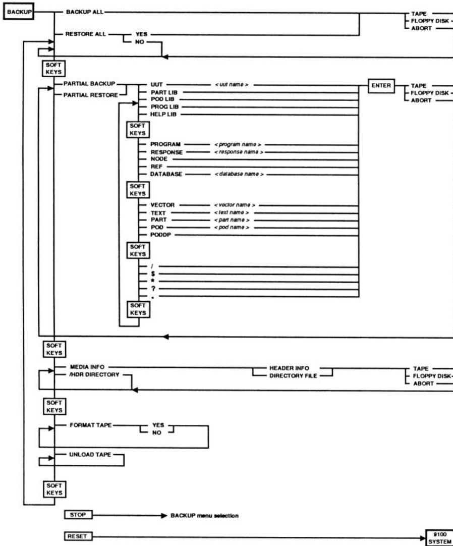
Figure 1. Key Syntax Diagram
