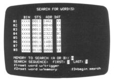
**SEARCH-FOR WORDS** — This screen allows the user to specify a sequence of up to 8 words to search for in either A or B Memory. The f1 and f2 keys are used to facilitate loading of a complex word into the search list from a trigger word or from memory.
