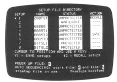
**SETUP DIRECTORY** — Up to eight ML4100 setup files can be saved, including timing line probe designations and their labels. (A setup file contains all setup parameters selected by the user.) Each file can be assigned a 6-character name and a status of "Protected" or "Unprotected". The "Protected" status, designated by a 2-digit security code, prevents accidental erasure or loss of stored data.
