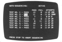
**AUTO SEQUENCING** — This screen summarizes automatic tests run to date, and always indicates which one is in progress. It also indicates the order in which the tests are being performed. This capability allows automatic powerup and operation of the ML4100 for sophisticated tests without expert knowledge of logic analyzer operation. Even more significantly, the ML4100 can now run repetitive, unattended tests for
