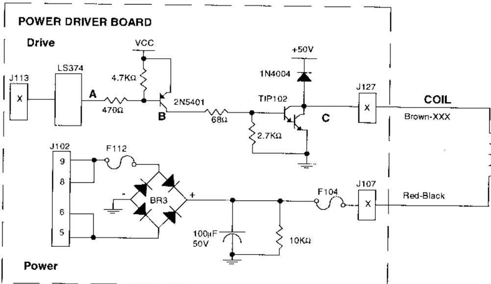
The processor toggles the output of the 74LS374. When point "A" is low, point "B" the collector of the 2N5401 transistor, is high. A high at point "B" turns on the TIP102 transistor and causes point "C" to drop low. When point "C" is low the coil is grounded through the transistor and turns on. The coil shuts off when point "A" toggles high.
