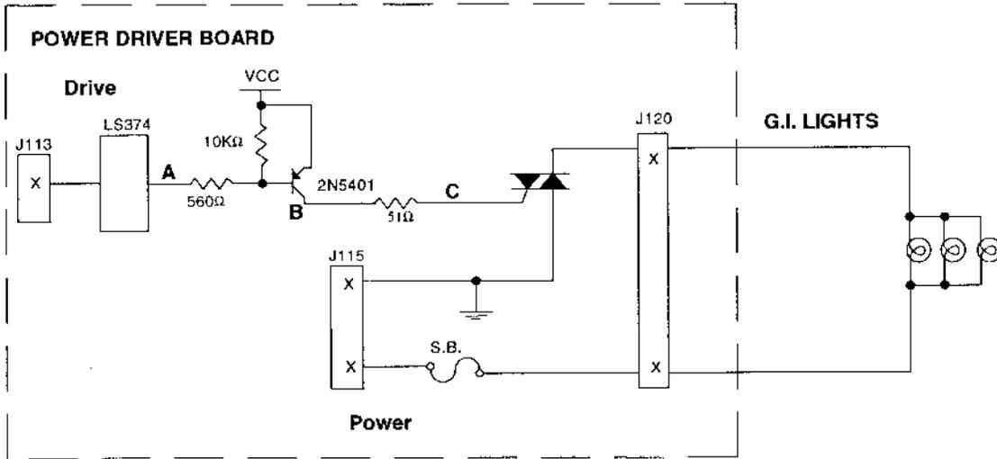
When point "A" toggles low, points "B" and "C" are high. This turns on the triac and the desired general illumination string lights.
