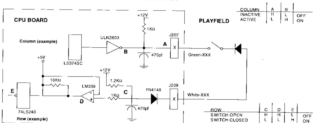
The microprocessor is constantly strobing the column side of the switch. When point "A" on the column circuit toggles low, the column side is active.
