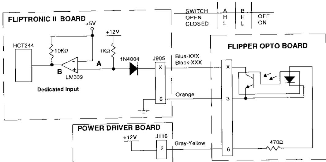
The flipper switch circuits operate similar to the dedicated switch circuit. The circuits are active low and tied to ground through the switch circuit.
