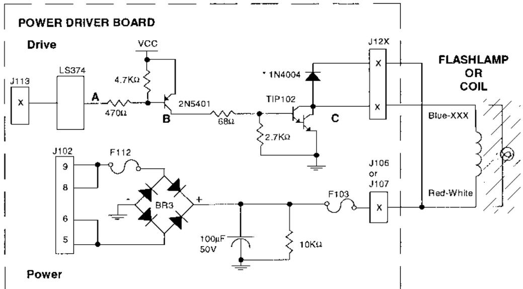
The processor toggles the output of the 74LS374. When point "A" is low, point "B" the collector of the 2N5401 transistor, is high. A high at point "B" causes a low at point "C". When point "C" is low the coil/flashlamp is grounded through the transistor and turns on. When point "A" toggles high the coil/flashlamp turns off.
