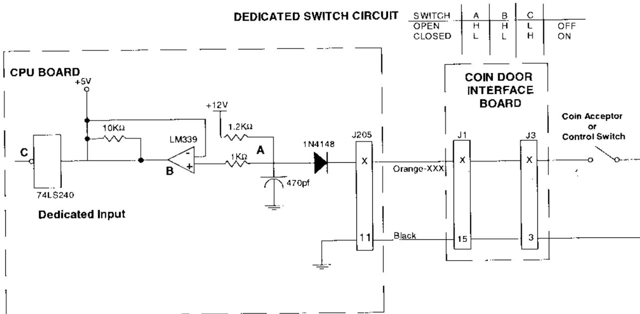
The dedicated switches operate similar to switches in the matrix, except that instead of a column circuit there is a direct tie to ground. Therefore, the column side is constantly active (low).
