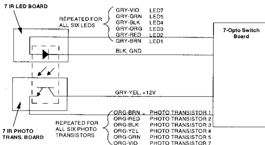
IN THE OUTHOLE TROUGH CIRCUIT, THE BALL ROLLS BETWEEN THE TWO BOARDS AND BREAKS THE BEAM, CAUSING THE SWITCH TO READ AS MADE.
