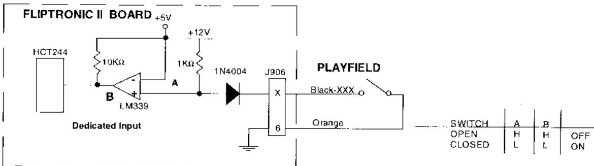
The flipper E.O.S. circuits operate similar to the dedicated switch circuit. The circuits are active low and tied to ground through the switch.
