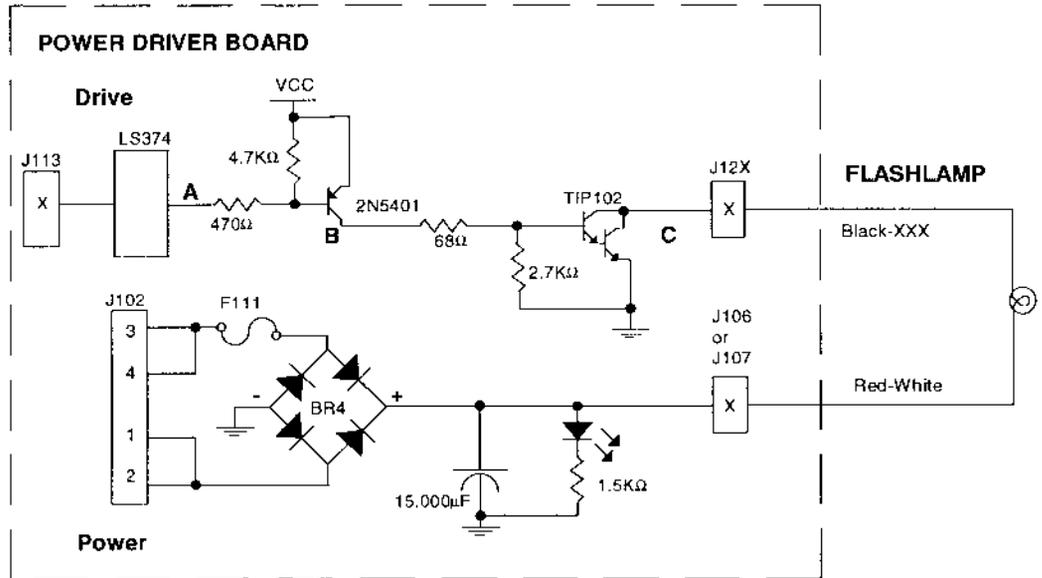
The processor toggles the output of the 74LS374. When point "A" is low, point "B" the collector of the 2N5401 transistor, is high. Once point "B" is high, point "C" the collector of the TIP102 transistor is low. When point "C" is low, the flashlamp is grounded through the transistor and turns on. When point "A" toggles high, the circuit shuts off.
