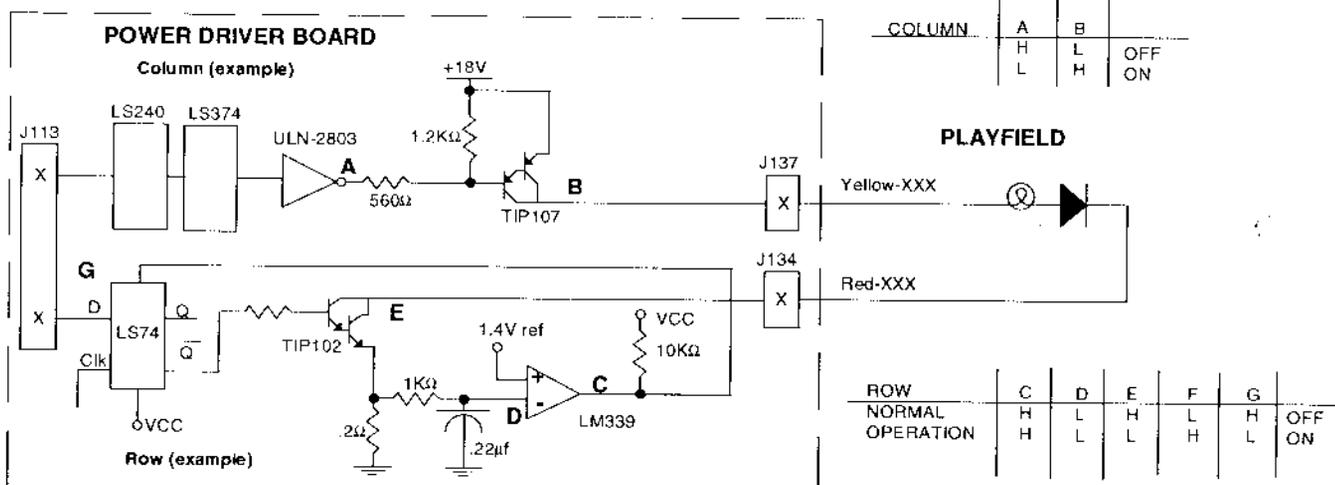
The processor sends a signal to the column circuit causing the output of the UNL-2803 to toggle. When point "A" drops low, the TIP107 transistor conducts and point "B" changes to a high state. At the same time, the processor drives the input of the 74LS74 low, causing a high at output "F". A high state at the base of TIP102 causes the transistor to conduct, bringing the row circuit to ground and turning the lamp on.
