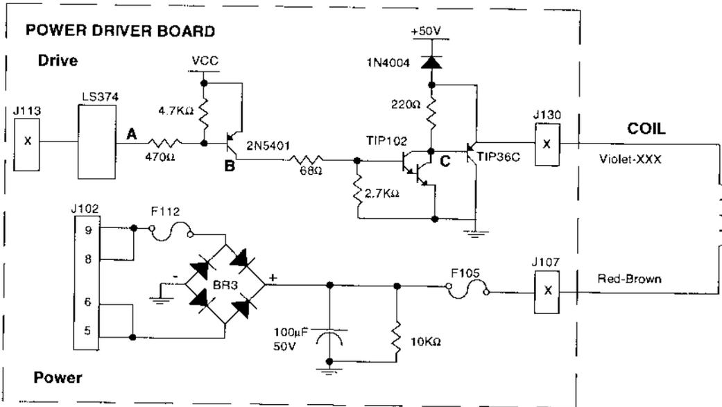
The processor toggles the output of the 74LS374. When point "A" is low, point "B" the collector of the 2N5401 transistor, is high. A high at point "B" causes point "C", the collector of the TIP102 transistor, and point "D", the emitter of the TIP36C transistor, to drop low. When point "D" is low, the coil is grounded through the transistor and turns on. The coil shuts off when point "A" toggles high.
