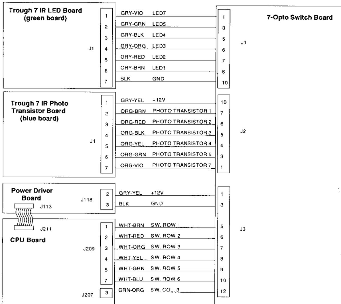
**NOTE: GRAY-BLUE AND ORANGE-BLUE WIRES FROM THE 7-OPTO SWITCH BOARD GO TO THE BALL POPPER AND ARE NOT PART OF THE OUTHOLE TROUGH CIRCUIT.**
