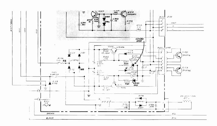
Figure 6 Schematic Diagram of Low-Voltage Power Supply
