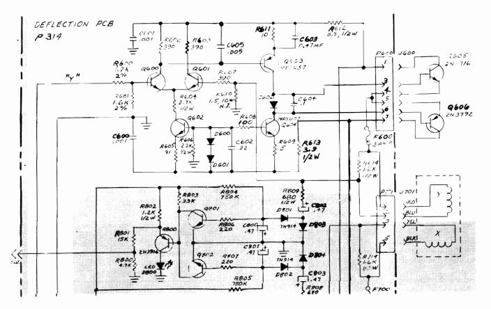
Figure 7 Schematic Diagram of Y Amplifier
