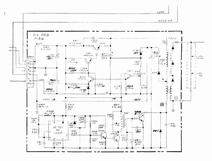
Figure 10 Schematic Diagram of High-Voltage Power Supply
