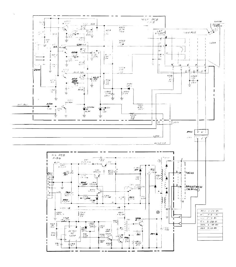
Figure 11 Monitor Schematic Diagram
