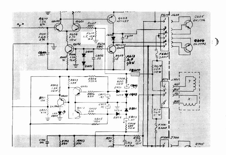
Figure 9 Schematic Diagram of Spot Killer Circuitry
