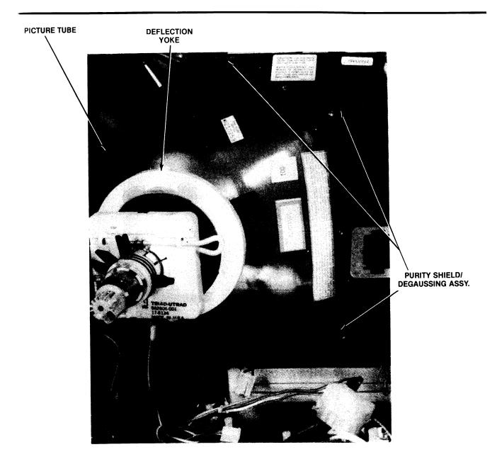
Figure 12 Monitor Assembly 92-053 C
