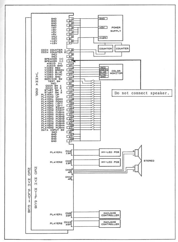
Set the switch on PCB on stereo position.
