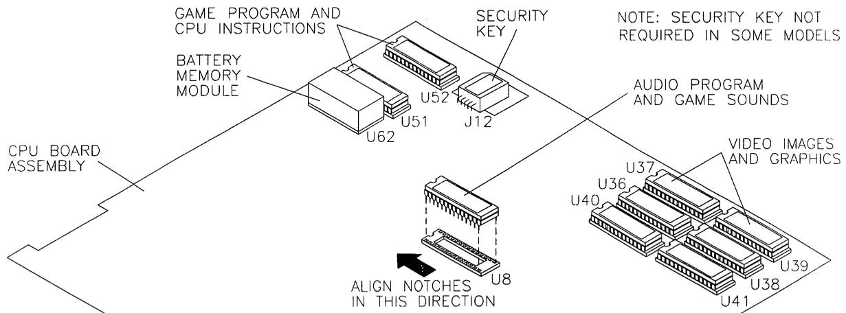
**ORIENTATION OF FIELD REPLACEABLE ELECTRONIC COMPONENTS**
