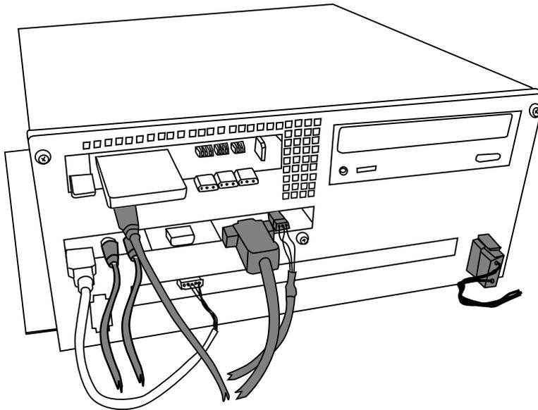
4. Slacken 4 off hex head nuts (M5) and remove the Game PCB Assy.
