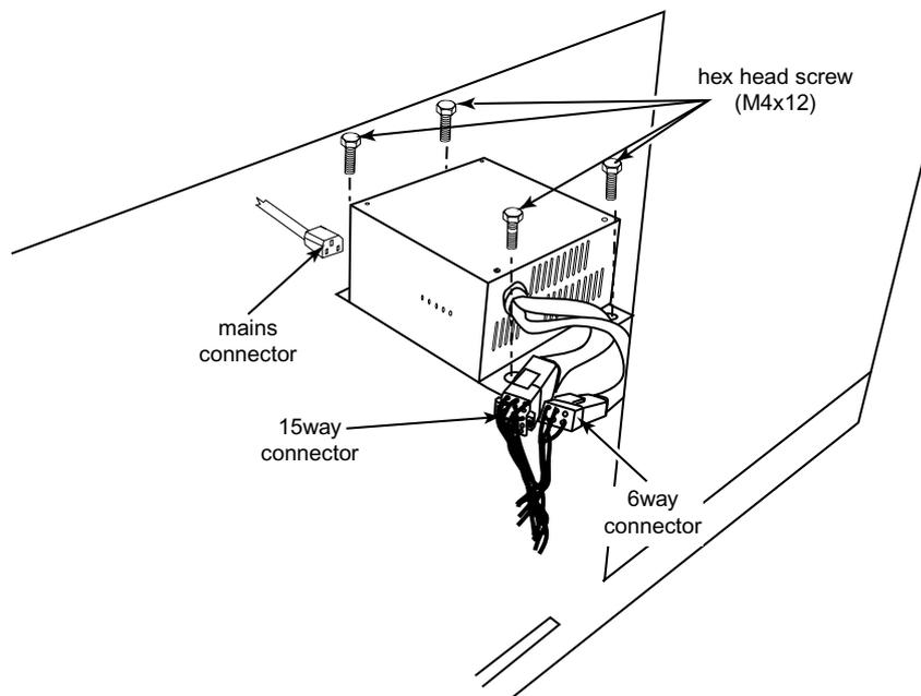
6. Remove 4 off hex head screws (M4x12) and remove the existing Power Supply.
