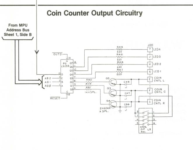
This circuit consists of coin counter drivers Q3, Q4, and Q5 and data latch P9. The circuit is addressed by the MPU on AB0-AB2 and written by the MPU on data line DB7. When the input to a driver is clocked high, its collector goes low grounding the return of the coin counter in the coin door.
