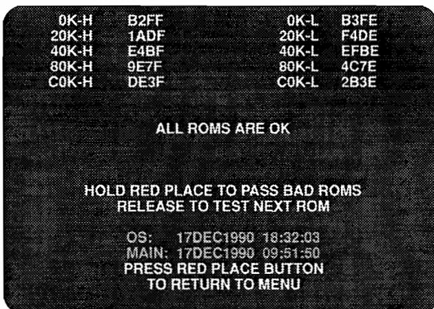
**Figure 2-8 Complete ROM Test Screen**
