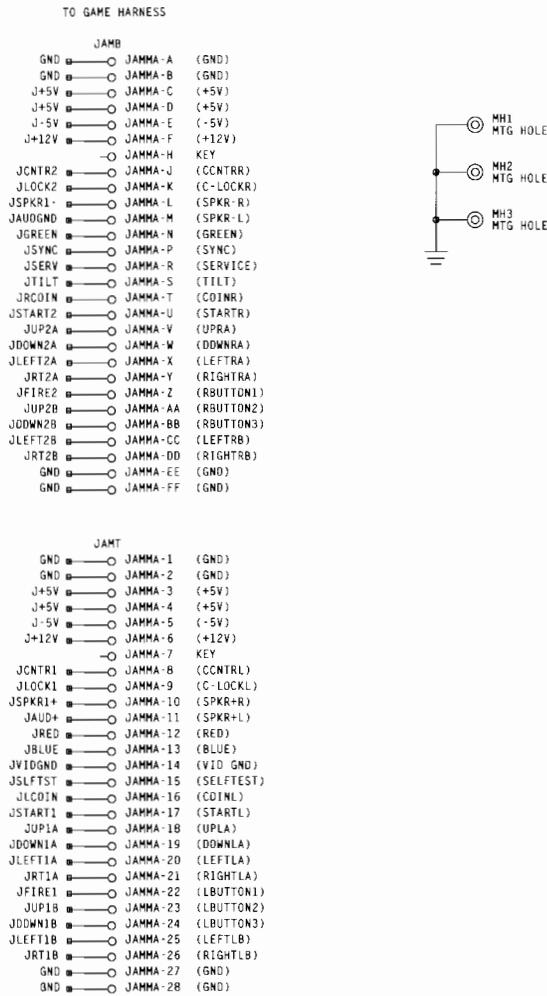
**Figure 5-4 JAMMA Filter PCB Schematic Diagram**
