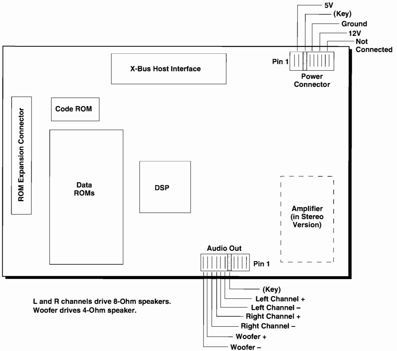
**Figure 5-6 CH31\_2 (CAGE Audio) Board Block Diagram**
