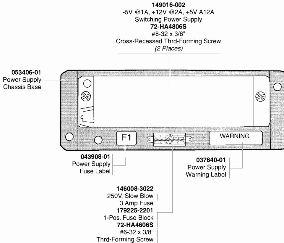
**Figure 4-2 Power Supply Assembly**
