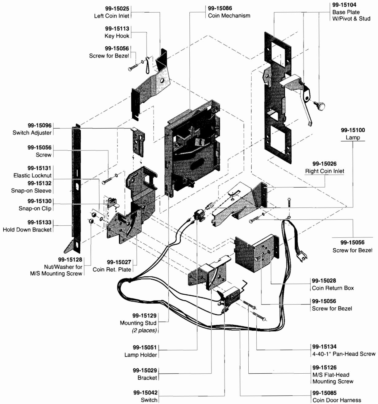
**Figure 4-3 Over/Under Coin Door Assembly**
