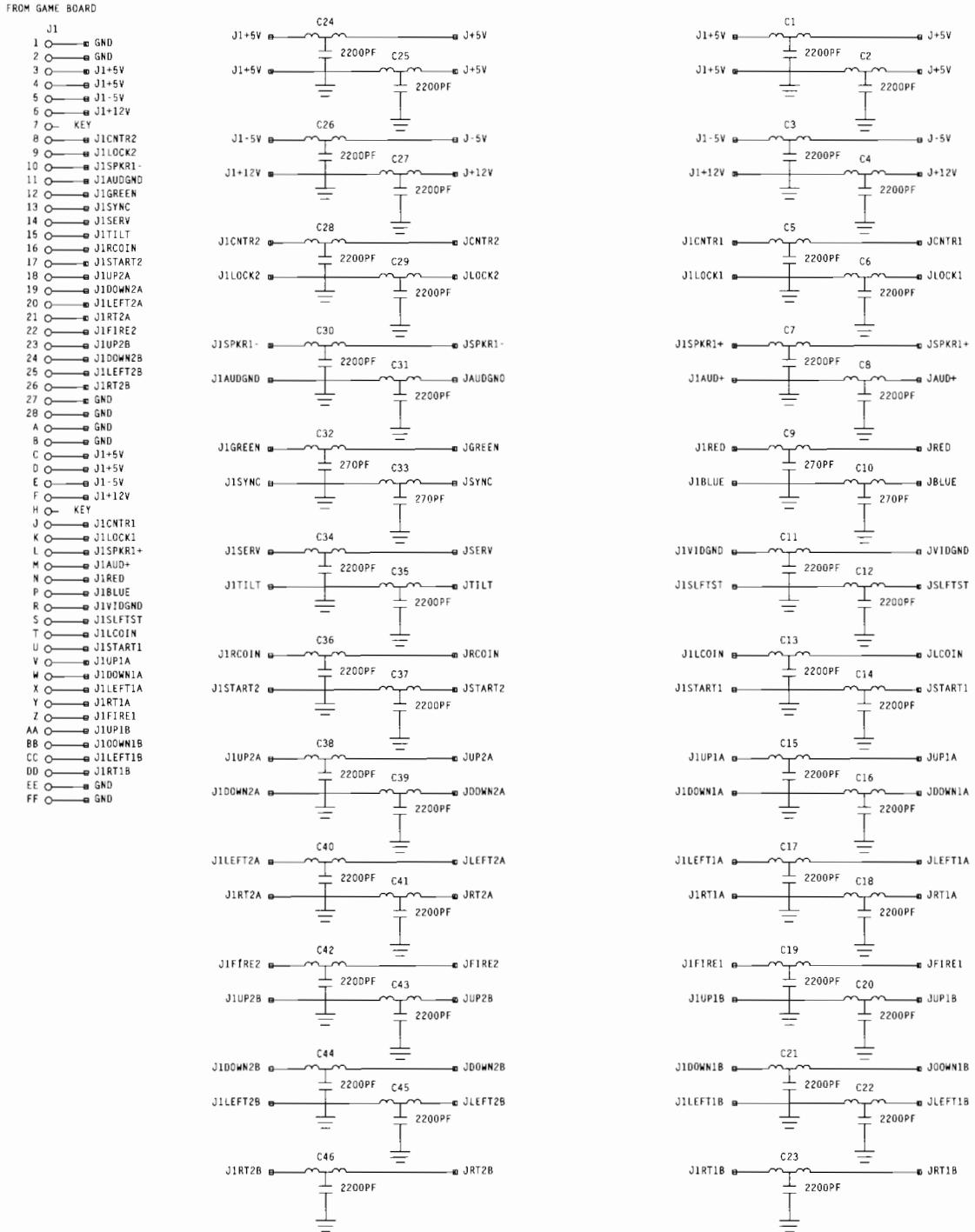
Figure 5-4 JAMMA Filter PCB Schematic Diagram
