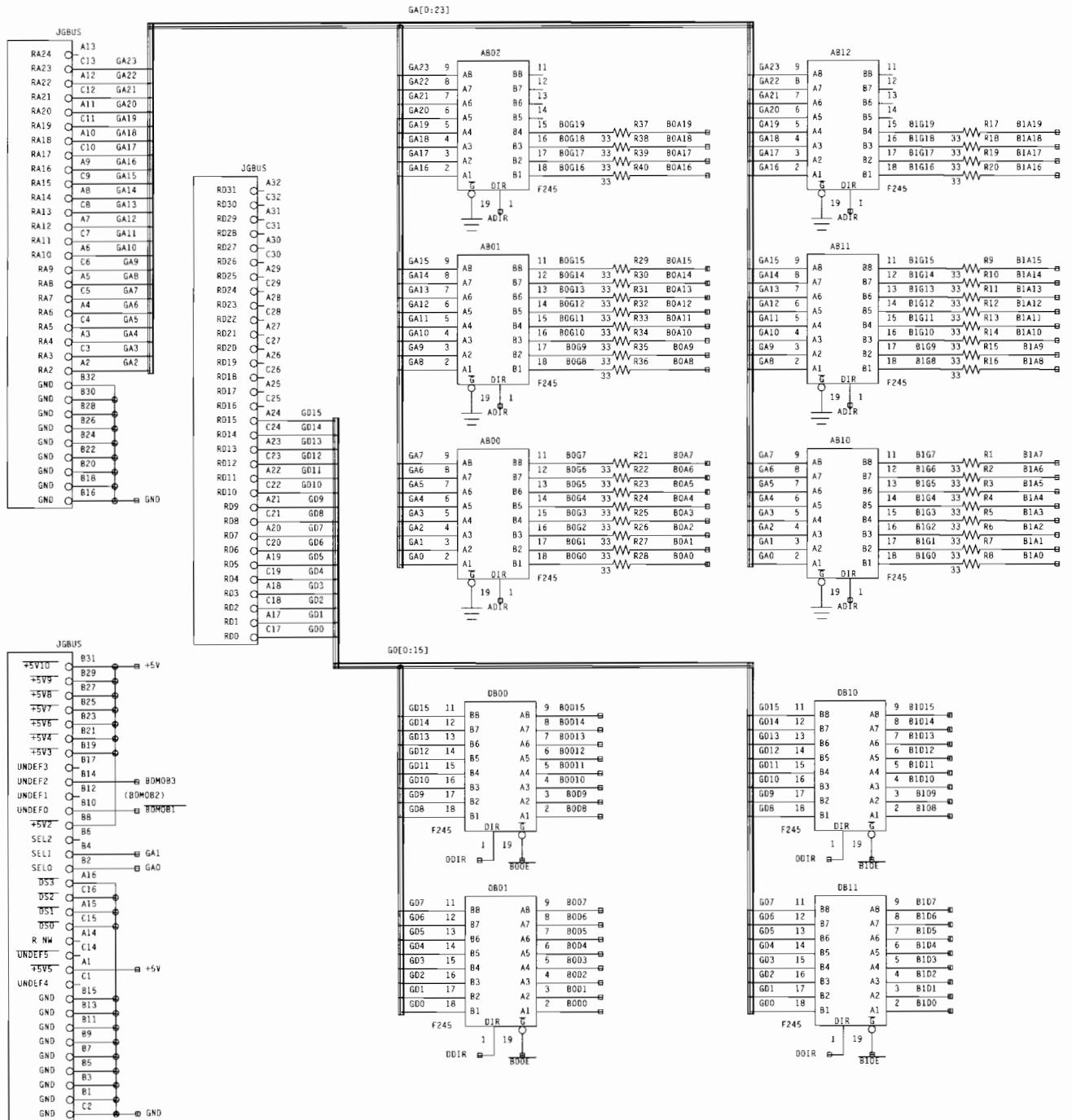
Figure 5-3 GT24M8 PCB Schematic Diagram
