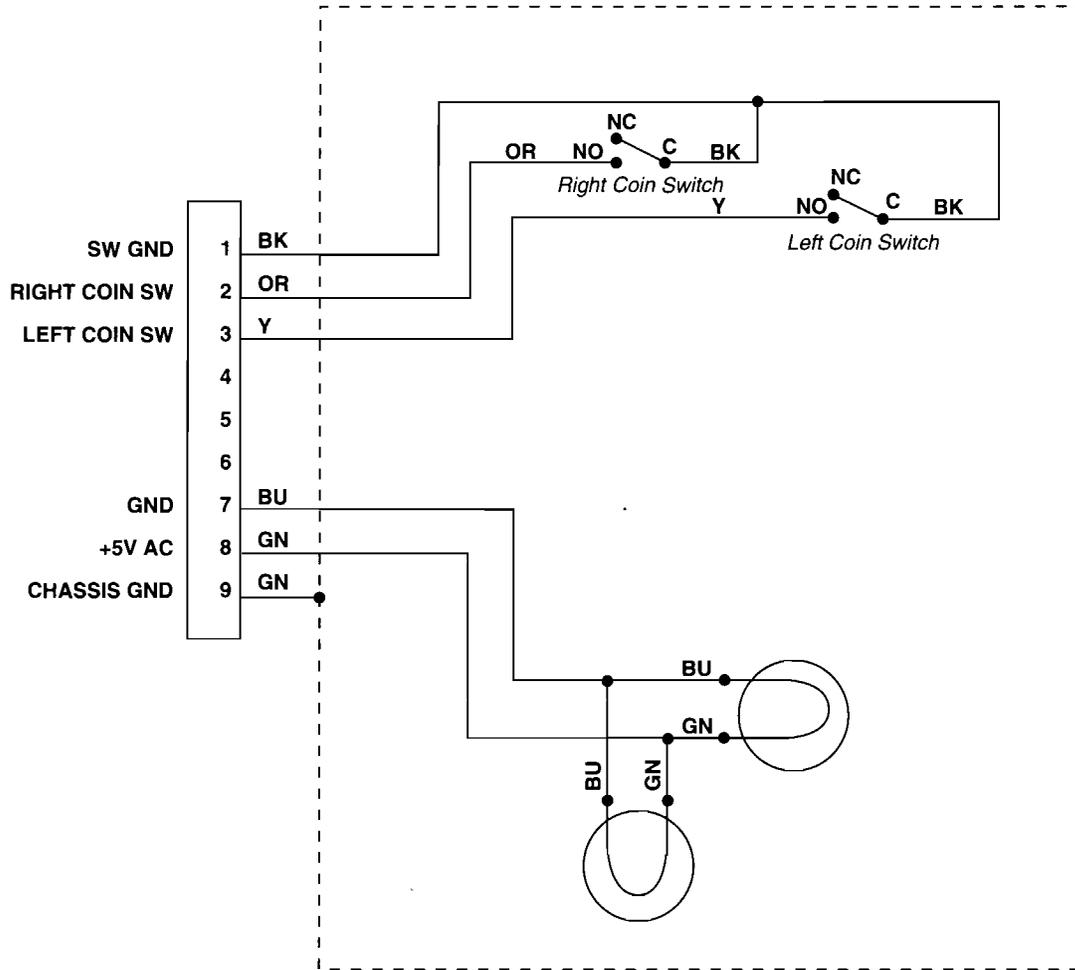
**Figure 5-2 Coin Door Wiring Diagram**
