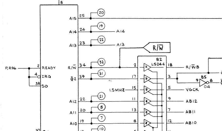
NOTE: THE MPU IN THIS GAME OPERATES AT A FREQUENCY OF 1.5 MHZ. THEREFORE THE MPU CHIP MUST BE 6502A. THE 6502'S MAXIMUM FREQUENCY IS 1 MHZ AND IS NOT COMPATIBLE WITH THIS GAME.
