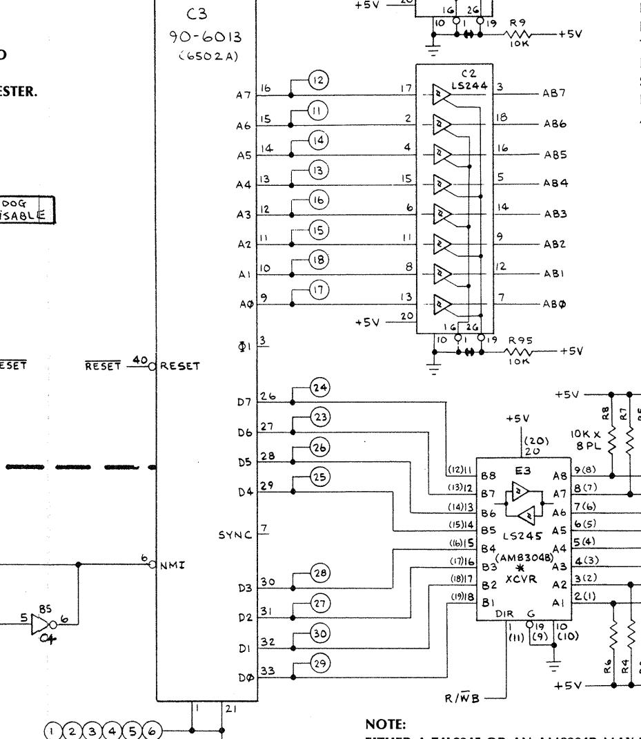
NOTE: DO NOT USE SPLIT PADS ON PCB FOR TROUBLESHOOTING PURPOSES. IF A 74LS244 IS INSTALLED AT LOCATION B2 AND/OR C2, THE SPLIT PAD FOR THAT LOCATION SHOULD BE FILLED WITH SOLDER. IF A 74LS241 IS USED, THE APPROPRIATE SPLIT PAD SHOULD BE OPEN.
