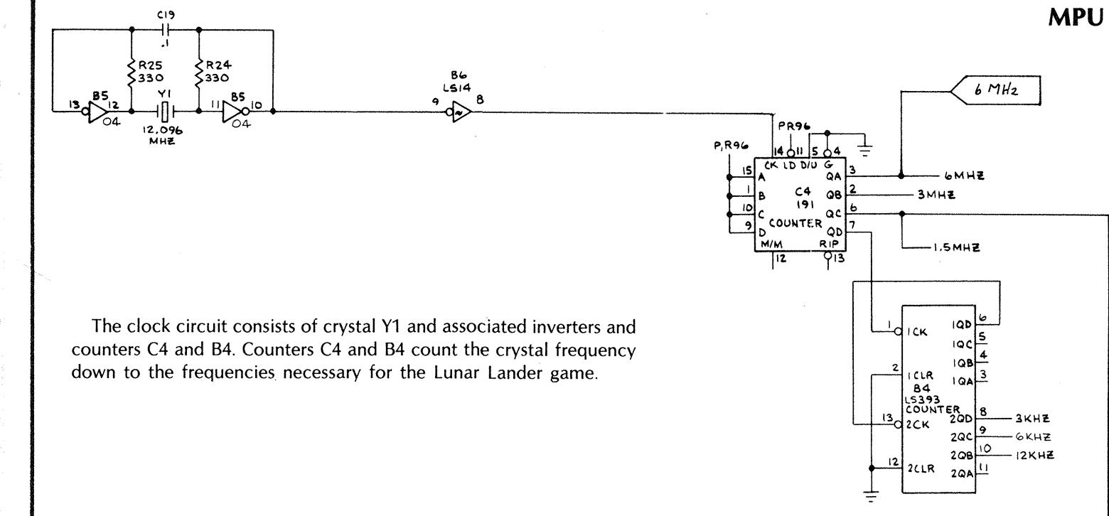
The clock circuit consists of crystal Y1 and associated inverters and counters C4 and B4. Counters C4 and B4 count the crystal frequency down to the frequencies necessary for the Lunar Lander game.
