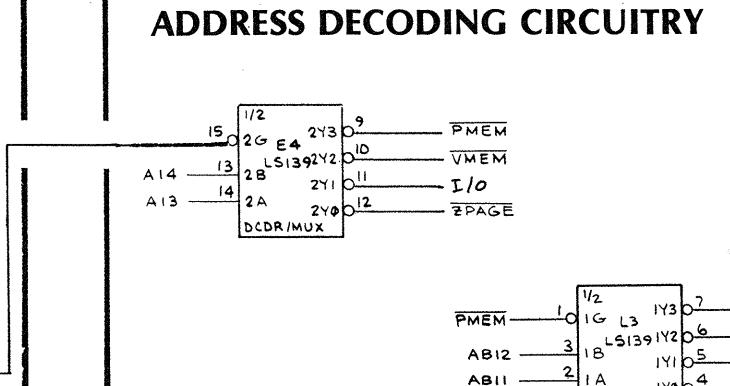
The address decoder performs the function of turning on or off the appropriate circuitry at the critical time, so that information can be transferred back and forth between the game circuitry and the MPU. The memory map below is for the Lunar Lander game.
