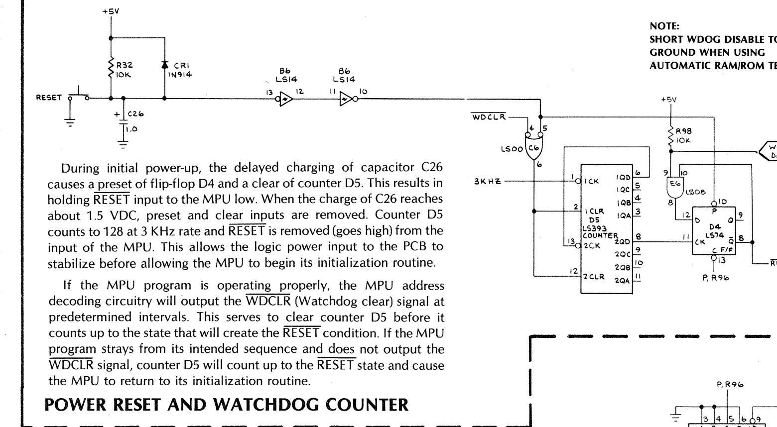
NOTE: SHORT WDOG DISABLE TO GROUND WHEN USING AUTOMATIC RAM/ROM TESTER.
