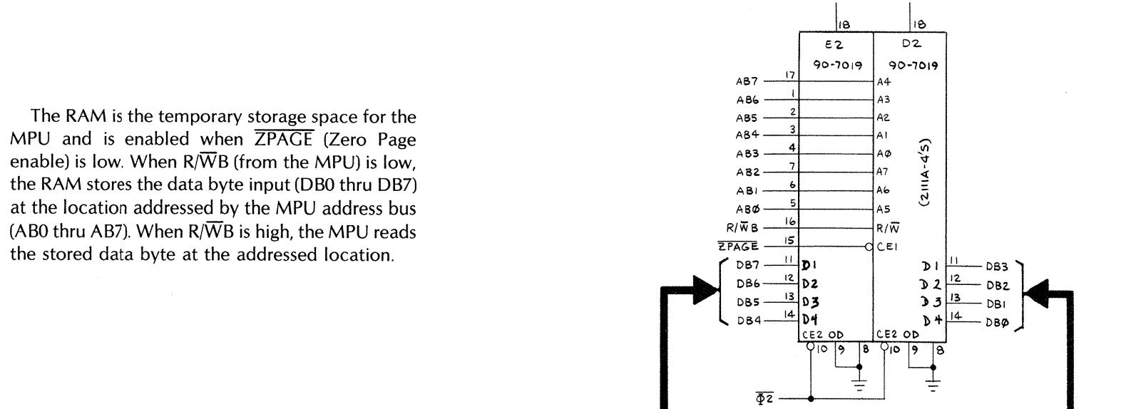
The RAM is the temporary storage space for the MPU and is enabled when ZPAGE (Zero Page enable) is low. When R/WB (from the MPU) is low, the RAM stores the data byte input (DB0 thru DB7) at the location addressed by the MPU address bus (AB0 thru AB7). When R/WB is high, the MPU reads the stored data byte at the addressed location.
