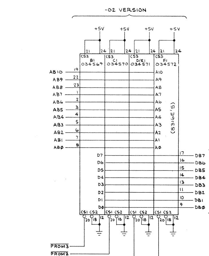
Program Memory for the Lunar Lander game is contained in PROMs for the -01 version of the PCB or ROMs for the -02 version of the PCB. One ROM is equivalent to four PROMs. All PROMs connected to a common enable must be removed before replacing with a ROM. For example, remove PROMs at locations F1, H1, and M1 before replacing with ROM at location F1. A ROM/PROM equivalent chart is contained in Chapter 5, Illustrated Parts Catalog, of the Lunar Lander game manual.
