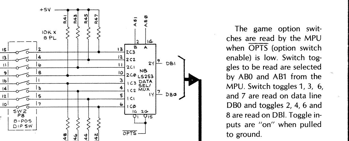
The game option switches are read by the MPU when OPTS (option switch enable) is low. Switch toggles to be read are selected by AB0 and AB1 from the MPU. Switch toggles 1, 3, 6, and 7 are read on data line DB0 and toggles 2, 4, 6 and 8 are read on DB1. Toggle inputs are "on" when pulled to ground.
