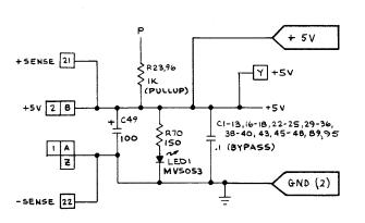
This circuitry consists of the PCB inputs and outputs for the +5 VDC logic power and 36 VAC input to the on board regulators. The +5 VDC inputs and outputs are discussed on the Sheet 1. Side A of this schematic set.
