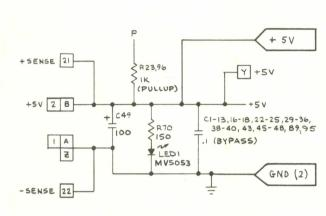
This circuitry consists of the PCB inputs and outputs for the +5 VDC logic power and 36 VAC input to the on board regulators. The +5 VDC inputs and outputs are discussed on the Sheet 1, Side A of this schematic set.
