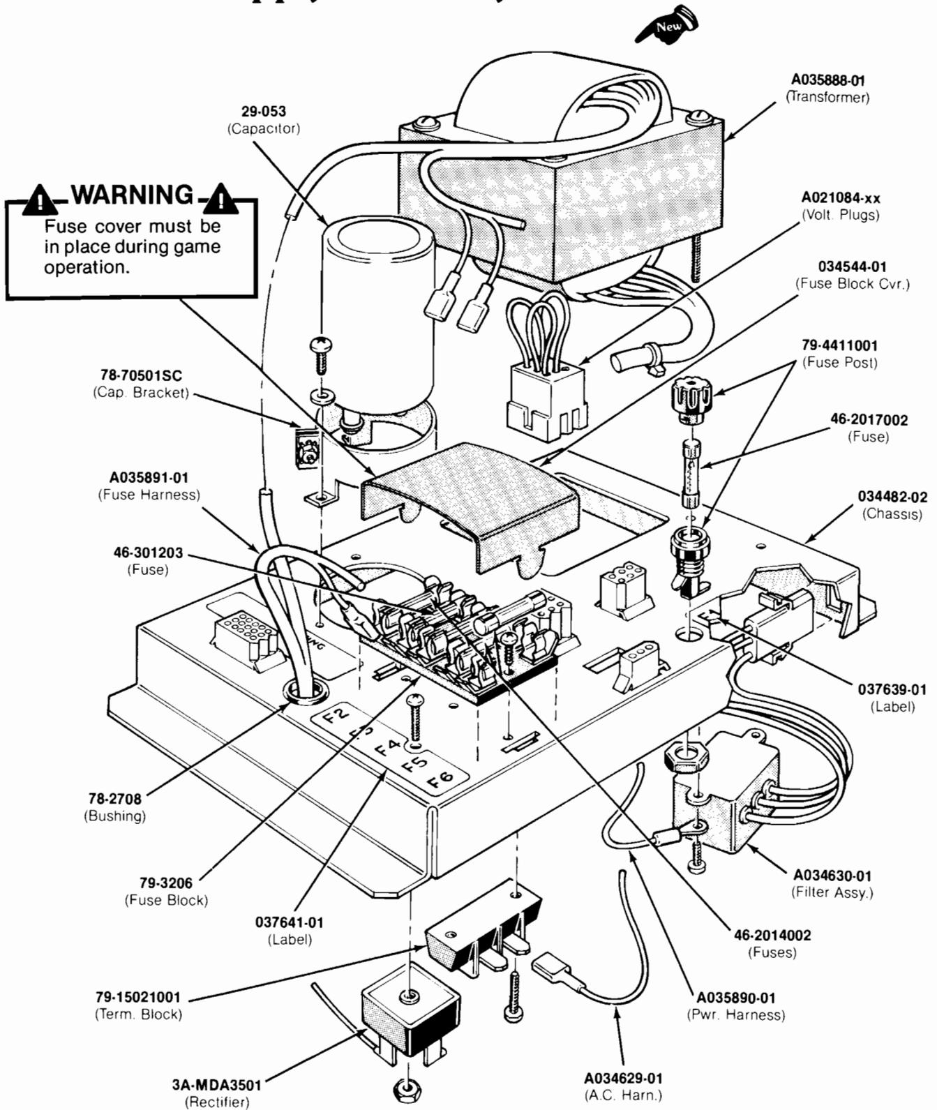
**Figure 3-12 Power Supply Assembly
