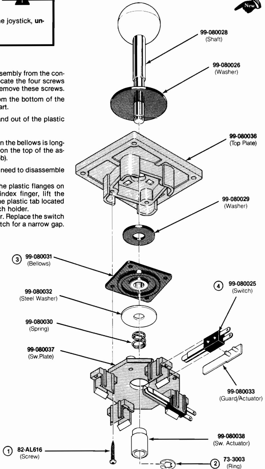
**Figure 3-4 8-Position Joystick Assembly
