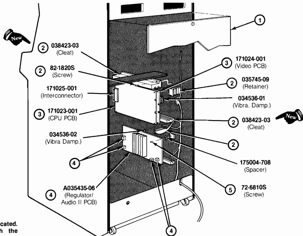
Figure 3-8 Printed-Circuit Board Removal
