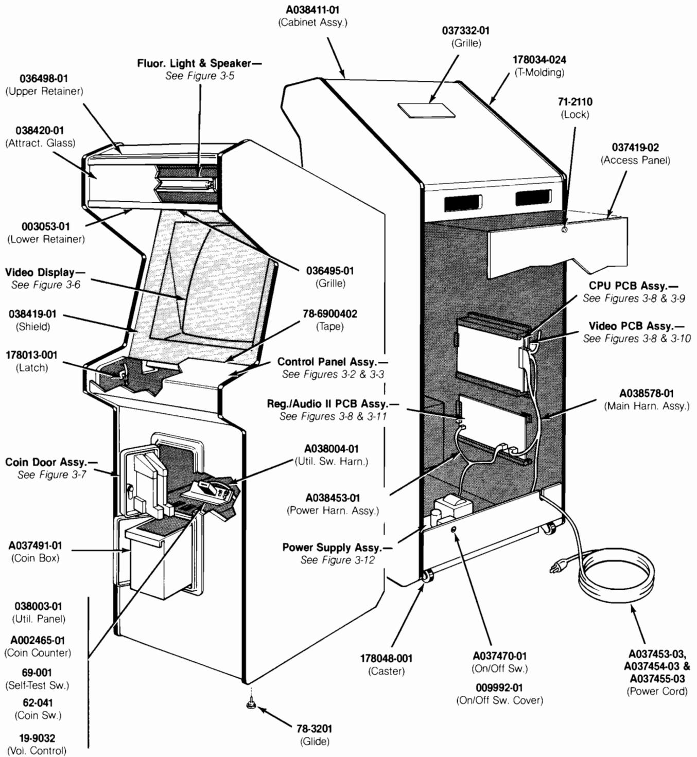
Figure 3-1 Cabinet-Mounted Assemblies
