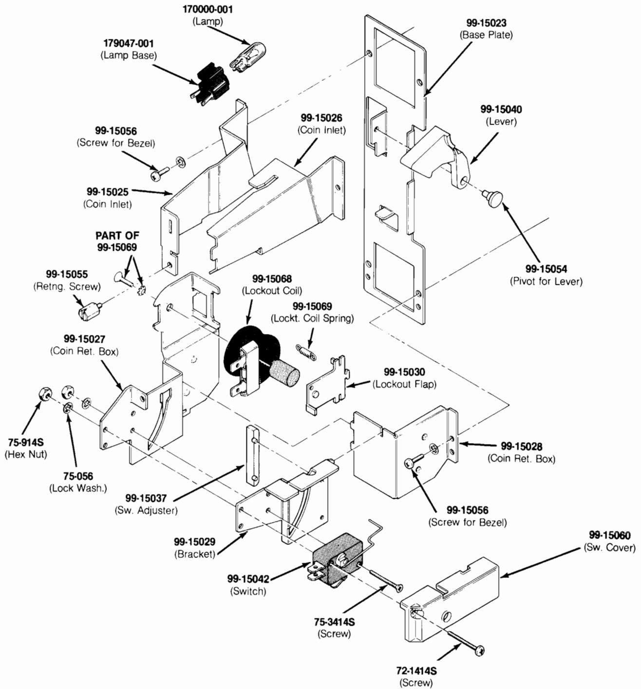
**Figure 3-7 Vertically Mounted Coin Door
