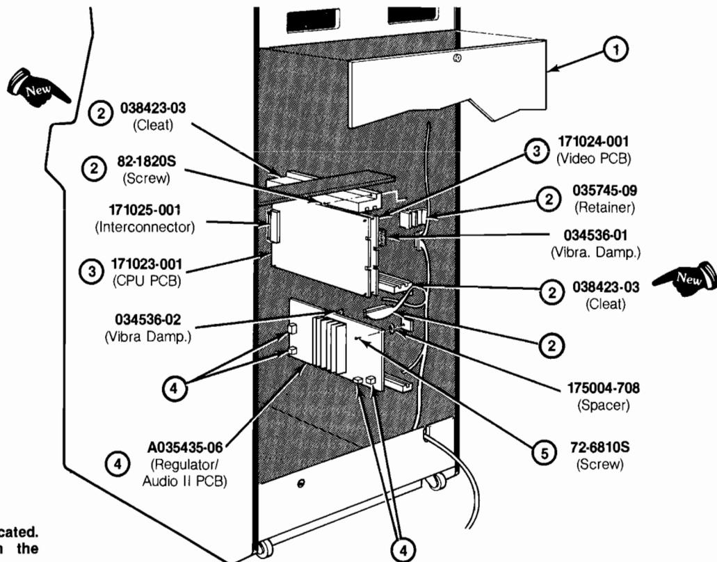
Figure 3-8 Printed-Circuit Board Removal
