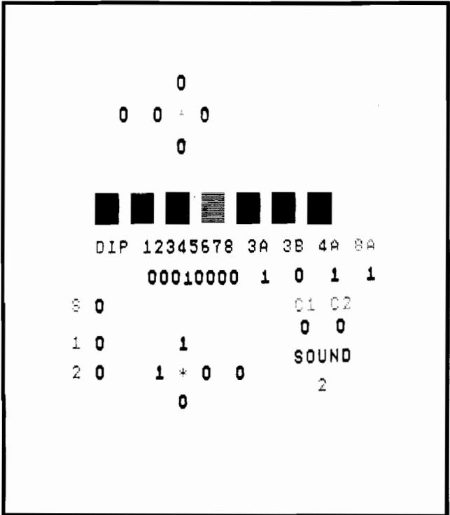
Figure 2-1 Self-Test Screen 1
