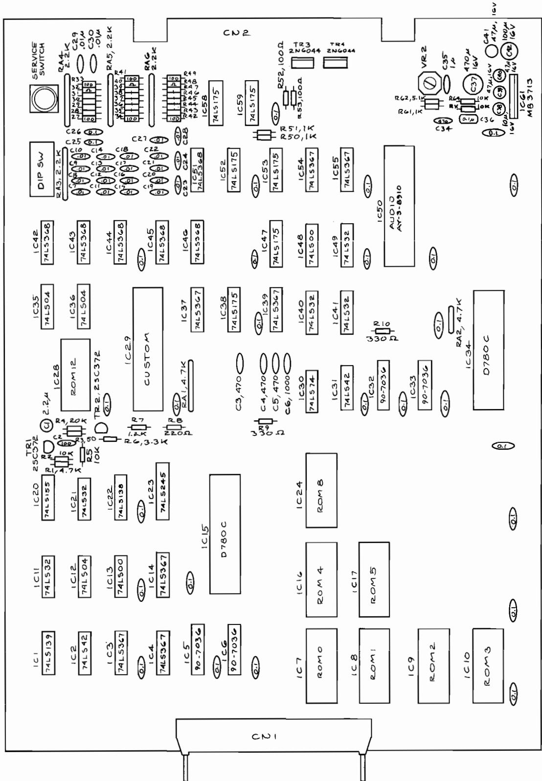
Figure 3-9 Kangaroo™ Central Processing Unit PCB Assembly
