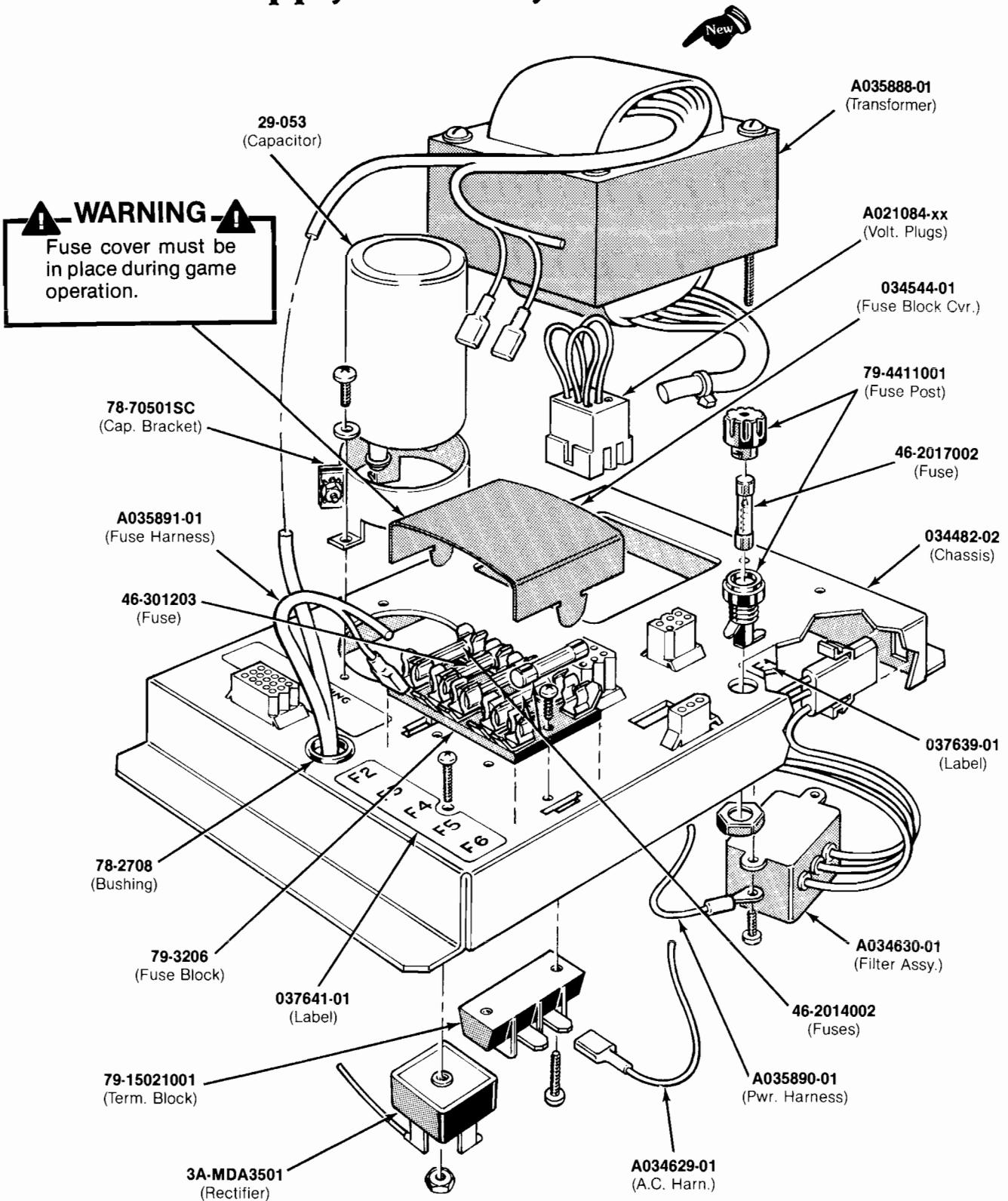
Figure 3-12 Power Supply Assembly
