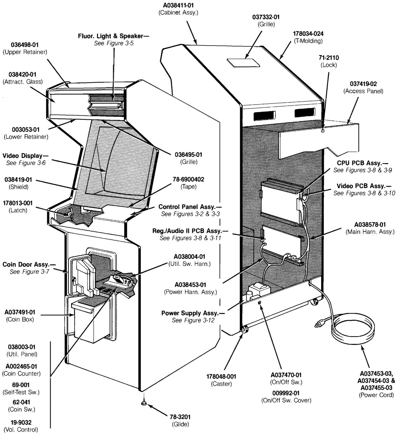
Figure 3-1 Cabinet-Mounted Assemblies
