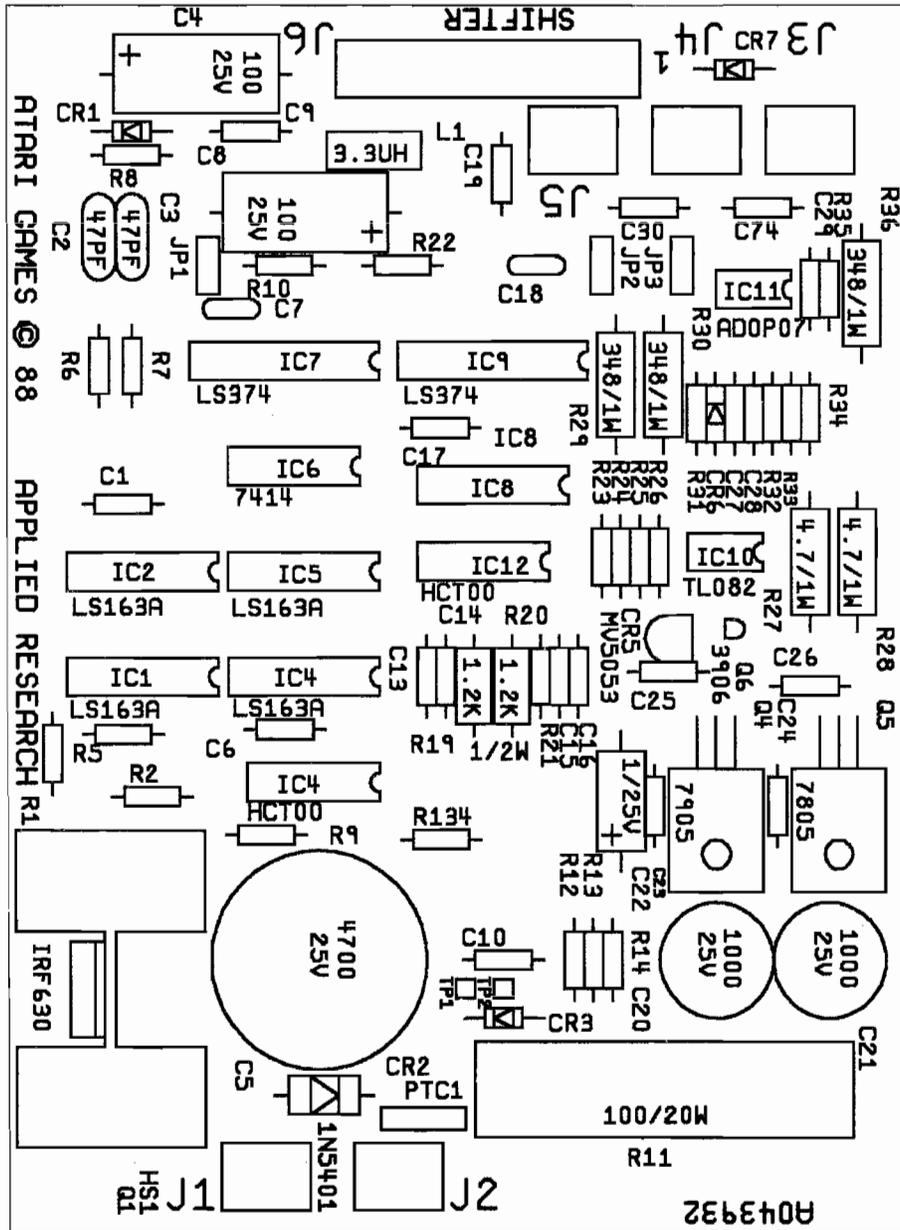
Figure 4-13 Shifter PCB Assembly
