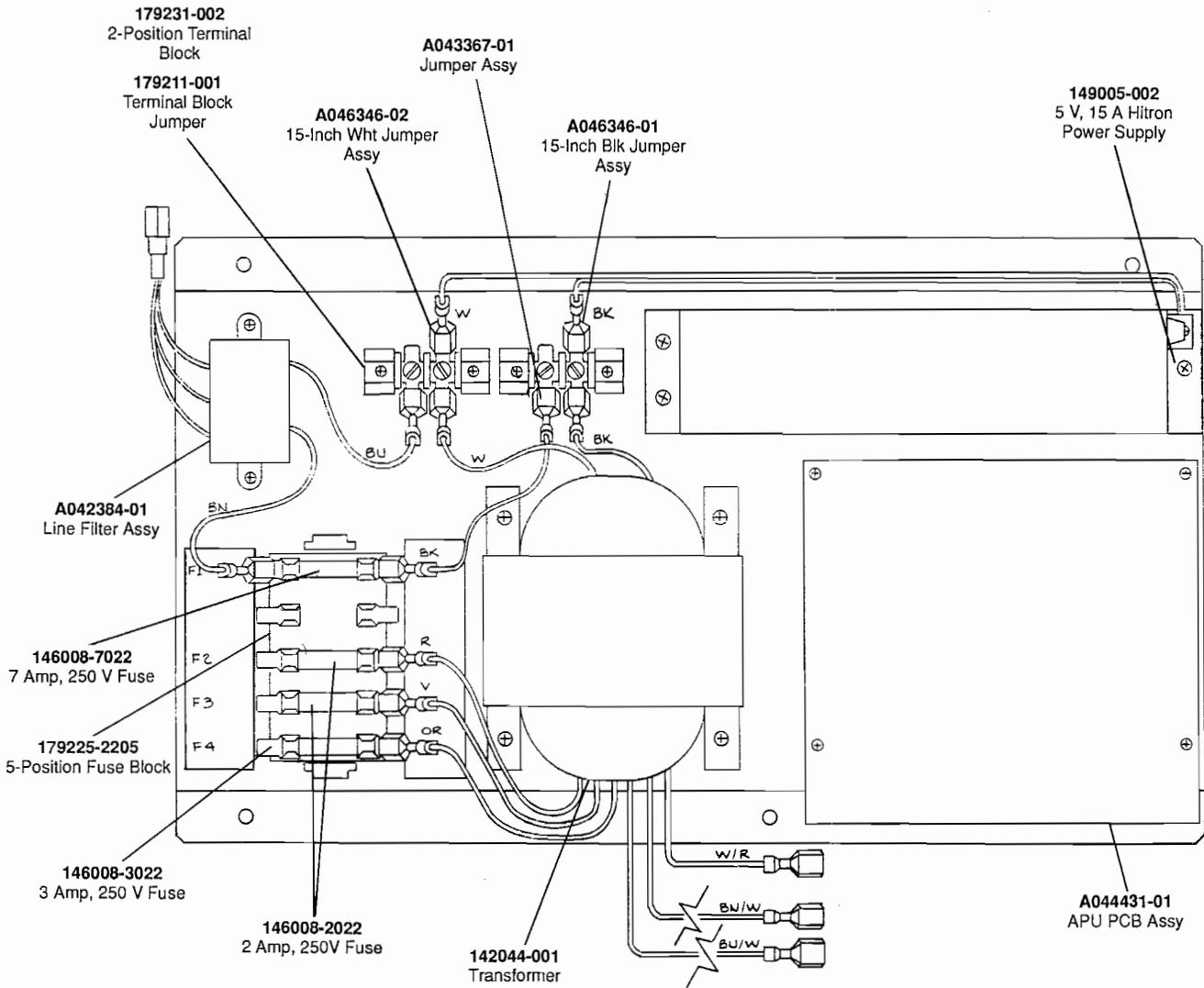
**Figure 4-10 Power Supply Assembly
