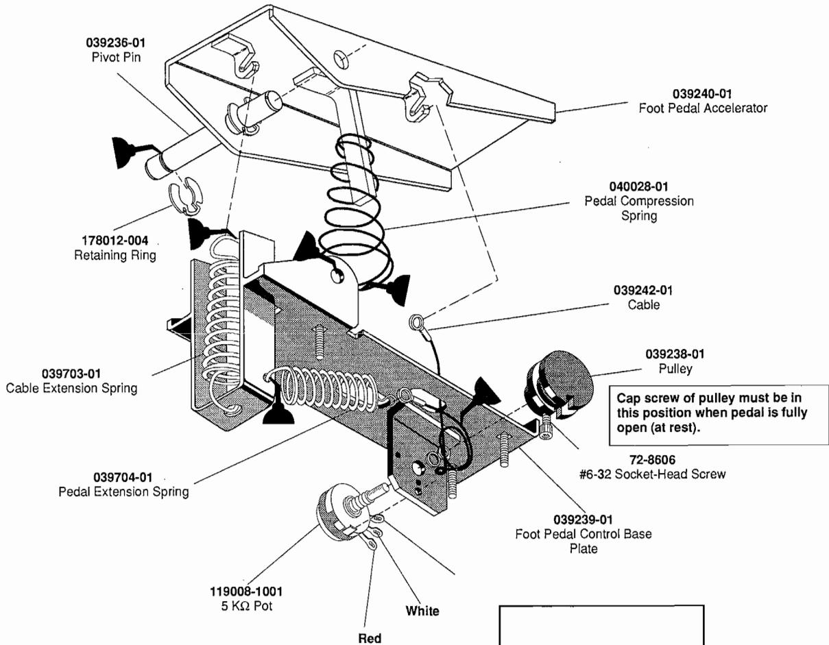
Cap screw of pulley must be in this position when pedal is fully open (at rest).
