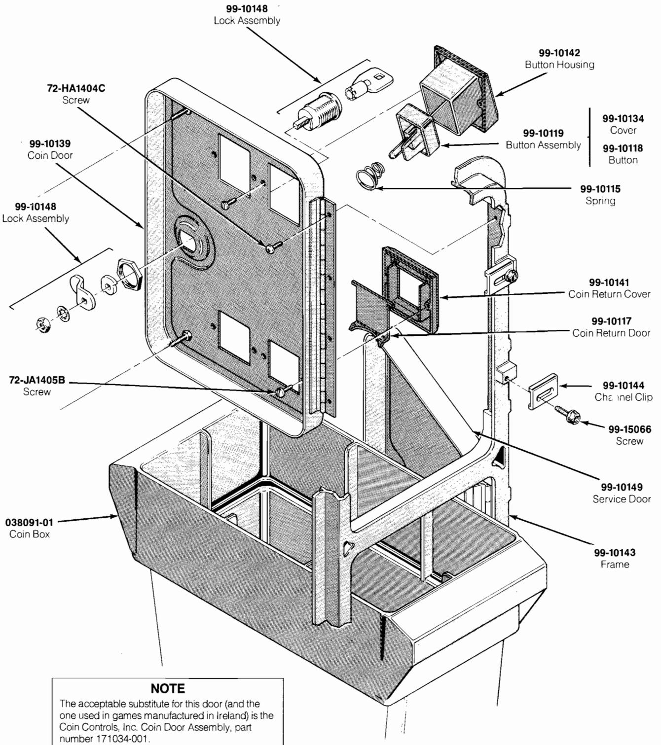
Figure 4-9 Coin Acceptors, Inc. Coin Door Assembly, Continued
