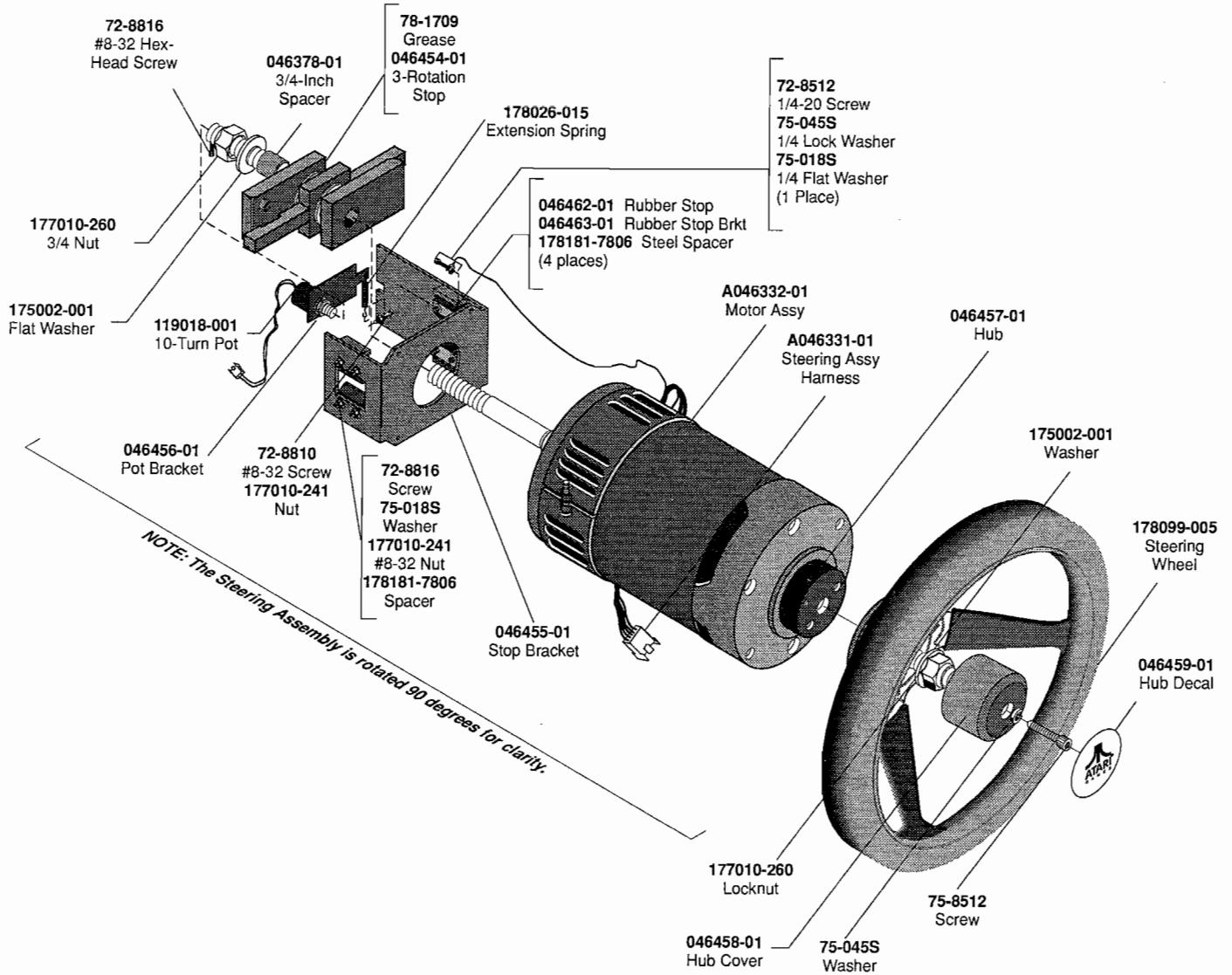
**Figure 4-5 Steering Assembly
