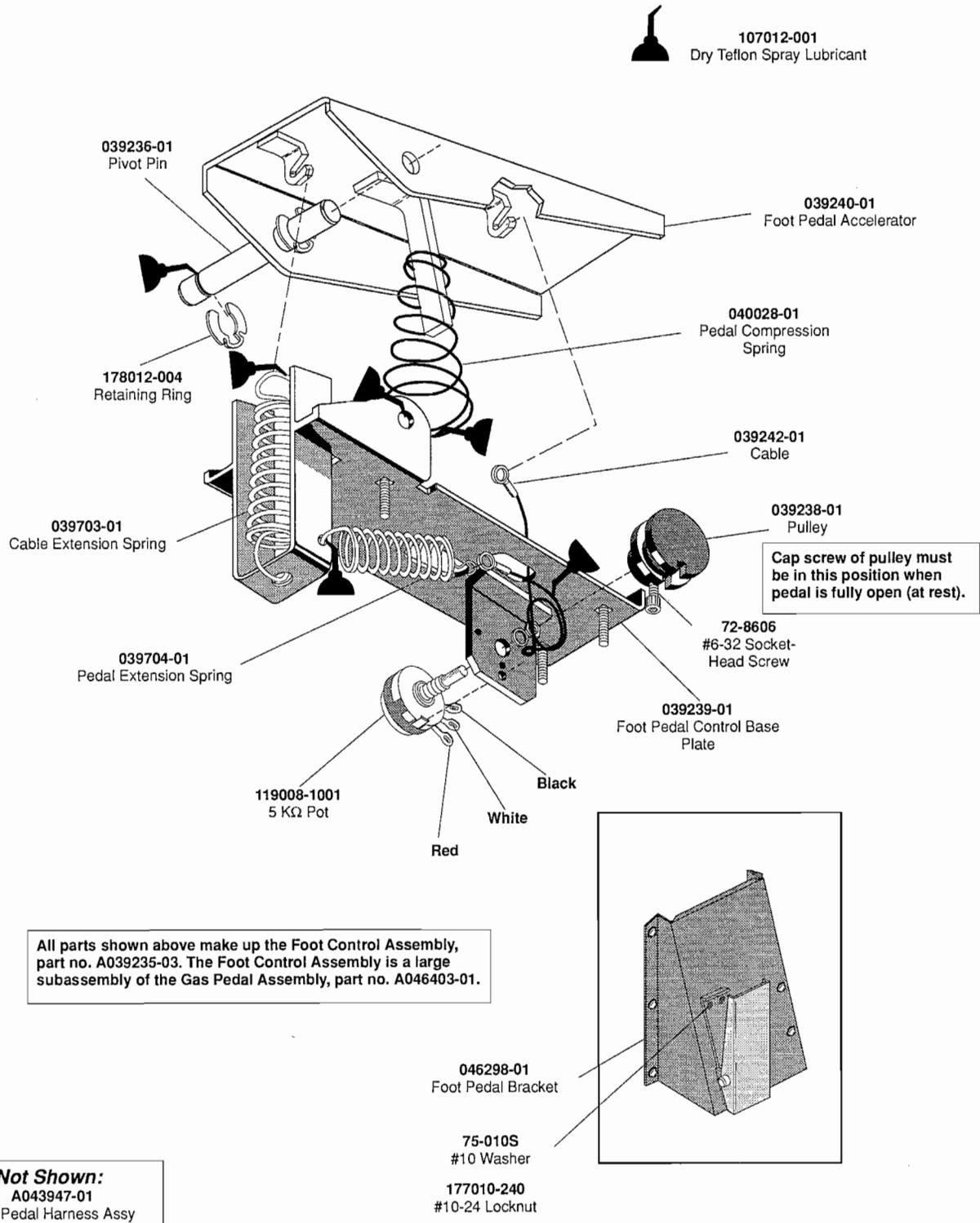
**Figure 4-8 Gas Pedal Assembly
