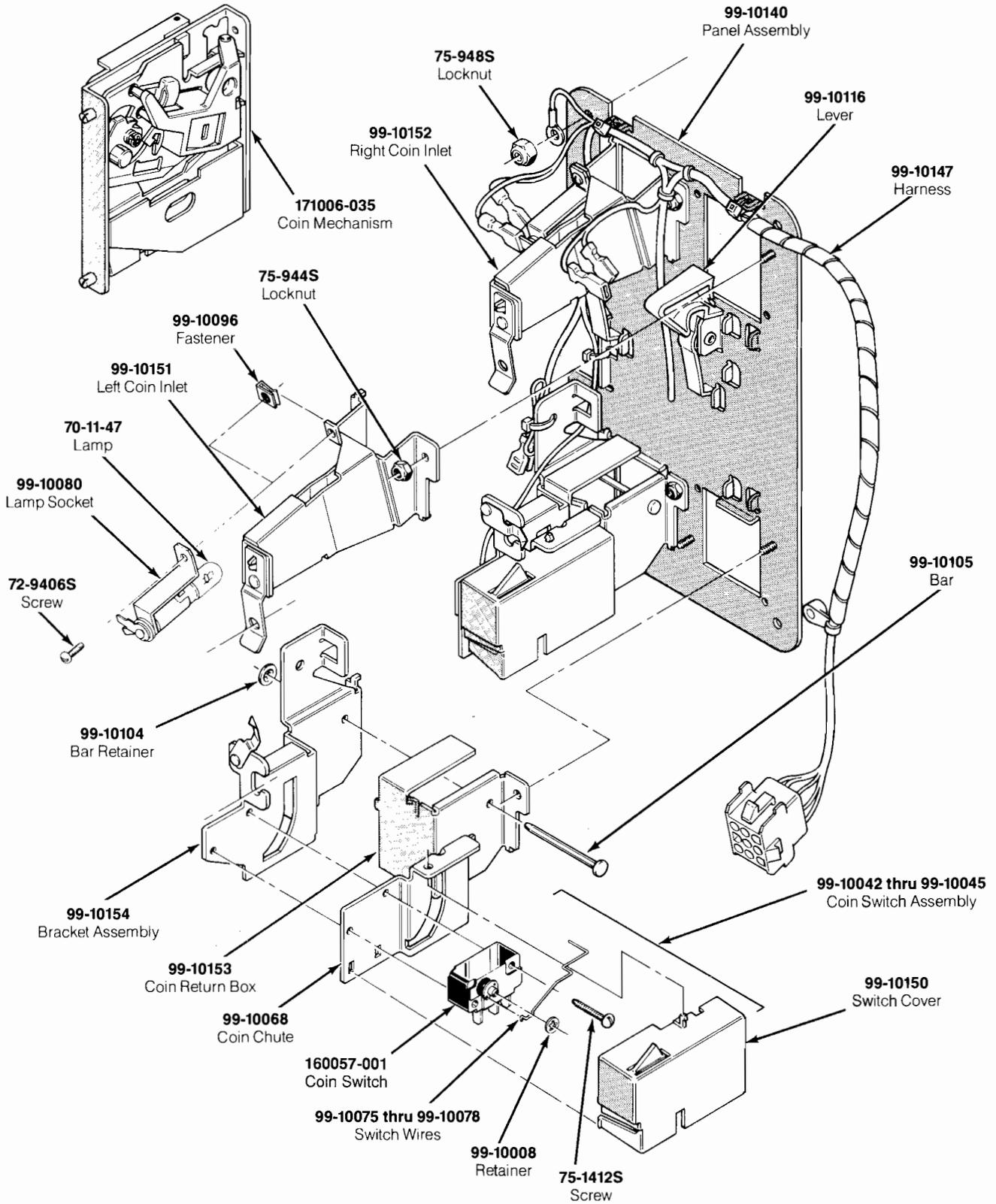
**Figure 4-9** Coin Acceptors, Inc. Coin Door Assembly
