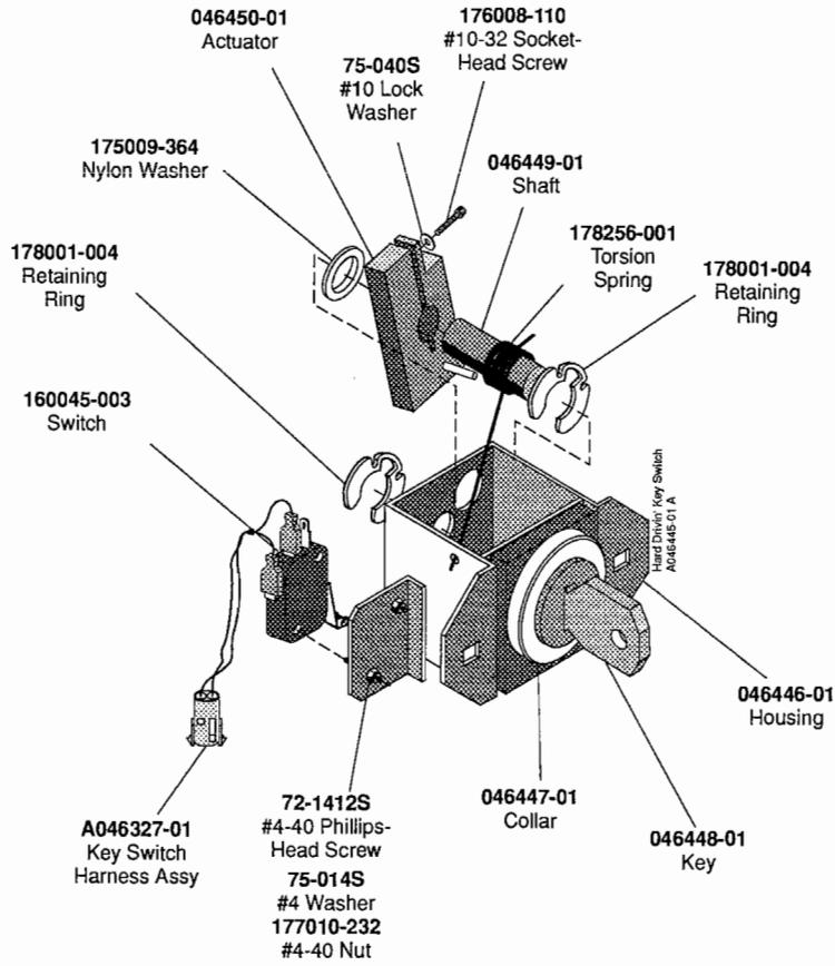
**Figure 4-4 Key Switch Assembly
