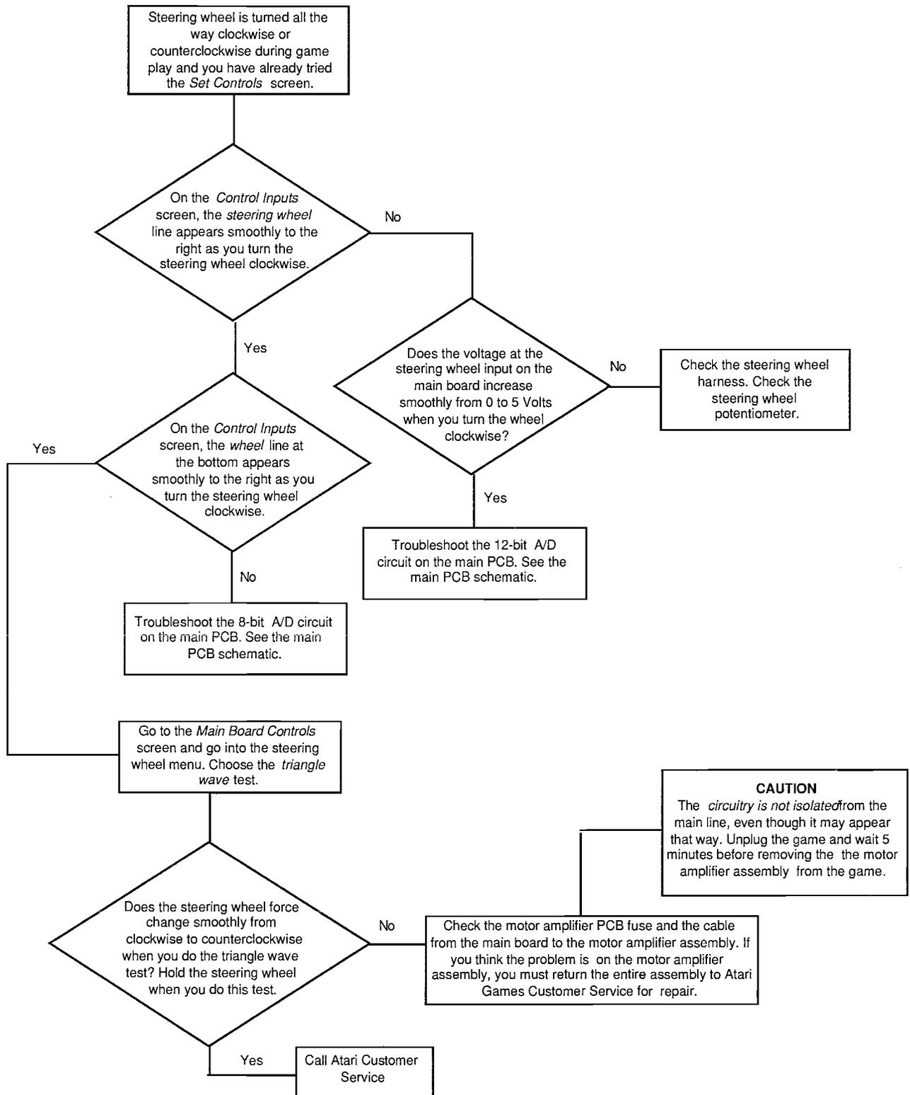
**Figure 3-3 Steering Wheel is Turned All the Way to One Side or the Other and You Have Tried the Set Controls Screens**
