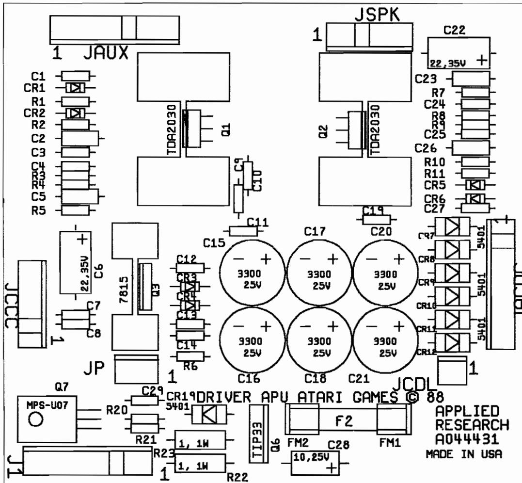
Figure 4-12 APU PCB Assembly
