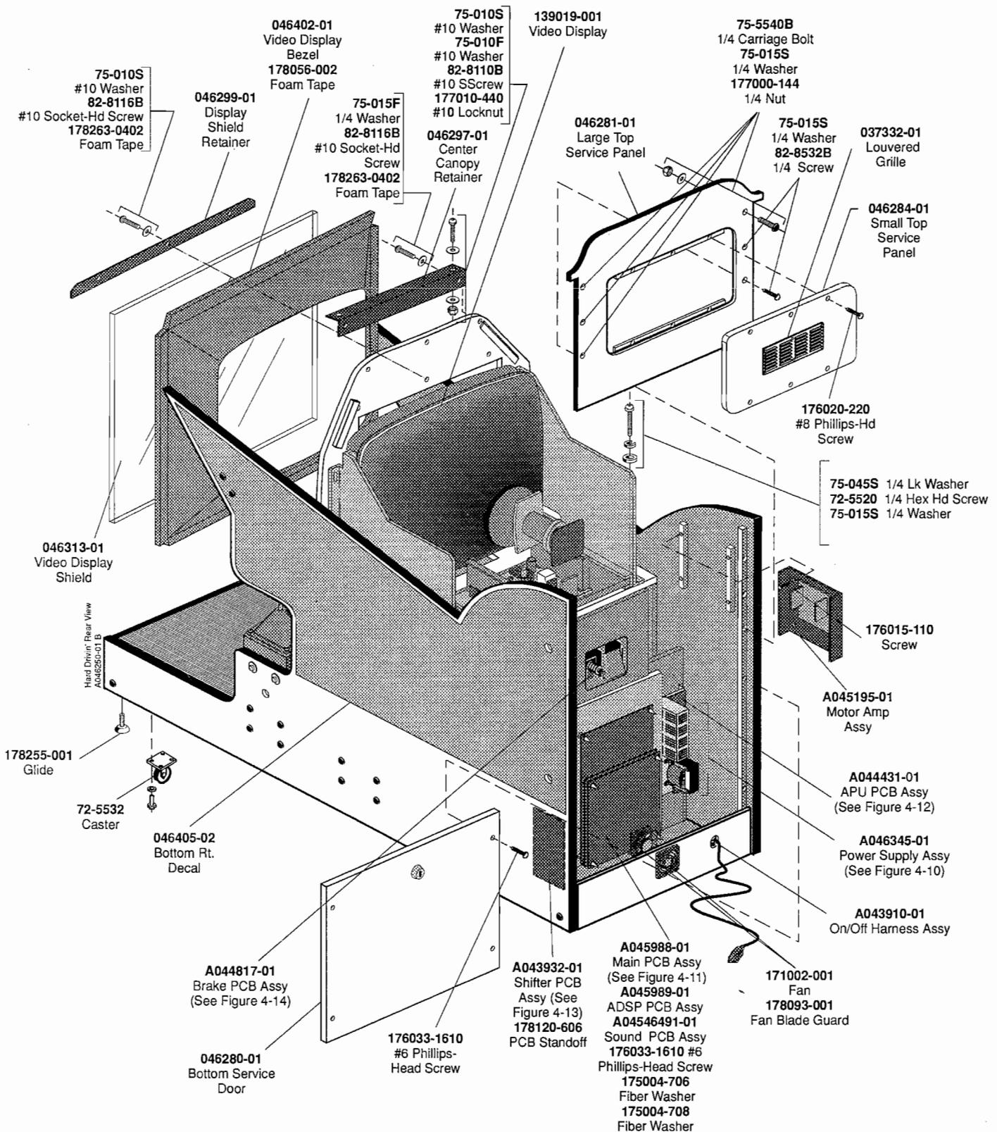
**Figure 4-1 Cabinet-Mounted Assemblies, Rear View
