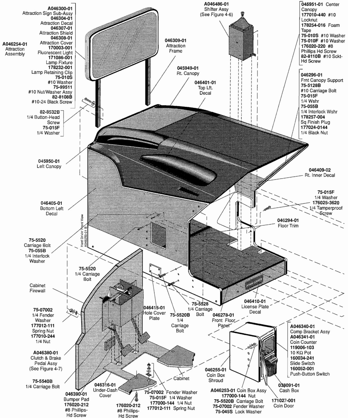
**Figure 4-1 Cabinet-Mounted Assemblies, Front View
