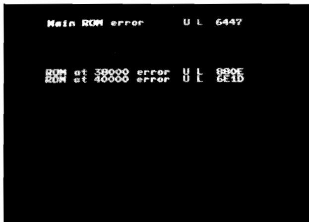
Figure 3-2 ROM Test Fails
