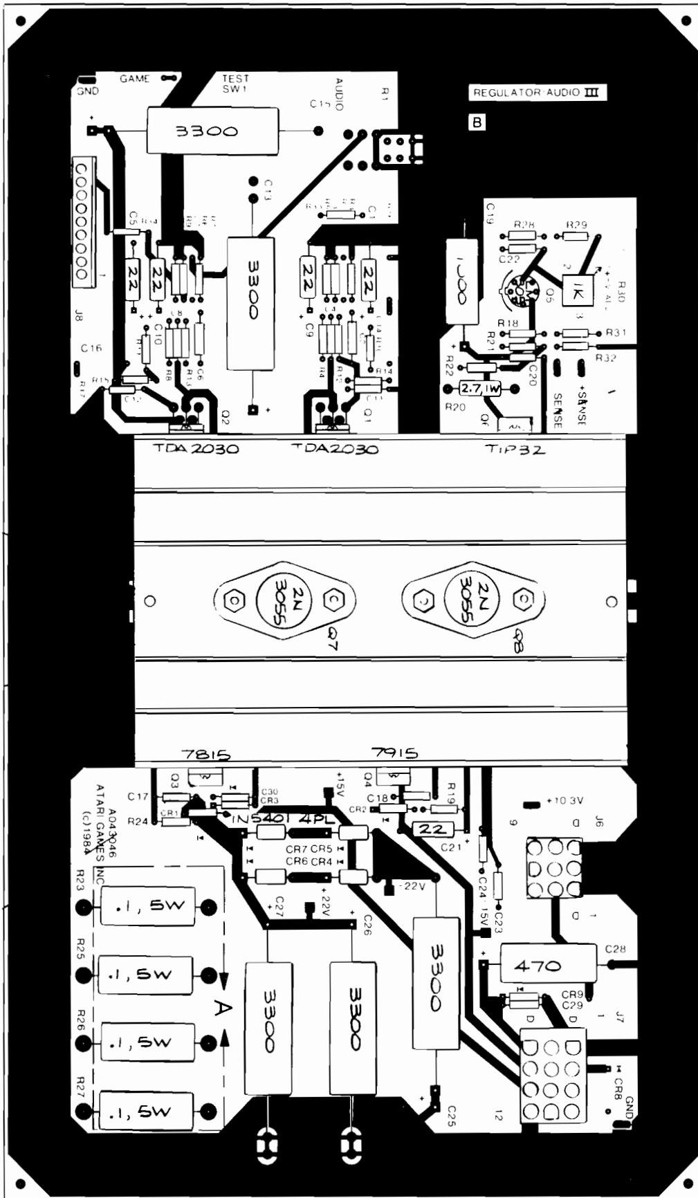
Figure 5-10 Regulator/Audio III Printed-Circuit Board Assembly
