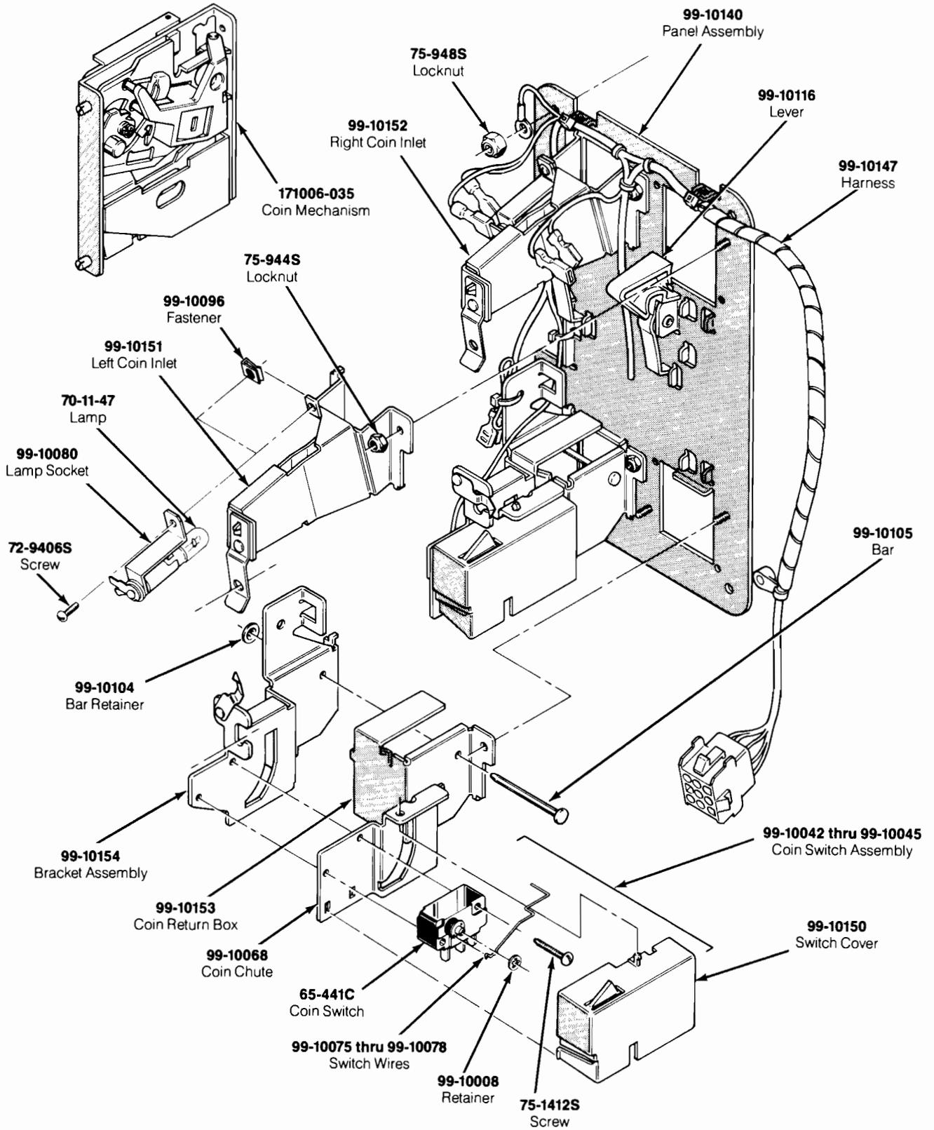
**Figure 5-7** Coin Acceptors, Inc. Coin Door Assembly
