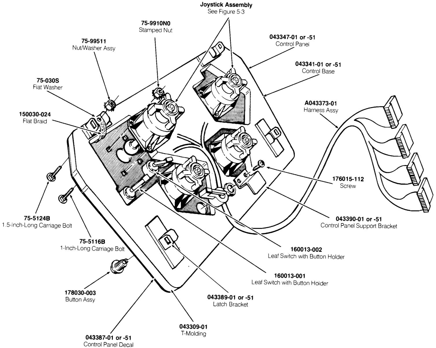
**Figure 5-2 Control Panel Assembly**
