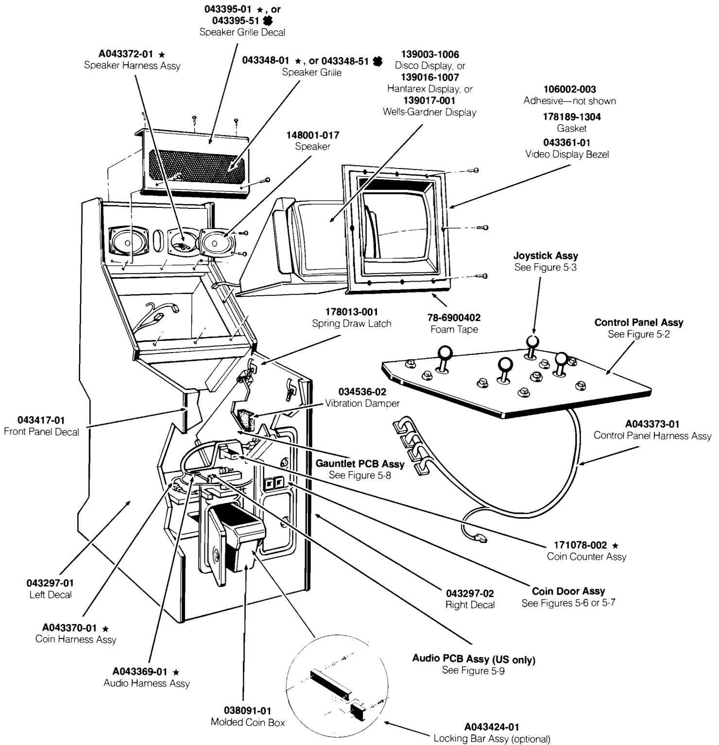
**Figure 5-1 Cabinet-Mounted Assemblies
