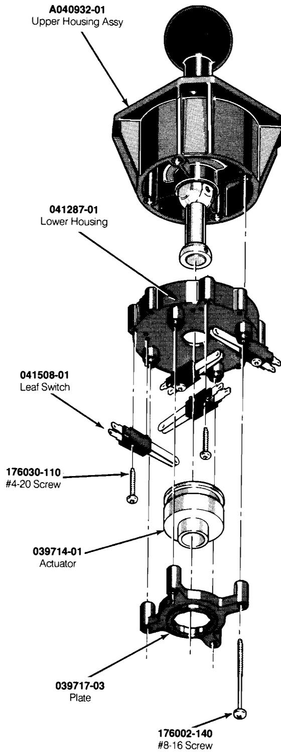
**Figure 5-3 Joystick Assembly
