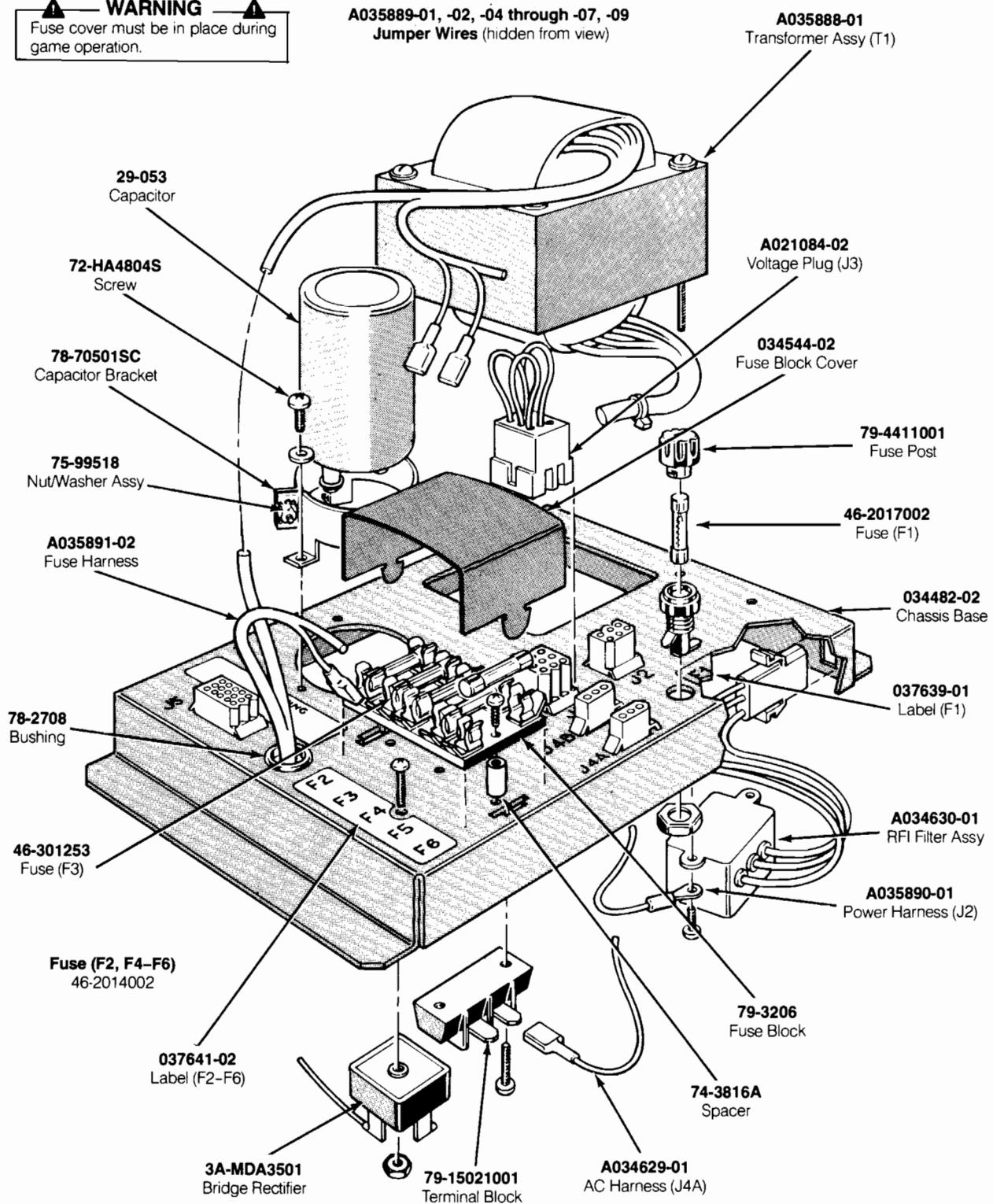
**Figure 5-5 Linear Power Supply Assembly**
