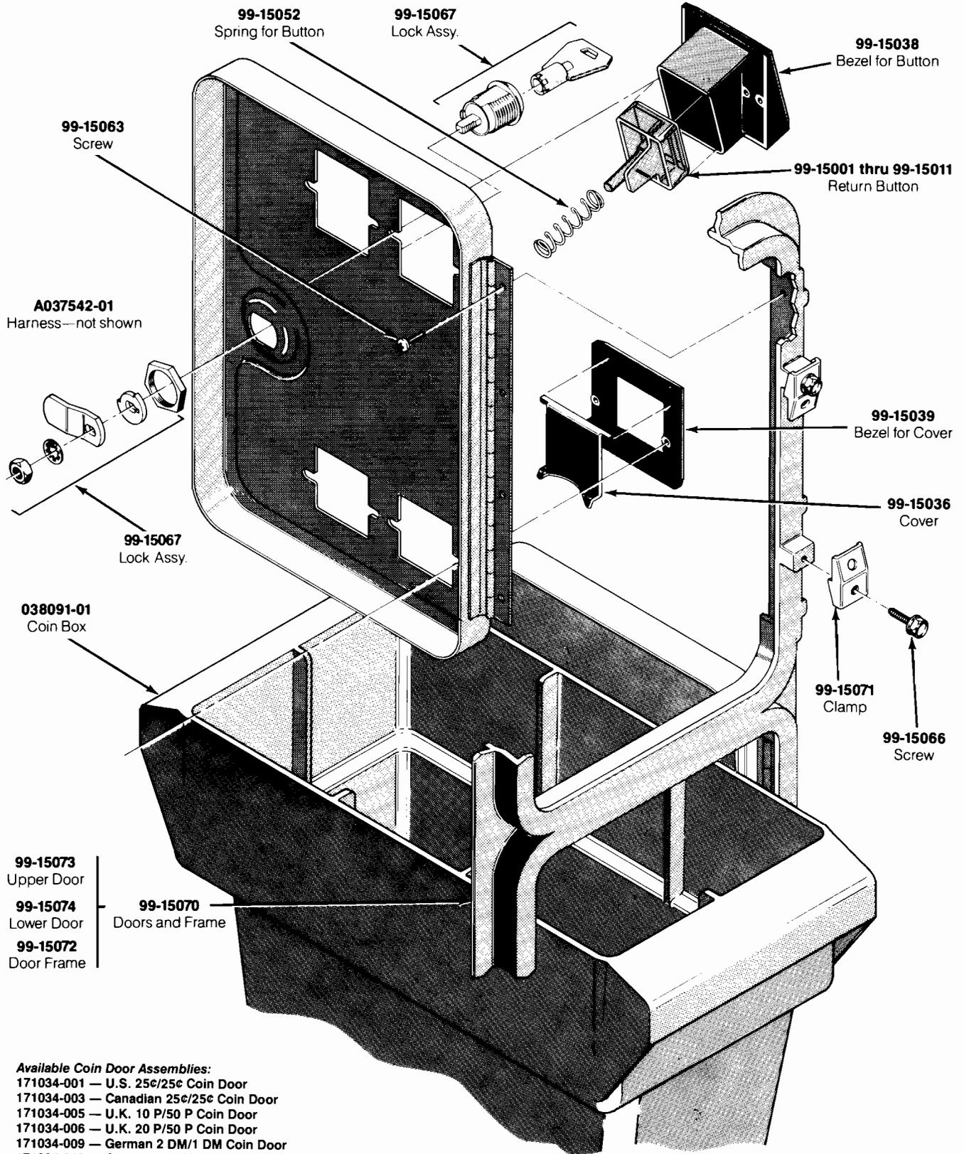
Figure 5-6 Coin Controls, Inc. Coin Door Assembly, continued
