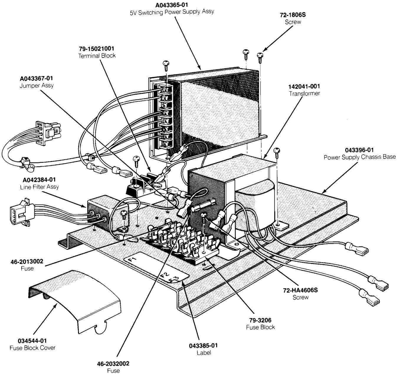
**Figure 5-4 Switching/Linear (SL) Power Supply Assembly
