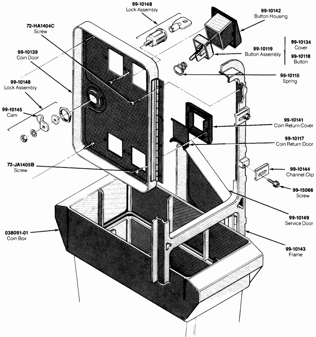
**Figure 5-7 Coin Acceptors, Inc. Coin Door Assembly, continued**
