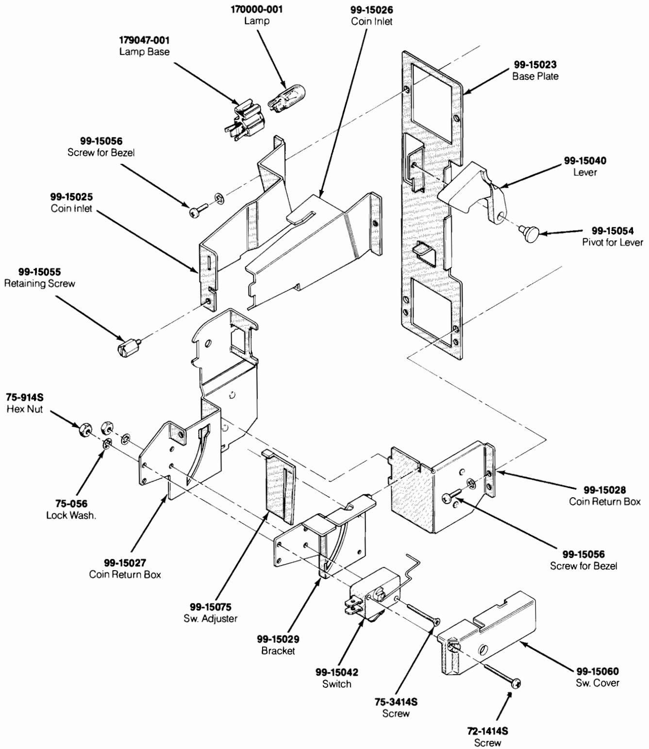
**Figure 5-6 Coin Controls, Inc. Coin Door Assembly
