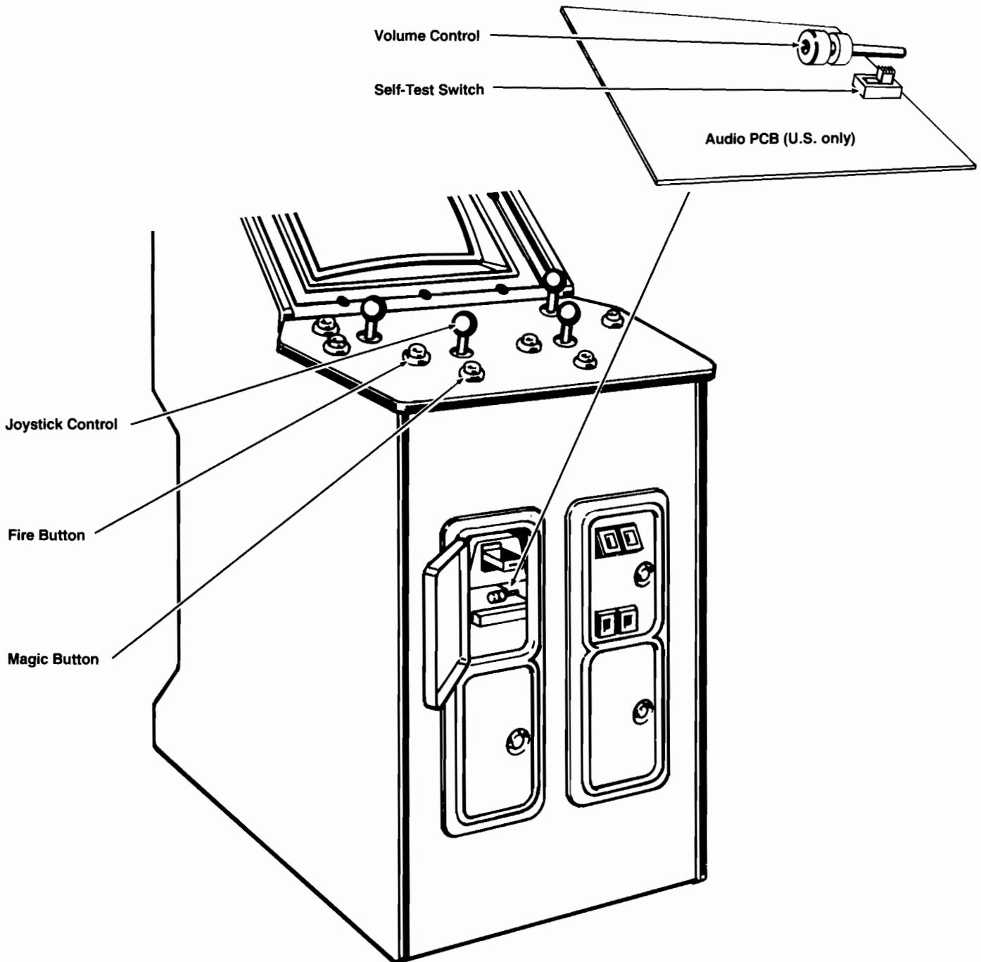
Figure 1-3 Control and Switch Locations
