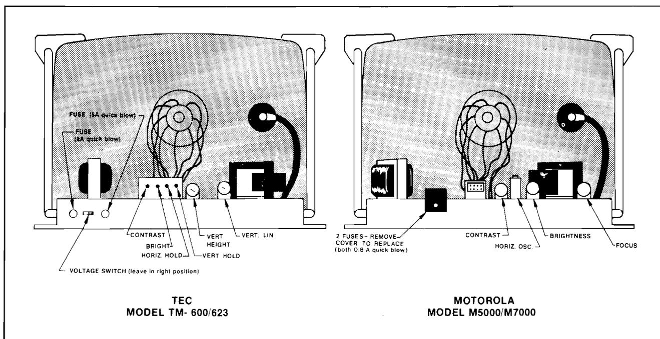
Figure 4-9 Locations of Adjustments on TV Chassis
