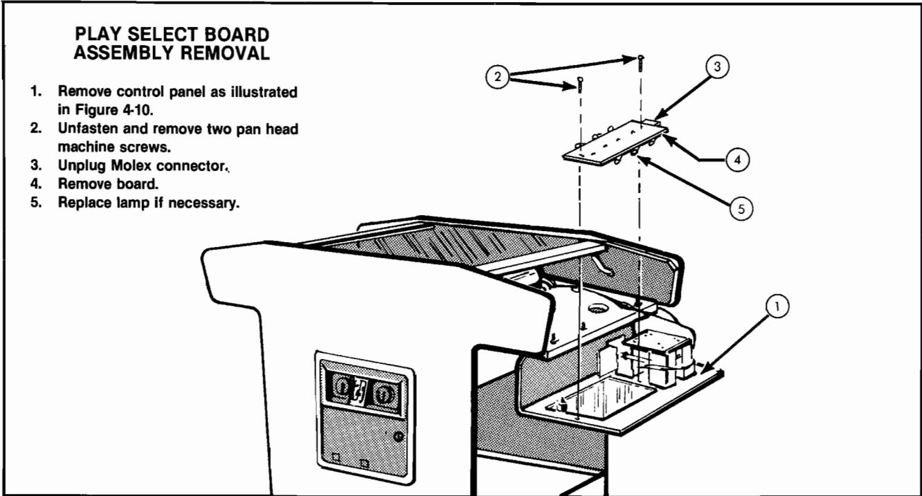
Figure 4-13 Play Select Board Assembly Removal
