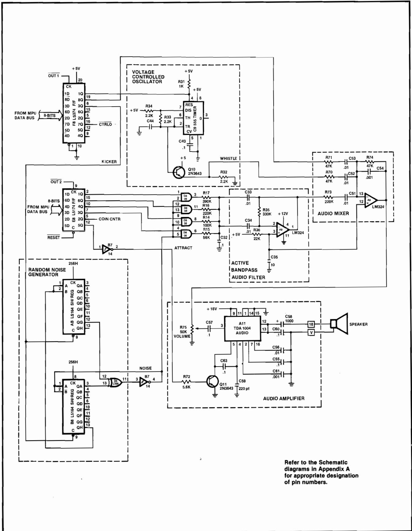
Figure 3-20 Audio Generator and Amplifier Simplified Schematic Diagram
