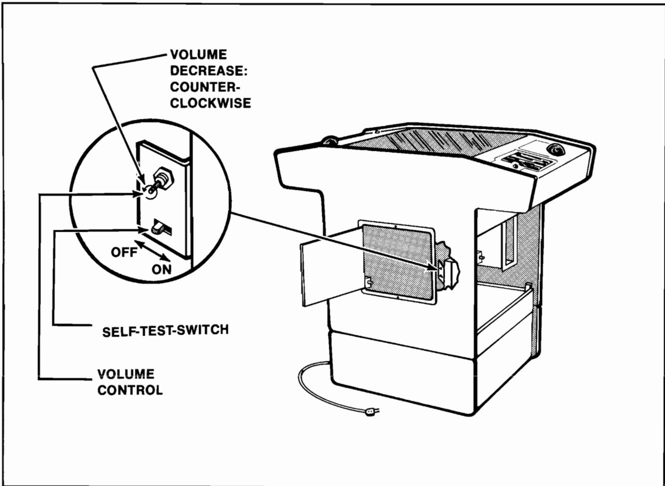
Figure 1-8 Location of Self-Test Switch and Volume Control
