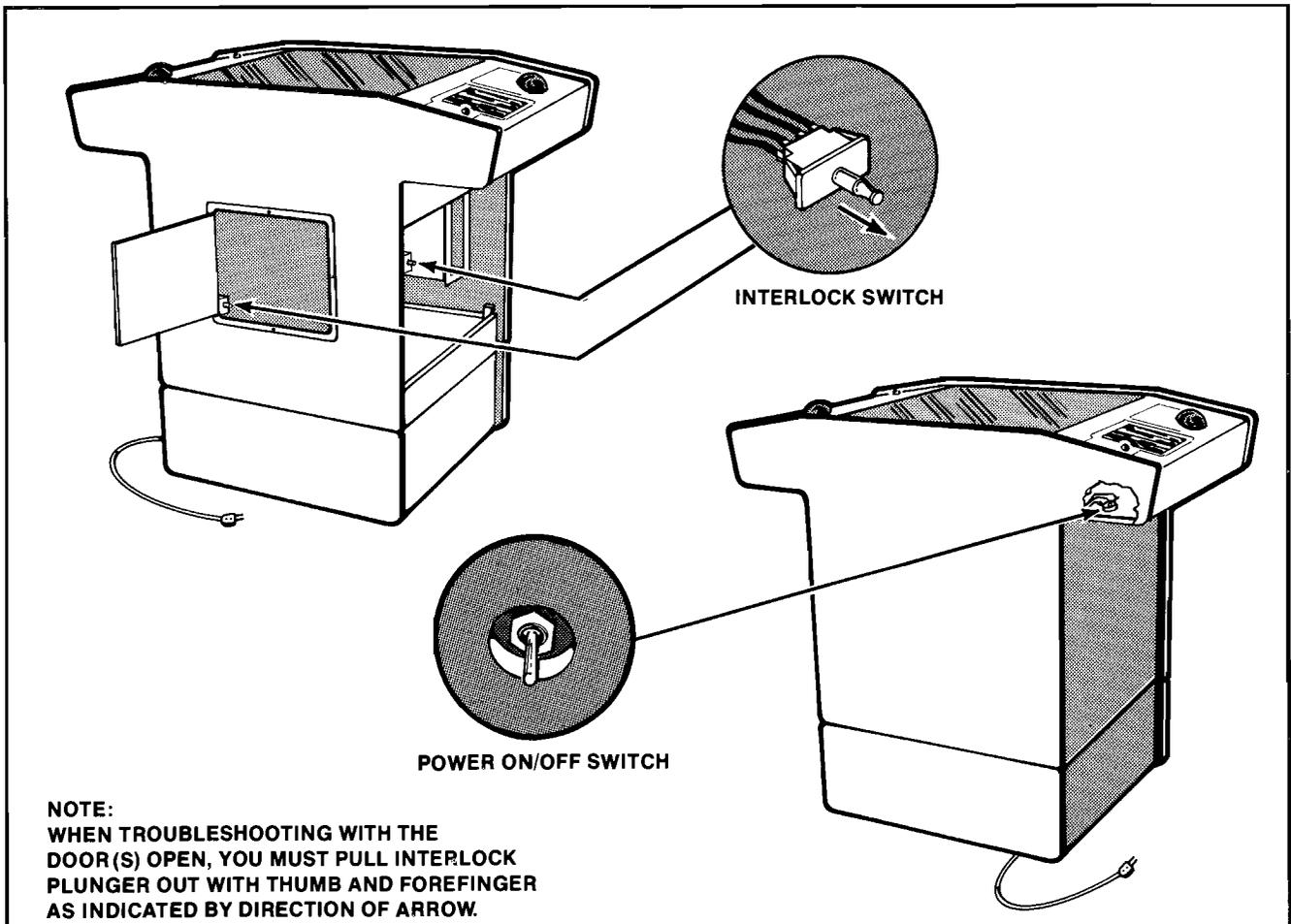
Figure 1-6 Location of Interlock and Power On/Off Switches
