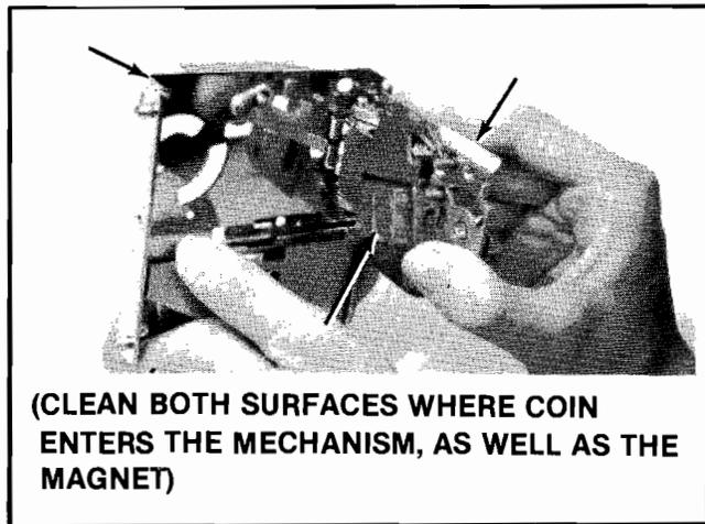
Figure 4-4 Surfaces to Clean Inside the Coin Mechanism
