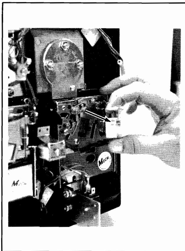
Figure 4-2 Hinging Open the Magnet Gate Assembly
