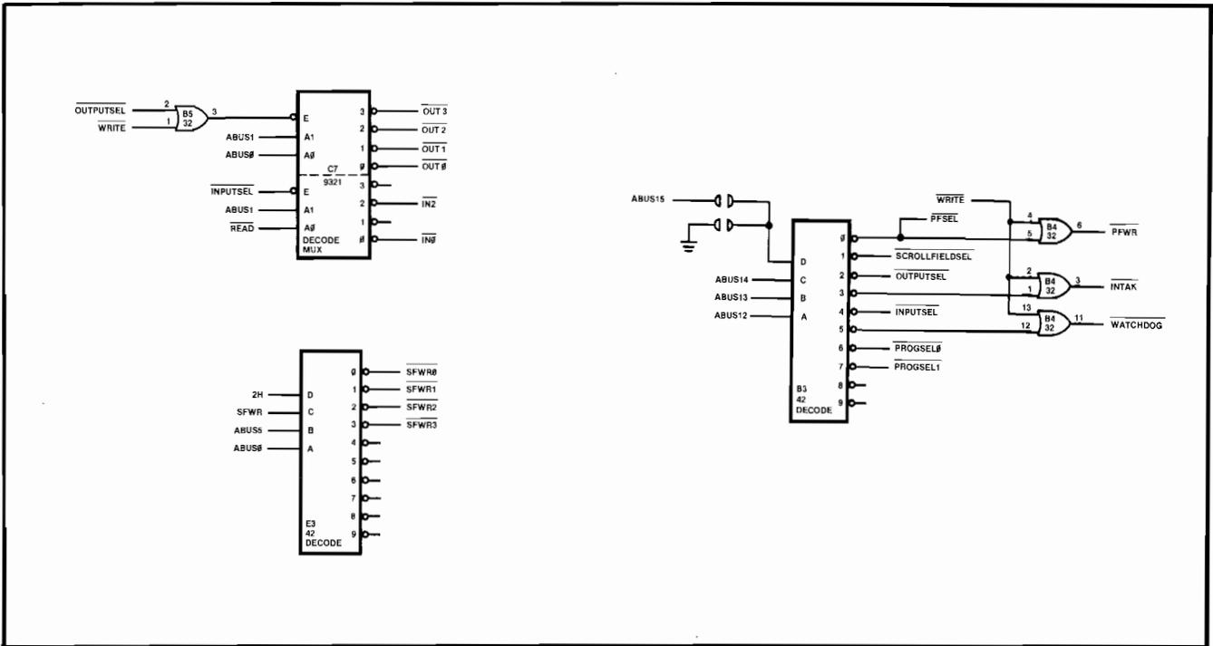
Figure 3-7 Address Decoding
