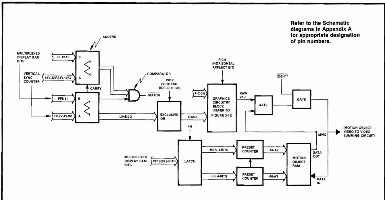
Figure 3-17 Motion Object Generator Block Diagram
