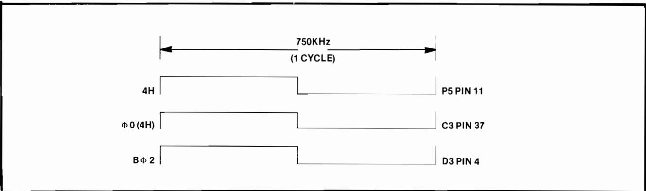
Figure 3-8 phi 0 Clock Driver Signal
