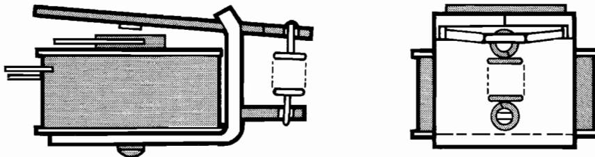
Figure 5-6 Coin Lockout Assembly
