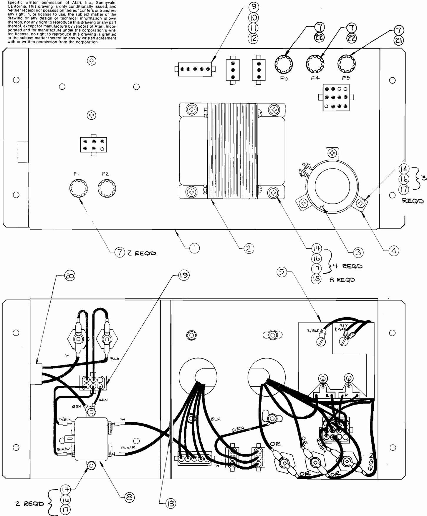
Figure 5-3 Type B Power Supply
