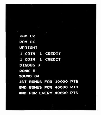
Figure 2-1 Self-Test Screen 1 Test Passes
