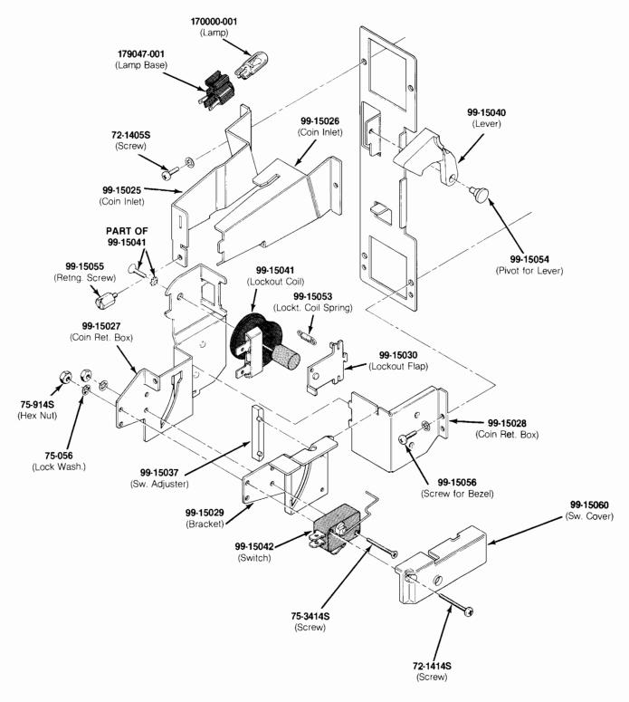
Figure 3-7 Vertical-Mounted Coin Door Upright and Cabaret Cabinets
