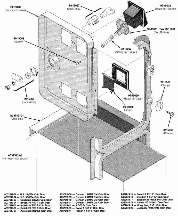
Figure 3-7 Vertical-Mounted Coin Door, continued Upright and Cabaret Cabinets
