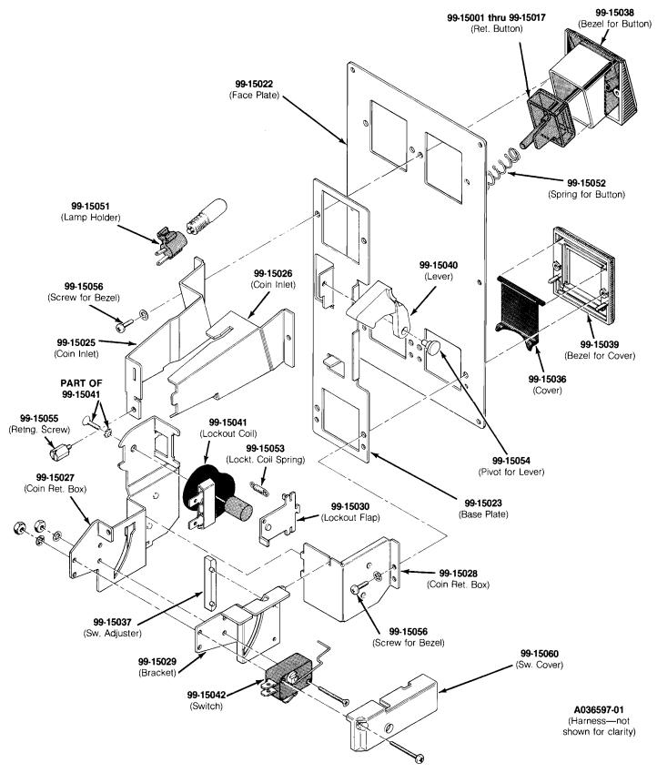
Figure 3-8 Double Coin Acceptor/Mount Assembly Cocktail Cabinet
