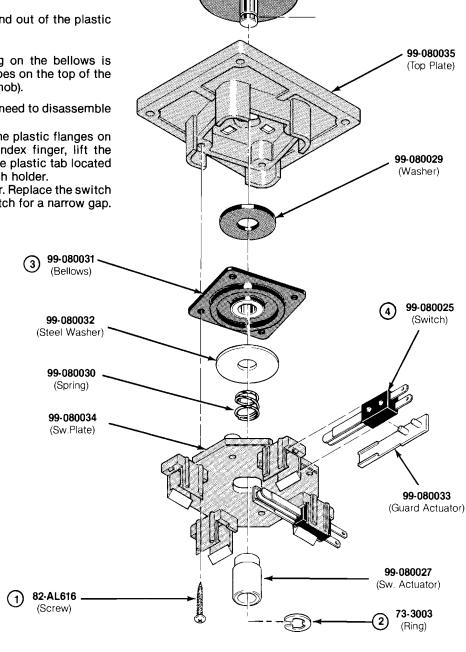
Figure 3-4 Joystick Assembly
