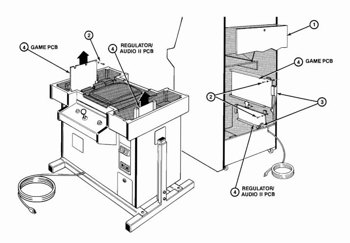
Figure 3-9 Printed-Circuit Board Removal
