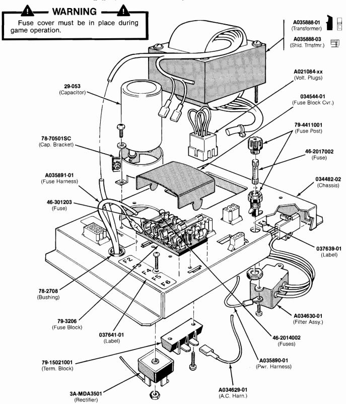
Figure 3-12 Power Supply Assembly
