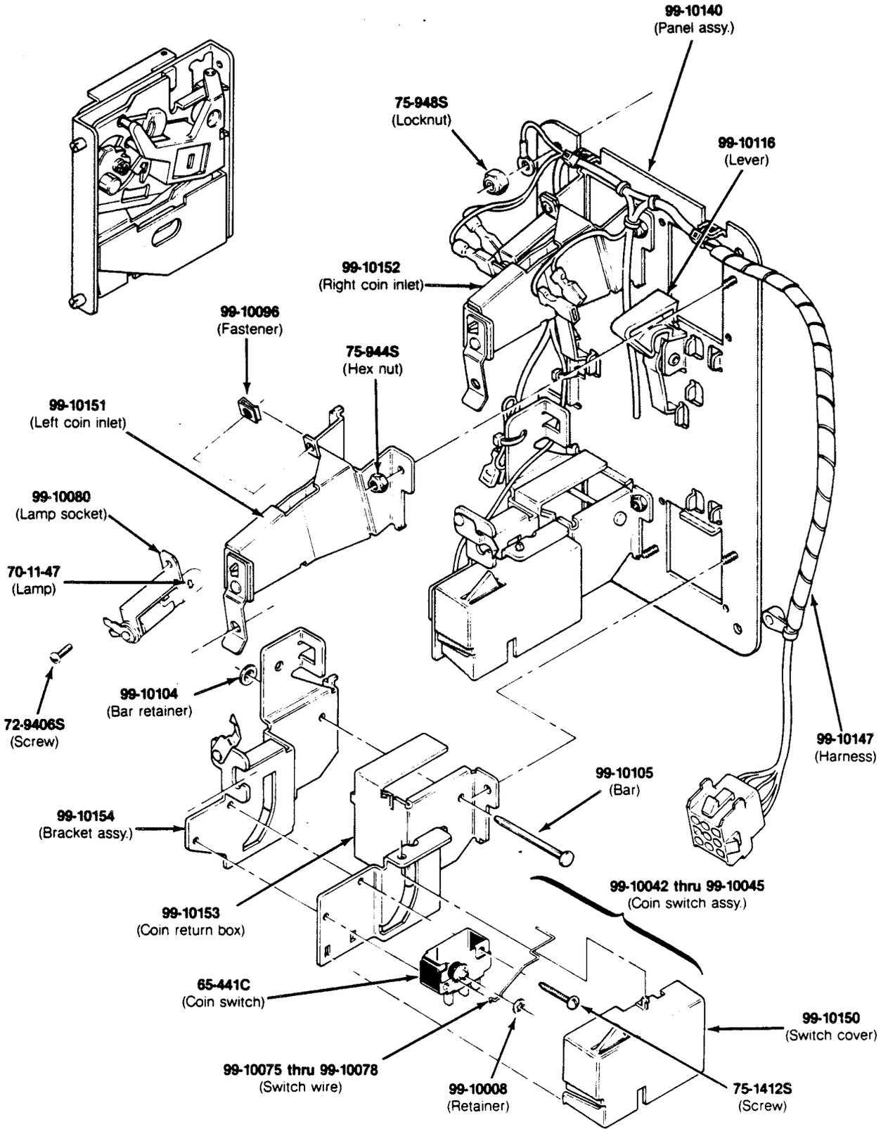
**Figure 3-9 American-Made Coin Door Assembly
