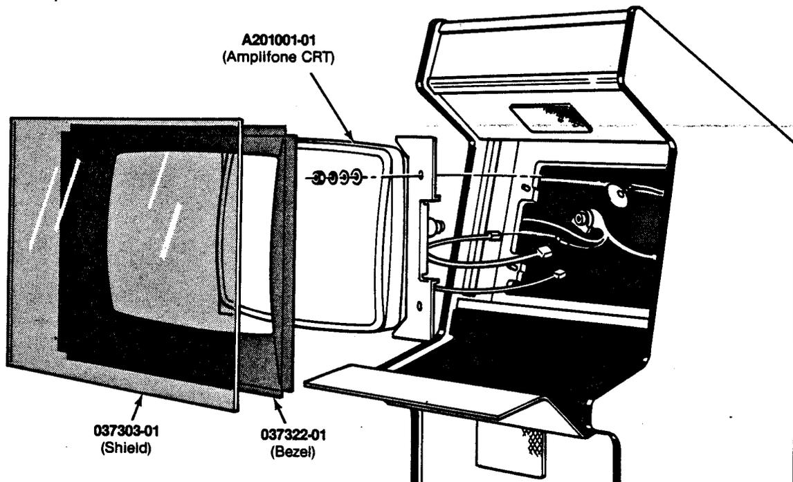
**Figure 3-6 Amplifone Video Display Parts List**
