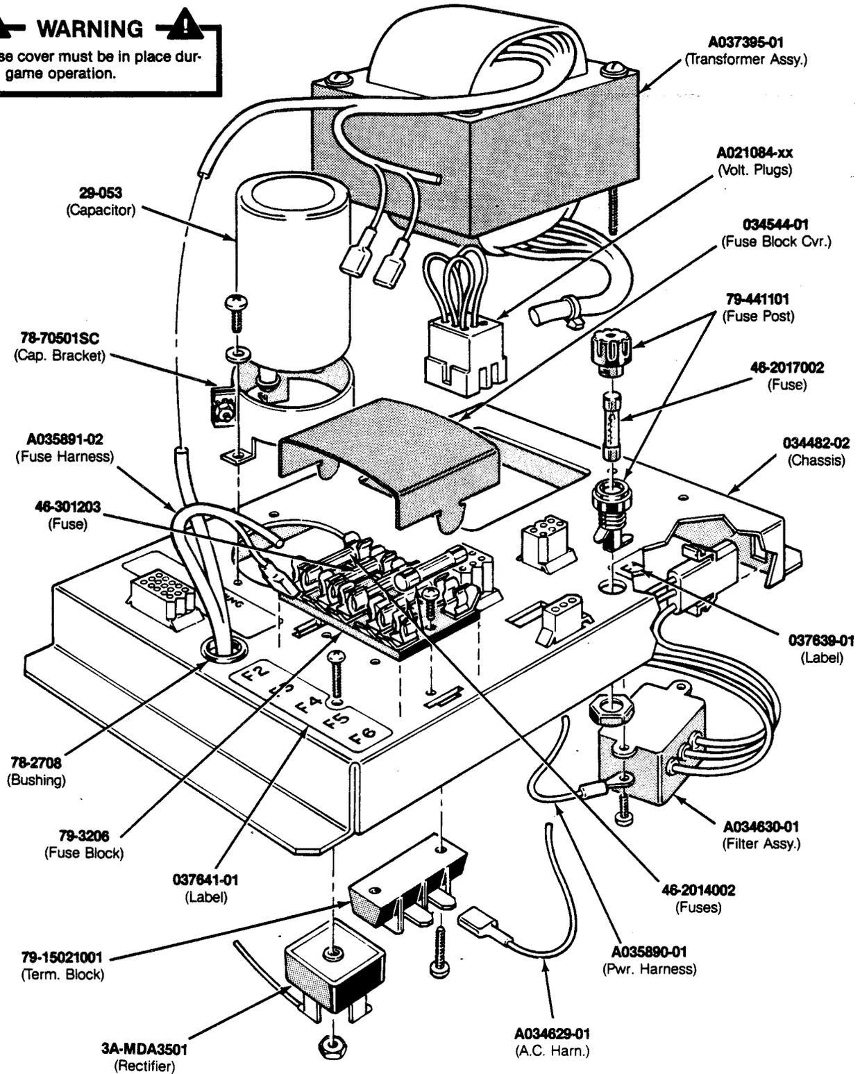
**Figure 3-10 Color X-Y Power Supply Assembly
