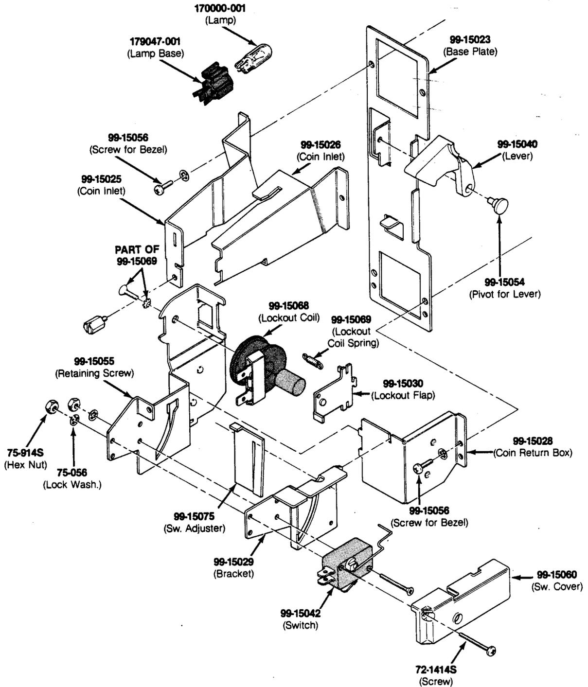
Figure 3-8 Vertically Mounted Coin Door
