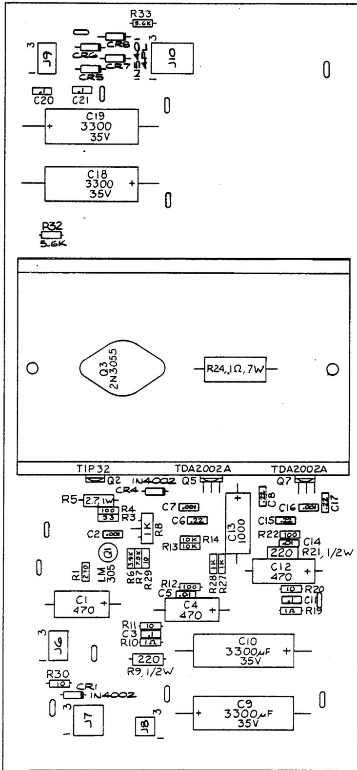
Figure 3-13 Regulator/Audio II PCB Assembly
