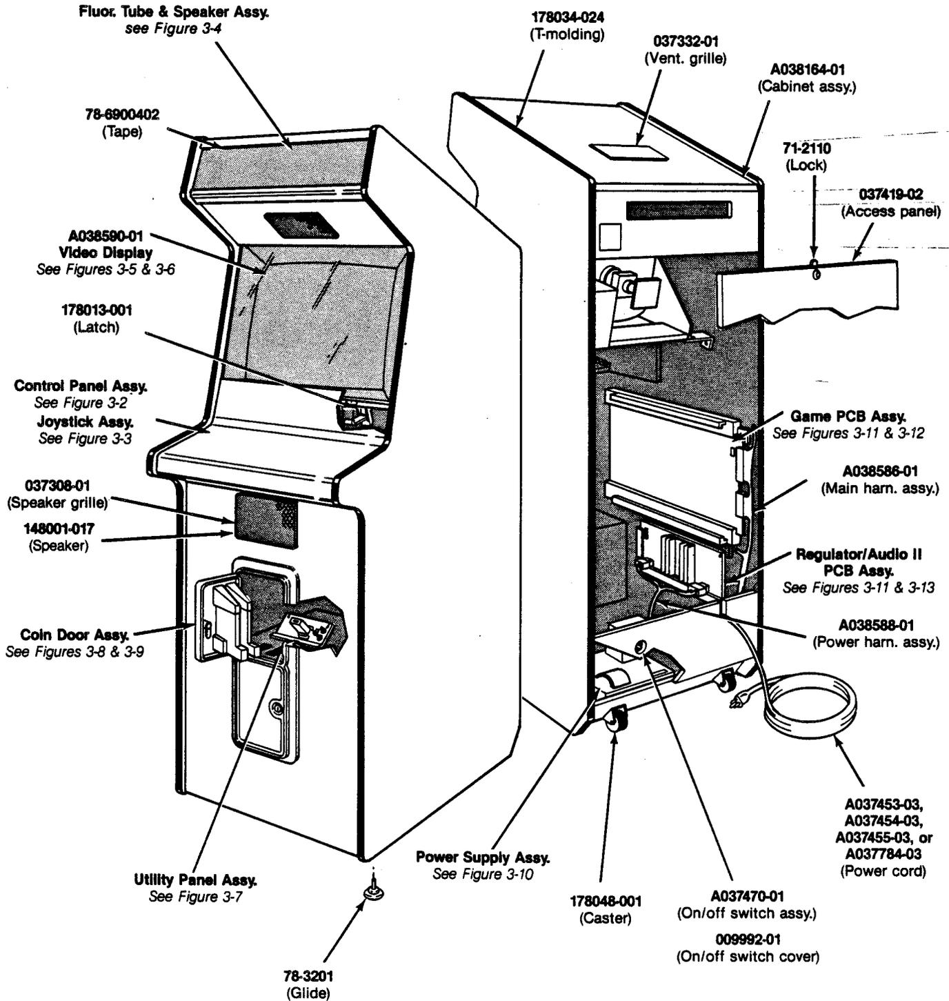
Figure 3-1 Cabinet-Mounted Assemblies
