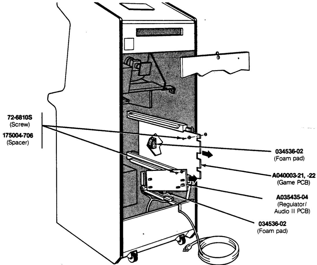
**Figure 3-11 PCB Mounting Hardware Parts List**
