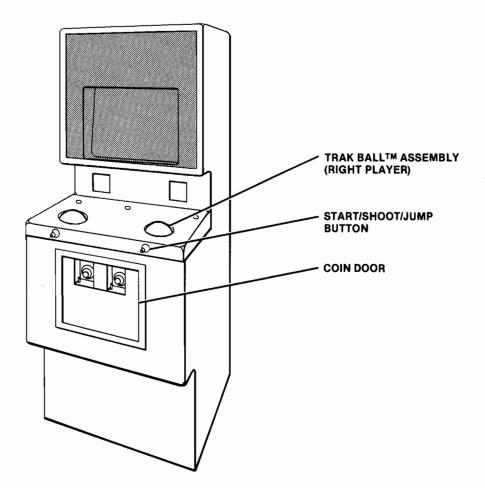
Figure 1-1 Control Panel and Player Controls
