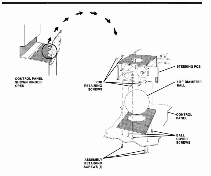
Figure 3-4 Trak-Ball<sup>™</sup> Assembly Removal
