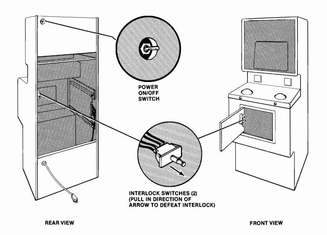
Figure 1-3 Power On/Off and Interlock Switches
