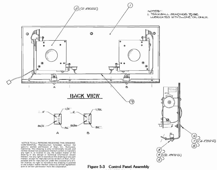
Figure 5-3 Control Panel Assembly A034355-01 A
