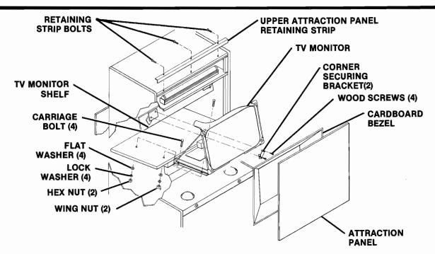
Figure 3-5 Removing the TV Monitor
