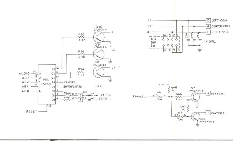
This circuit consists of coin counter drivers Q8, Q9, Q10 and data latch M10, clocked by the microcomputer's address decoder. When the input to a driver is clocked high, its collector goes low, grounding the return of the coin counter in the coin door. When START1 or START2 is clocked low, it grounds the START LEDs in the control panel.
