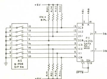
are selected by AB0 and AB1 from the MPU. Switch toggles ground.
