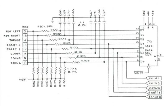
The coin door and some control panel switches are read by the MPU when SINP1 (switch input one enable) is low. Switches to be read are selected by AB0 thru AB2 from the MPU. All inputs are read on data line DB7. Switch inputs are "on" when pulled to ground.
