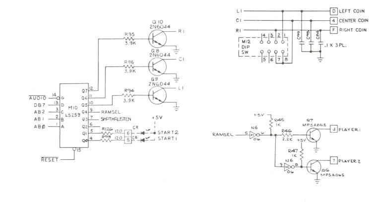
This circuit consists of coin counter drivers Q8, Q9, Q10 and data latch M10, clocked by the microcomputer's address decoder. When the input to a driver is clocked high, its collector goes low, grounding the return of the coin counter in the coin door. When START1 or START2 is clocked low, it grounds the START LEDs in the control panel.
