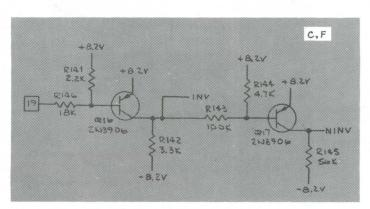
The video inverter circuitry is only used in a cocktail game. In an upright game, pin 19 is unconnected and therefore floats. When pin 19 floats, transistor Q16 is turned off and transistor Q17 is turned on. Therefore, INV is -8.2 VDC and NONINV is about +8.2 VDC. The result is a non-inverted X-axis and Y-axis output.
