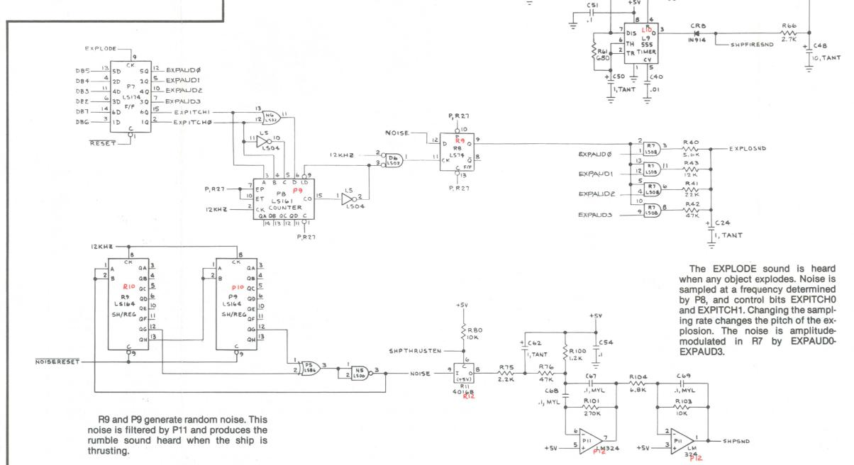
**AUDIO OUTPUT** All sounds are mixed in 1/4 of P11. This is Audio 1. The signal is then inverted by another THUMPSND RB3 47K 1/4 of P11 and becomes Audio 2. These out-ofphase signals provide a push-pull output to the SAUCRSND R77 W 39K audio section of the Regulator/Audio PCB. LIFESND R78 M47K SAUCREIRESND ROI WIOOK 5 AUDIO1 SHPFIRESND R84 W 100K EXPLOSND R82 4.7K SHPSND R102 4.7K 9-4 C113
