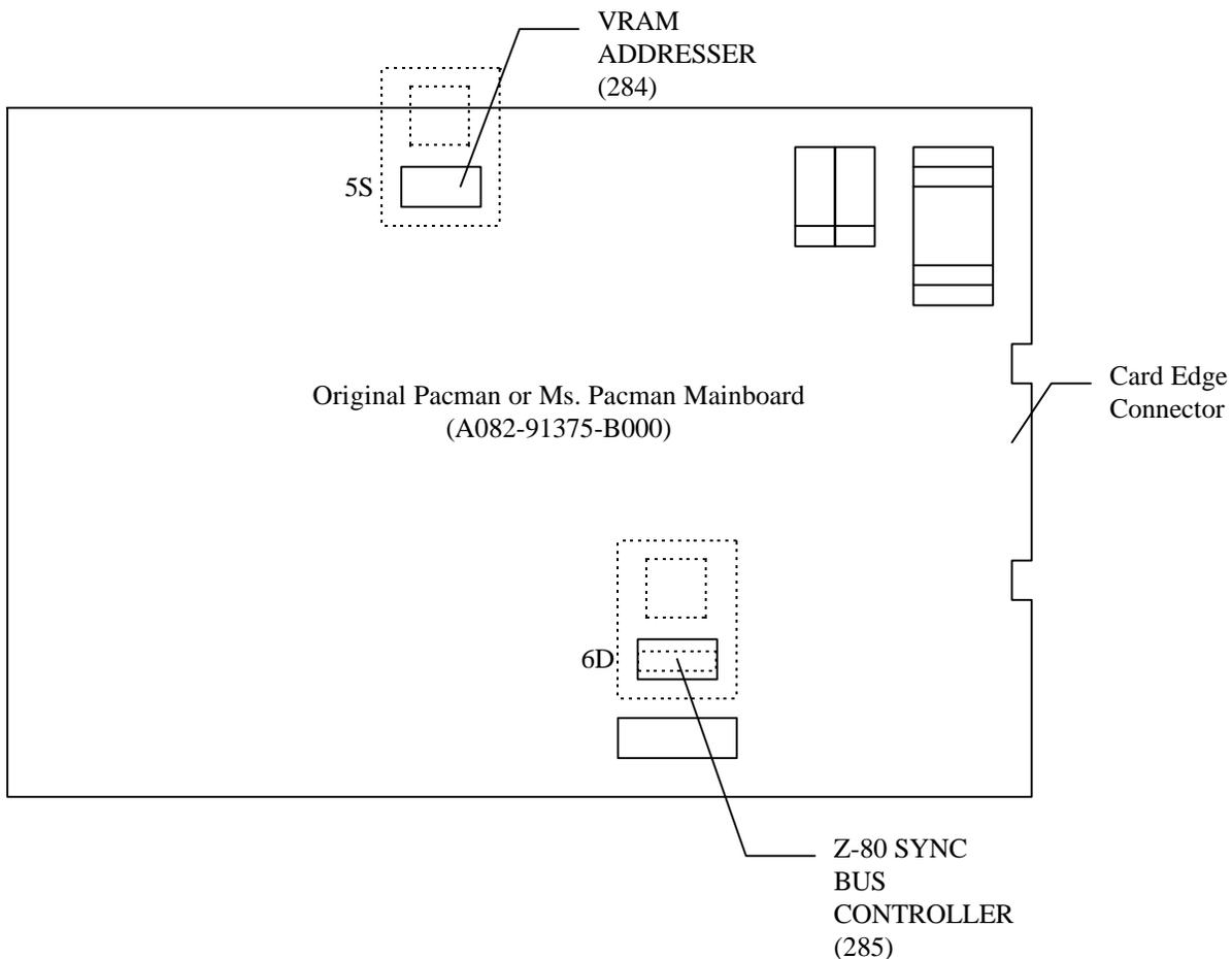
1. Remove the damaged or defective 284 or 285 daughtercard from location 5S (284) or 6D (285).
