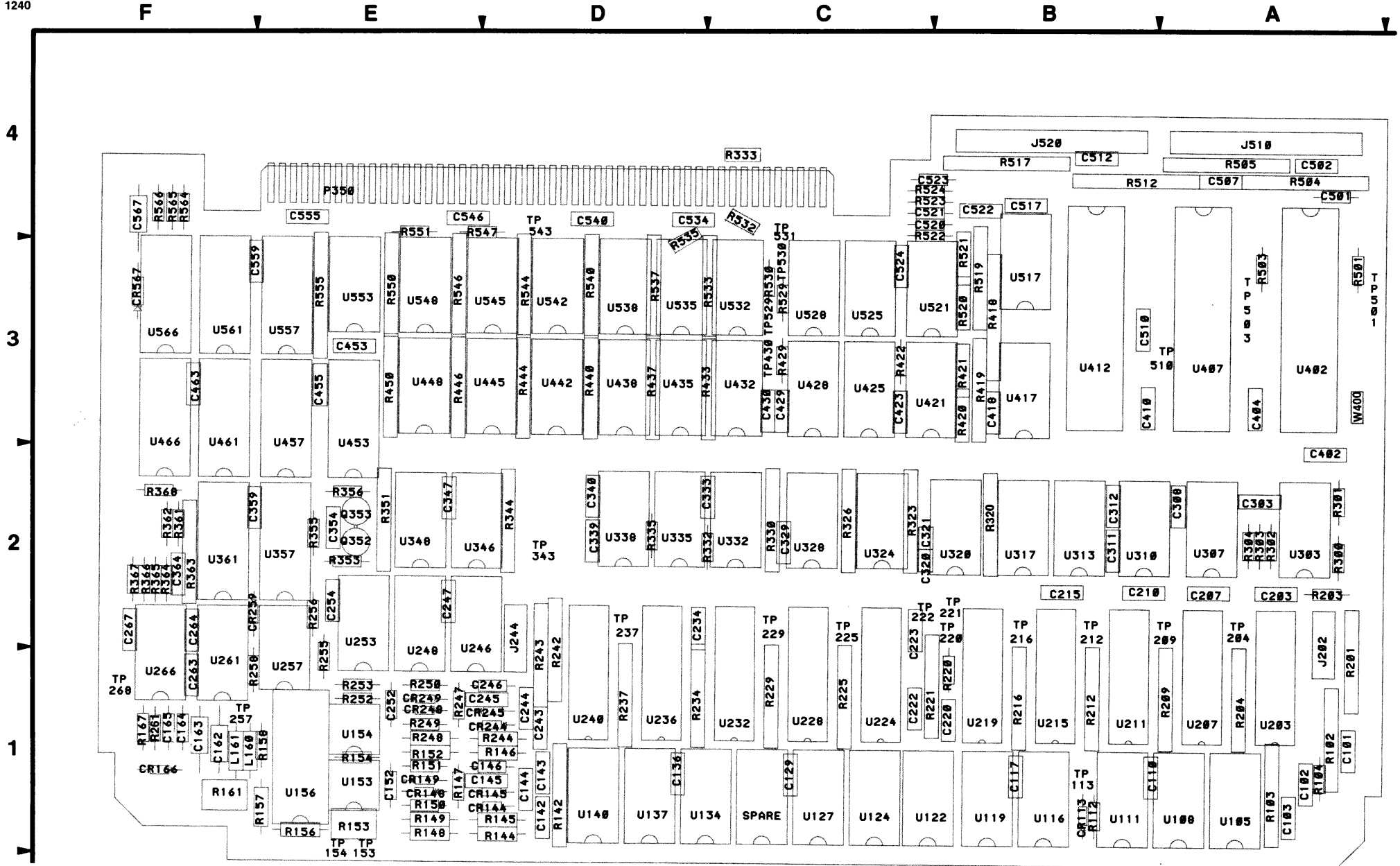
Figure 10-21. A16 18-Channel Acquisition Board Component Locations.
