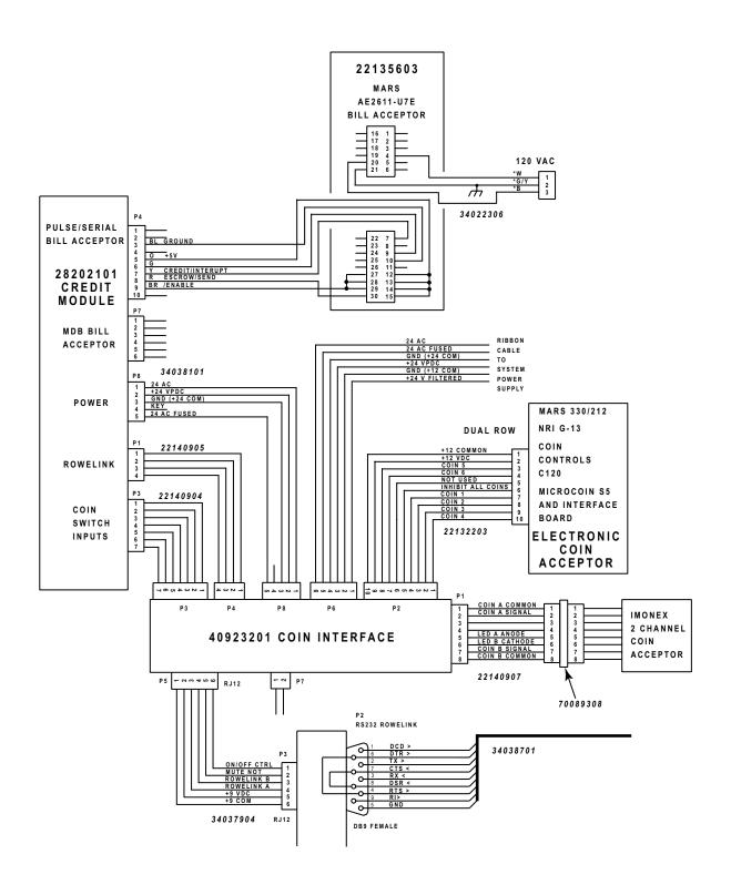
FIGURE 5-2 DL-11 WIRING DIAGRAM
