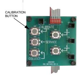
FIGURE 2-3 SWITCHES CIRCUIT BOARD
