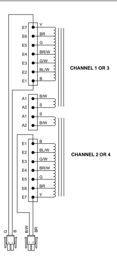
40832108 TRANSFORMER WIRING DIAGRAM
