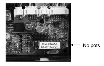
If you press the *Uplink to Mech* button a third time and your pcb does **not** have potentiometers, the CPM asks if you want to uplink the factory pot settings.
