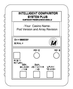
When the *Dual Voltmeter* Button is pressed the LCD will display the reference voltage levels that pot "C" and pot "S" on the control pcb are set to.
