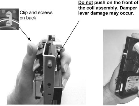
Using clip and screws on back for leverage, slide sensor coil assembly back to loosen token holder.
