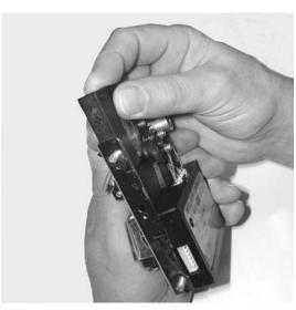
Slide sensor coil stack back and replace token holder
