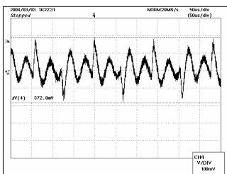
An oscillating current is passed through the exciter coil. The detector coils are magnetically coupled to the exciter coil via the magnetic fields in the gaps. The detector coils serve to sense the difference in magnetic field strength between the gaps. When this difference is at its smallest (balanced coil gaps), the resultant waveform is identified as a "null".
