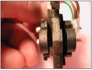
• Coin Comparitor ® technology uses a system of three coils spaced and stacked such that the diameters of each of the cylindrical coil bobbins are parallel to each other. There are two gaps created between the three coils. In one gap a reference sample coin is held. The other gap is positioned in the validation path below the coin entry. As the deposited coin passes through this gap, it is compared to the reference sample coin.
