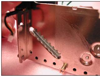
• The Accept Gate is located below the Sensor Coil Assembly and above the Exit Optics. If a valid coin is detected, the Accept Gate is opened allowing the coin to fall out the bottom of the unit on the accept side. In reject mode, a bad coin is deflected by the Accept Gate and falls out of the bottom of the mechanism on the reject side.
