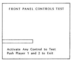
When any control panel button is pushed, it lights up on the panel its name appears in the blank area of the screen. To test coin mechs, insert a coin or token in each one, and Coin Mech 1 (left mech), Coin Mech 2 (right mech) message appears on the screen for each. The Manual Mode button may also be tested. The long green horizontal line at the bottom expands and shrinks lengthwise when the knob is turned. To return to the menu, press Player 1 and Player 2 at the same time.
