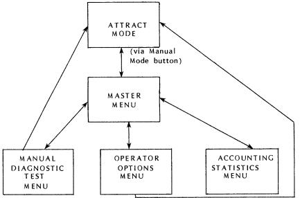
The only way to leave the Operator Interface Mode and return to the Attract Mode is to select "Exit Operator Interface, Resume Play", a selection on any menu. Also, the Manual Diagnostic Menu, Operator Options Menu, and Accounting Statistics Menu have a selection allowing you to return to the Master Menu.
