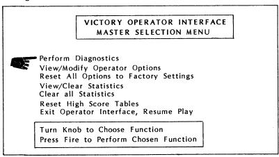
In the left margin, a hand pointer is left of the first function, "Perform Diagnostics". The operator uses the Control Panel Knob to move the hand pointer to the appropriate menu selection, and presses the Fire button to have the function carried out.
