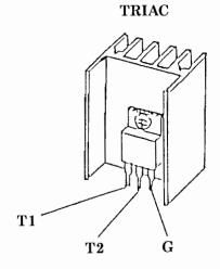
Turn the power off and check for the presence of conductivity between T1 and T2 out of the 3 Triac pins by using a tester. If conductivity is present, then the Triac is damaged.
